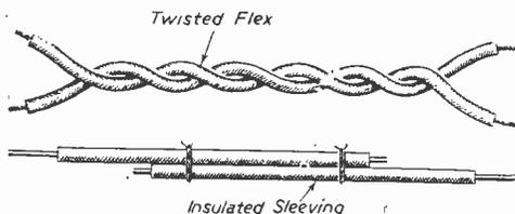
Fig. 1.—Temporary small value condensers may be made up on these lines.
