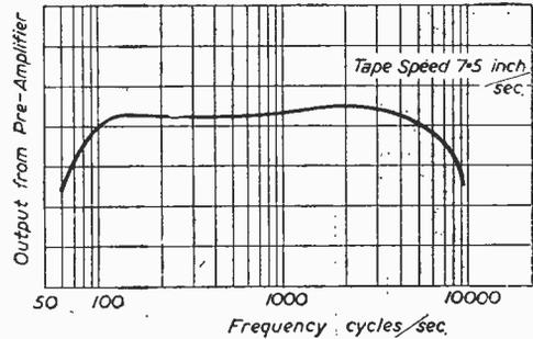
Fig. 3.—Equalised curve for constant input voltage.
