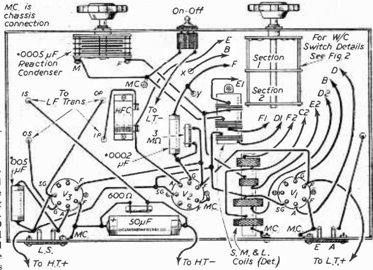
Fig. 6.—Sub-chassis layout and wiring.
