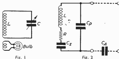
Fig. 1.—Simple absorption wavemeter. The loosely coupled bulb circuit does not damp the tuned circuit as much as when the bulb is directly included in the tuned circuit. The values of  $L$  and  $C$  are chosen so as to allow of resonance at the frequency of interest.
