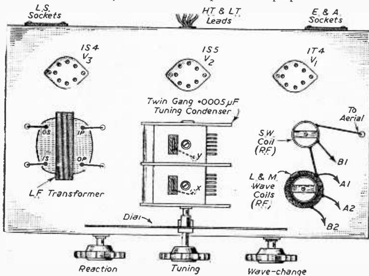
Fig. 2.—Top of chassis layout.
