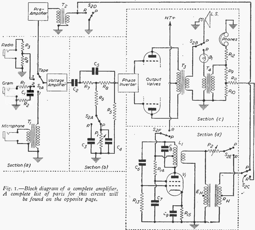
Fig. 1.—Block diagram of a complete amplifier. A complete list of parts for this circuit will be found on the opposite page.
