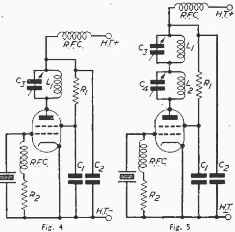
A crystal replaces the T.G. circuit here, and in Fig. 5 an additional tuned circuit ( $L_2C_4$ ), resonated to its second harmonic enables the oscillator of Fig. 4 to give a useful second harmonic output, although the Tritet has now superseded this arrangement.
