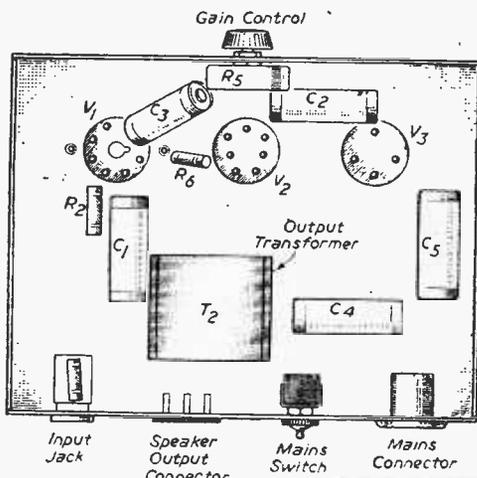
Fig. 3.—Key to the positions of the components shown in the photograph of the sub-chassis view of the amplifier.
