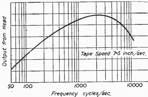
Fig. 2.—Uncompensated output to be expected from the playback head.
