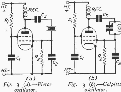
The circuit of Fig. 3(a), commonly called the Pierce oscillator, although Pierce originated the circuit of Fig. 4 as well, may be regarded as derived from the modified Colpitts oscillator of Fig 3 (b).
