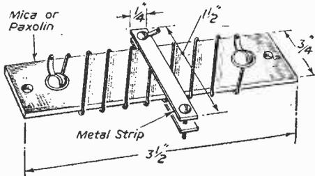
Fig. 2.—Details of the main L.T. dropping resistor.
