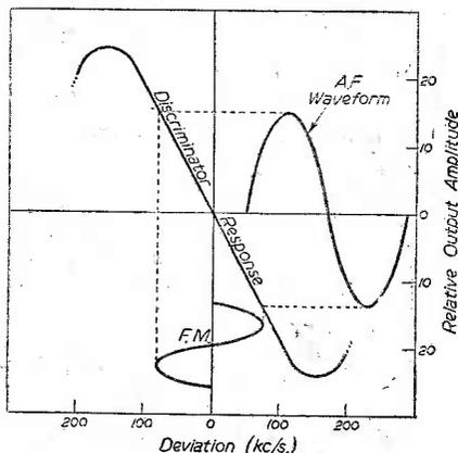
Fig. 9.—Response characteristic of amplitude discrimination.
