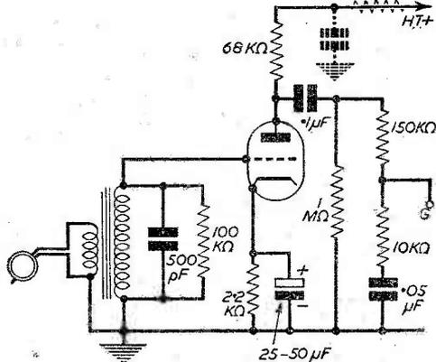
Fig. 6.—To provide bass compensation a tone-control pre-amplifier is desirable using a circuit similar to that shown here.
