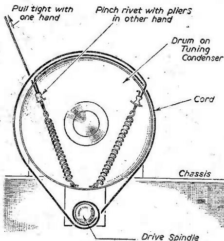
Fig. 1.—The simplest type of cord drive showing method of terminating cord.
