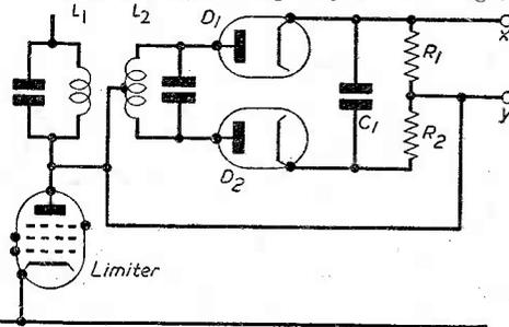
Fig. 10.—Basic circuit of phase discriminator.
