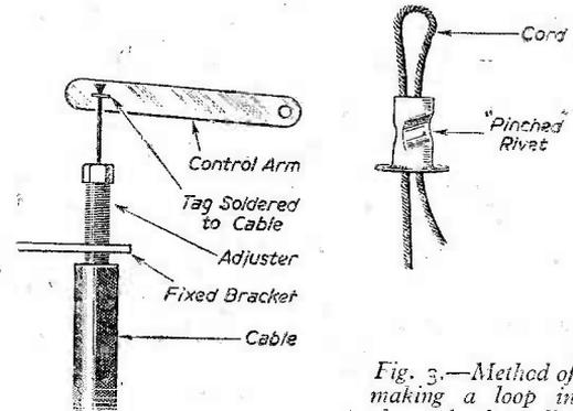
Fig. 2.—Construction of a Bowden cord adjustment.
