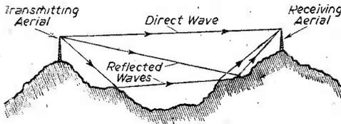
Fig. 4.—This diagram shows how a signal can be split up in radiation.
