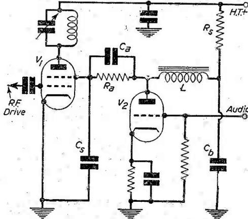
Fig. 2.—Choke-coupled screen modulator.
