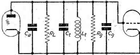
Fig. 5a.—Single parallel circuit.
