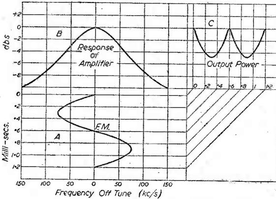
Fig. 5.—Composite graph, illustrating the introduction of A.M. on an F.M. signal when passed through a tuned stage having a response as shown in A. Note that the output power waveform in C is really the shape of the resultant amplitude modulation envelope.
