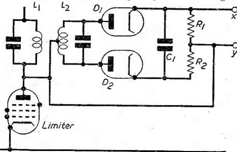
Fig. 10.—Basic circuit of phase discriminator.
