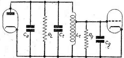
Fig. 6.—A tapped parallel circuit. The step-down voltage ratio =  $r$ .
