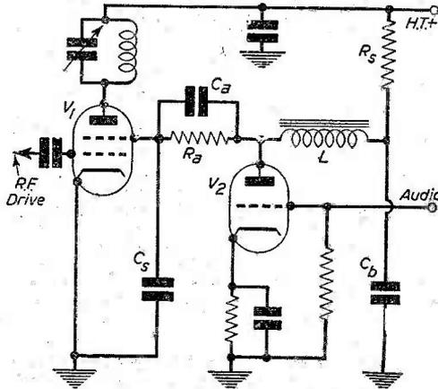
Fig. 2.—Choke-coupled screen modulator.
