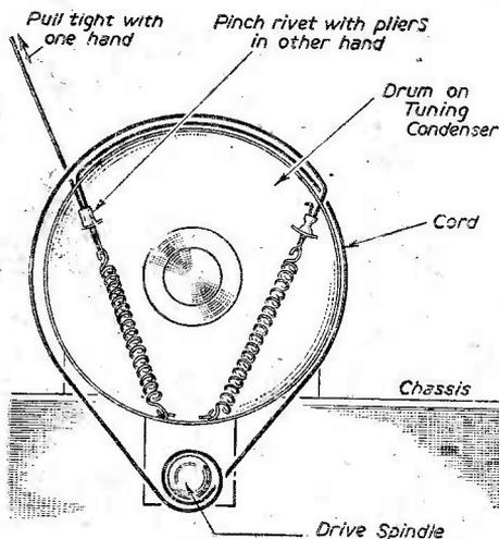
Fig. 1.—The simplest type of cord drive showing method of terminating cord.
