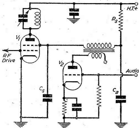
Fig. 1.—Transformer-coupled screen modulator.
