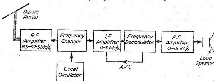
Fig. 11.—Block schematic of an F.M. receiver.
