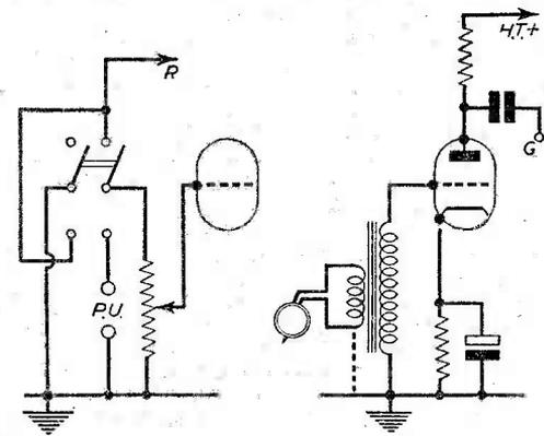
Fig. 4 (left).—A double-pole change-over switch arranged as shown here will enable radio to be silenced when using gramophone. Fig. 5 (right).—A simple pre-amplifier stage which is necessary with low-output pick-ups.
