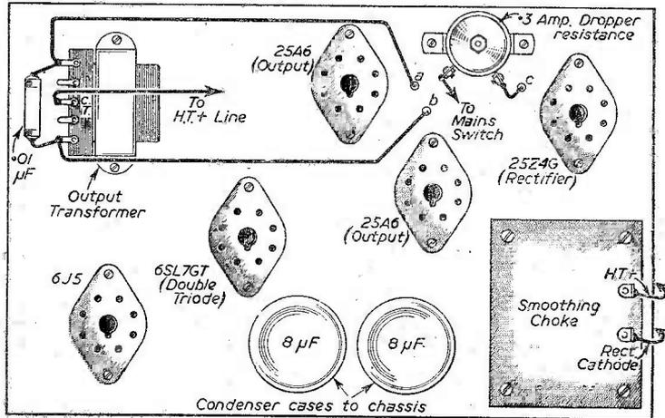
Fig. 2.—Top of chassis layout.
