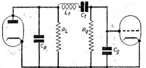
Fig. 7.—A series circuit.
