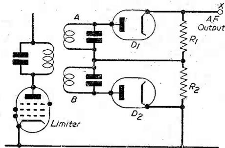
Fig. 8.—Basic circuit of amplitude discriminator.
