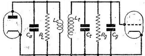
Fig. 5b.—An untuned primary is shown here.
