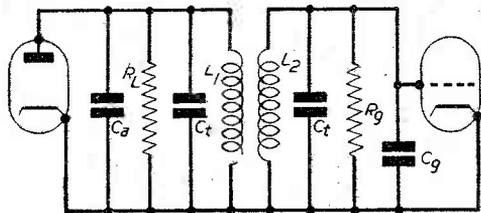
Fig. 8.—A double parallel circuit.
