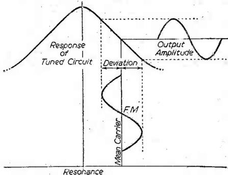
Fig. 7.—Using a mistuned resonant circuit to convert F.M. to A.M.
