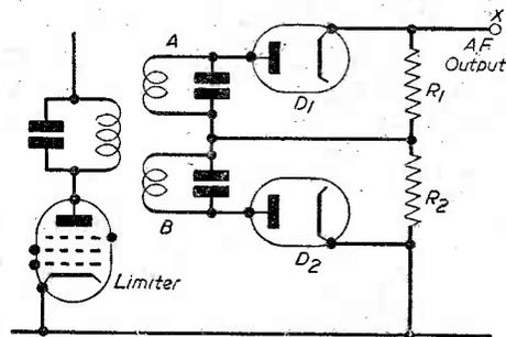
Fig. 8.—Basic circuit of amplitude discriminator.
