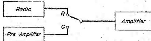
Fig. 7.—A radiogram consists merely of a radio tuner, a pre-amplifier and a main amplifier, with input switching as shown in this block diagram.
