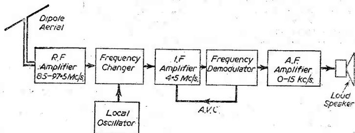
Fig. 11.—Block schematic of an F.M. receiver.
