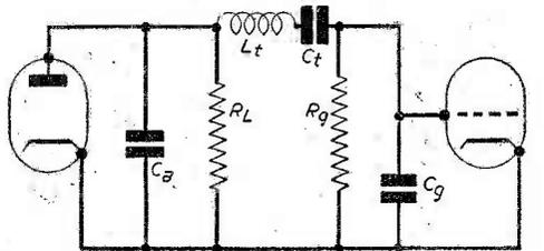
Fig. 7.—A series circuit.
