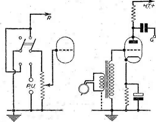
Fig. 4 (left).—A double-pole change-over switch arranged as shown here will enable radio to be silenced when using gramophone. Fig. 5 (right).—A simple pre-amplifier stage which is necessary with low-output pick-ups.
