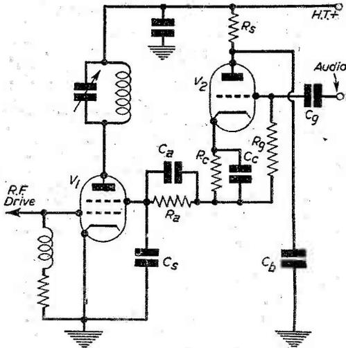
Fig. 4.—Series-screen modulator.
