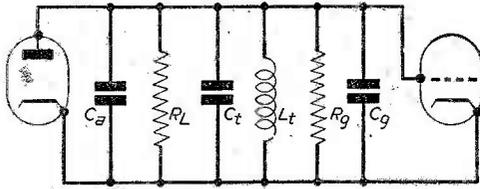
Fig. 5a.—Single parallel circuit.
