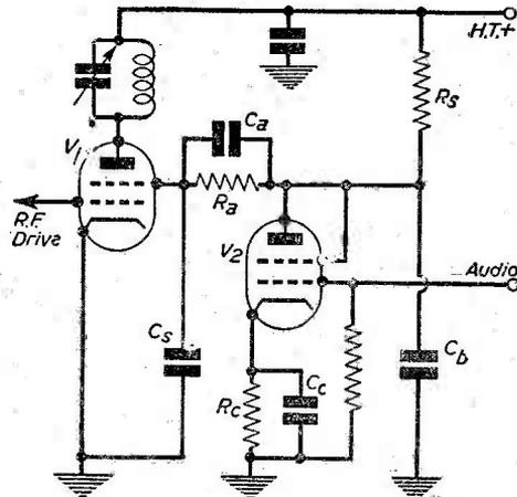
Fig. 3.—Resistance-coupled screen modulation.
