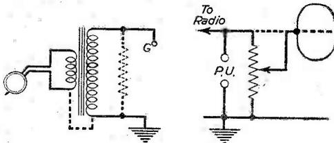
Fig. 3.—A resistor is sometimes necessary across the pick-up transformer secondary, and it is generally desirable to earth the primary winding. Fig. 3 (a) (right).—Pick-up sockets may be connected direct across a radio volume control if this is on the L.F. side.
