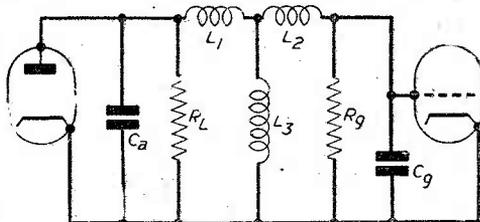
Fig. 9.—A common inductance shunt.
