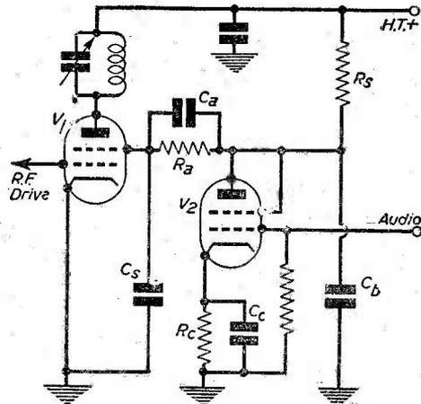
Fig. 3.—Resistance-coupled screen modulation.
