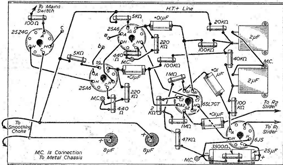
Fig. 3.—Under-chassis wiring details.
