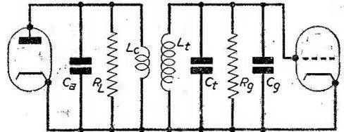
Fig. 5b.—An untuned primary is shown here.
