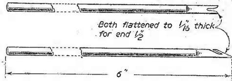
Fig. 4.—Threading tool for dial cord.
