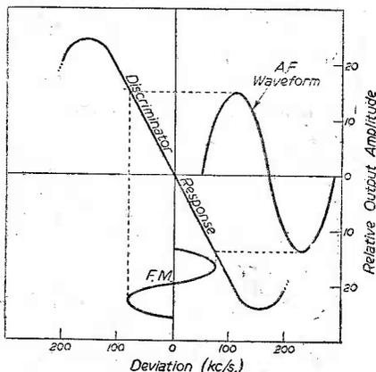
Fig. 9.—Response characteristic of amplitude discrimination.
