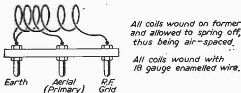
Fig. 3.—Method of winding L<sub>1</sub> and coil-winding data.
