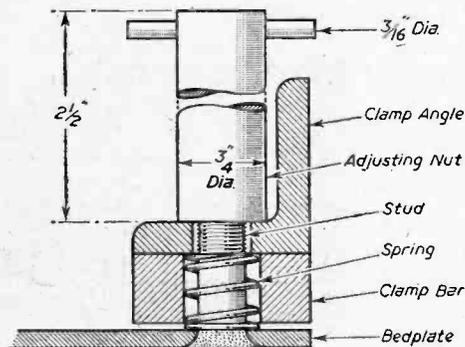
Fig. 2.—The spring-loaded clamp.
