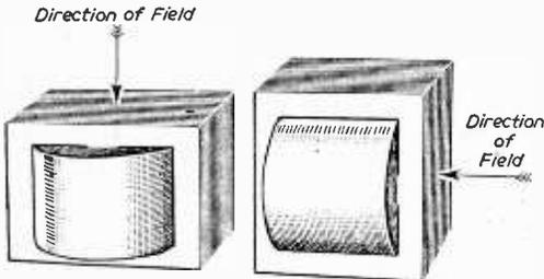
Fig. 4.—Mounting positions of transformers or chokes to avoid interaction.
