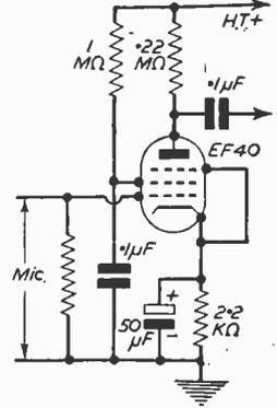
Fig. 5.—Circuit of a single stage pre-amplifier.
