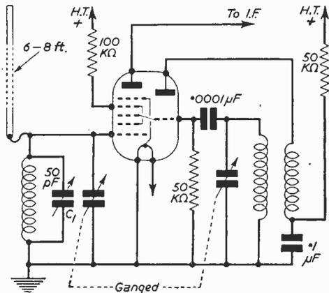
Fig. 4—Tuned aerial circuit in a frequency changer stage of a superhet or S.W. converter.
