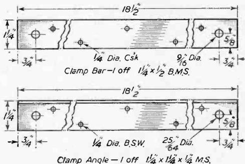
Fig. 3.—Clamp bar and angle.
