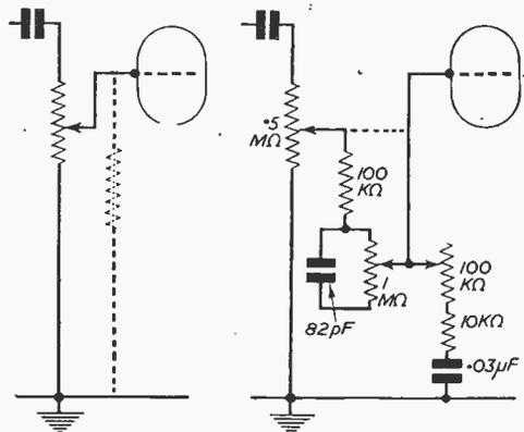
Fig. 1 (left).—Standard volume control. Fig. 2 (right).—Additional components for a compensated volume control.
