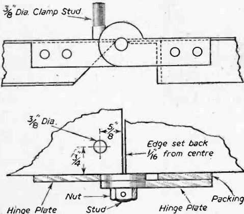
Fig. 4.—Details of the hinge.
