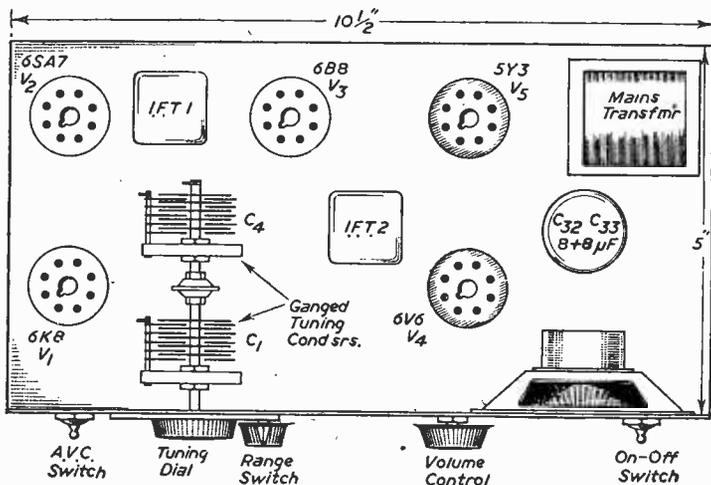
Fig. 2.—Layout and dimensions of the chassis.
