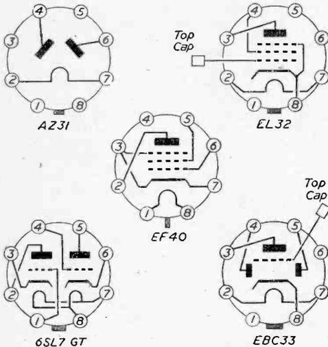
Fig. 1.—Valve-base connections.
