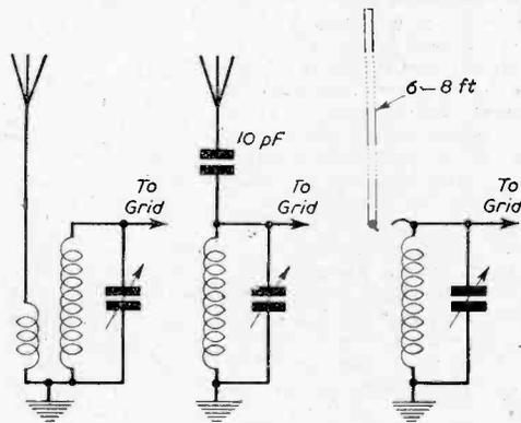
Fig. 1—An untuned aerial. Fig. 2—Another form of untuned aerial. Fig. 3—A tuned aerial.
