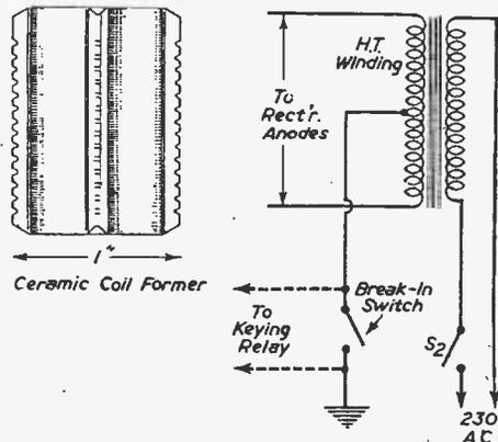
Figs. 3 and 4.—(Left) The coil former. (Right) Details of switch in the H.T. winding.
