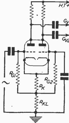
Fig. 6.—The phase inverter stage.
