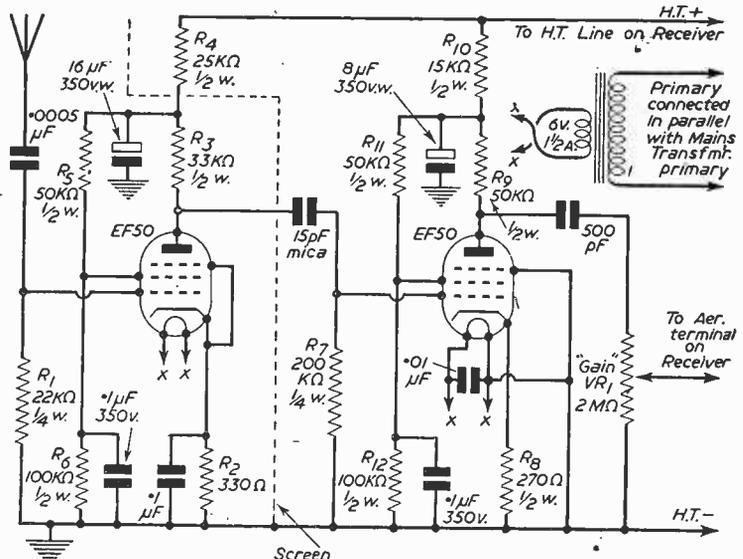
The circuit of the pre-amplifier. No separate list of parts is given as all details are marked on the circuit.
