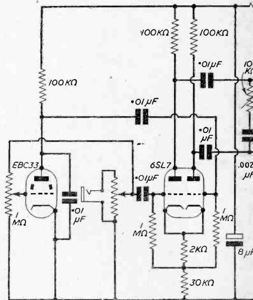
Fig. 2.—Theoretical circuit of the amplifier. T
