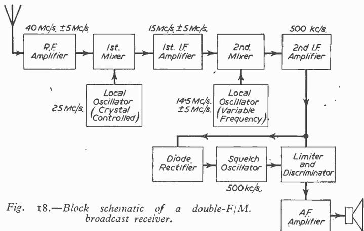
Fig. 18.—Block schematic of a double-F/M broadcast receiver.
