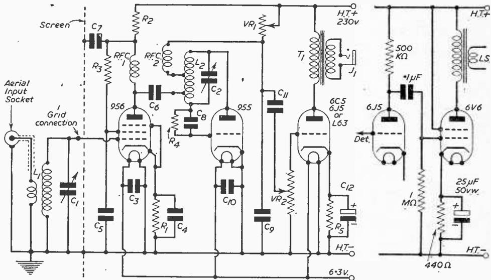
Fig. 1.—Theoretical circuit and alteration L.S. output.
