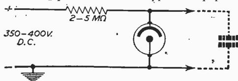
Fig. 2.—A D.C. supply for experimental use.
