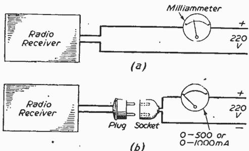
Fig. 1—(above) Basic arrangement and (below) practical arrangement.
