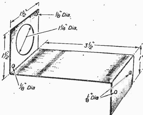
Fig. 1.—Details of the bracket for the unit.
