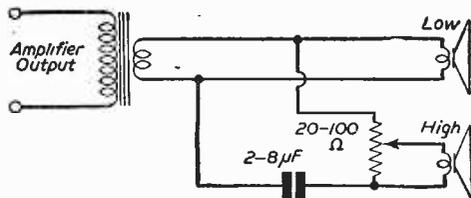
Fig. 2.—A simple cross-over scheme to avoid overloading the small "top" speaker.
