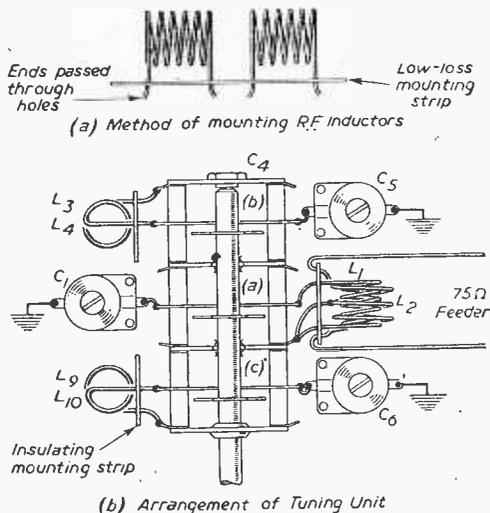
Fig. 20.—Details of the coils and tuning unit.
