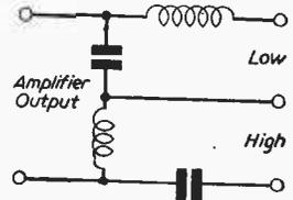
Fig. 3.—A simple cross-over network for dual speakers.
