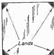
(c) Crystal clamping electrode for AT or BT cut crystals showing the raised lands at each corner.
