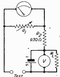
Fig. 5.—Circuit for adjusting shunts.
