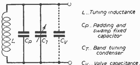
Fig 1.—V.F.O. tuned circuit.
