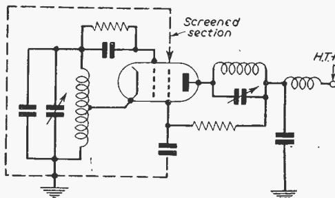
Fig. 5.—"Electron-coupled" form of the grounded anode Hartley. The oscillator output is coupled from the screen-enclosed oscillator section via the electron stream, if a fully screened valve is used.
