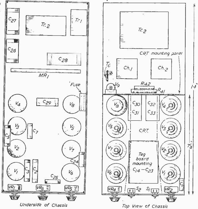
Fig. 5.—Views of the chassis showing layout of essential parts.
