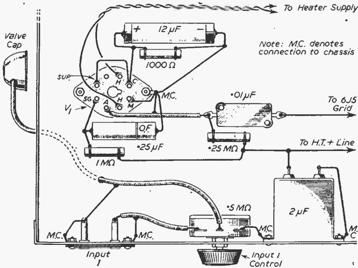
Fig. 2.—Wiring diagram of the 6J7 stage.
