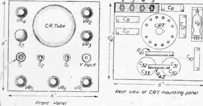
Fig. 3.—Panel and C.R.T. mounting details.
