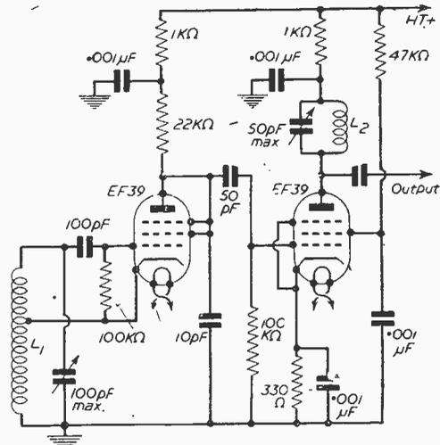
Fig. 47.— $L_1$  consists of 6 $\frac{1}{2}$  turns 18 s.w.g. on a  $\frac{1}{2}$  in. former, tapped 2 turns from the "hot" end.  $L_2$  consists of 2 turns 18 s.w.g. on a  $\frac{1}{2}$  in. former (this coil can be self-supporting).
