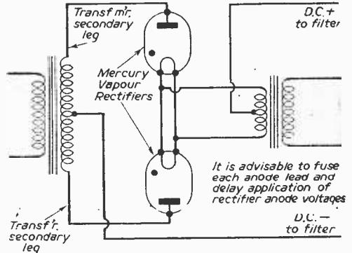
Fig. 1.—Basic circuit of a rectifier unit.
