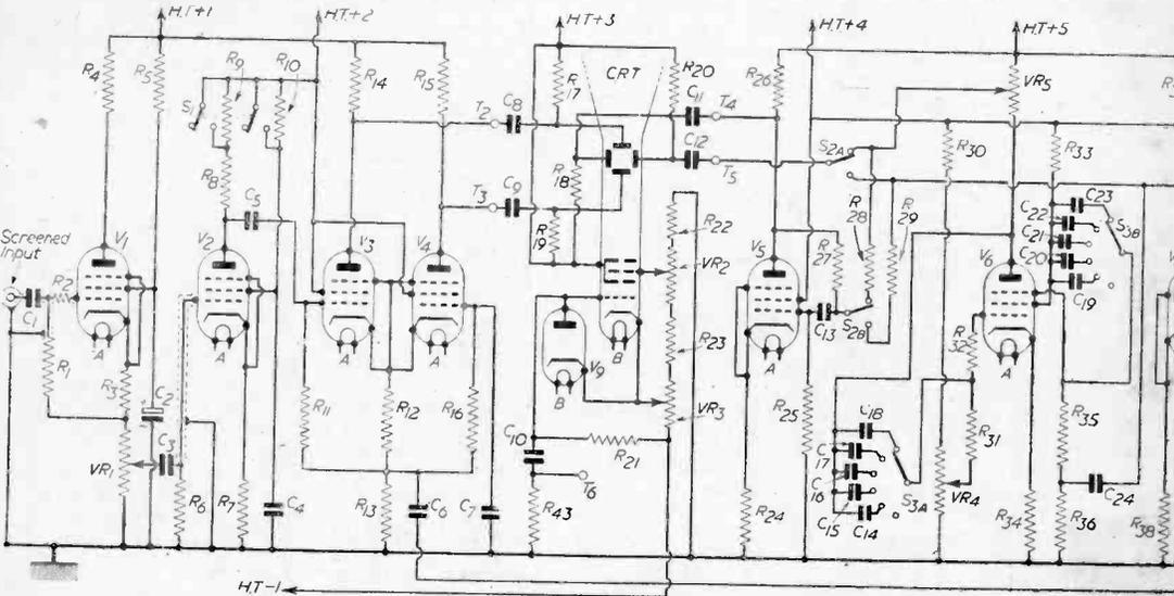
Fig. 1.—Theoretical circuit of the Versatile Oscilloscope.
