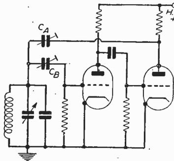
Fig. 8.—The Franklin oscillator.  $C_A$  and  $C_B$  are 0-15 pF. trimmers.
