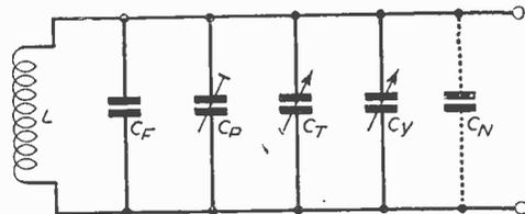
Fig 2.—Practical V.F.O. tuned circuit.  $C_v$  padding condenser (e.g., 500 pF.);  $C_p$  variable padding (band-setter) (e.g., 500 pF.);  $C_t$  main tuning condenser (e.g., 100 pF.);  $C_y$  "QSY" control (e.g., 5 pF.);  $L$  tuning inductance;  $C_n$  optional negative coefficient temperature-compensating condenser (see text).
