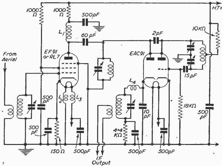
Fig. 54.—Another self-quenched super-regenerative arrangement.
