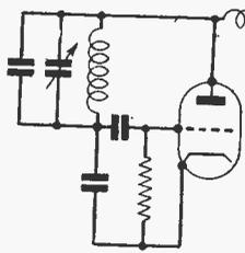
Fig 3. — The Colpitts oscillator.
