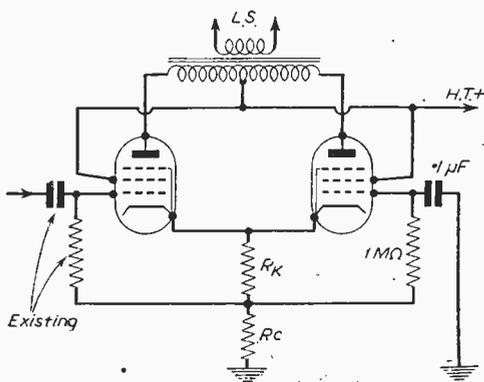
Fig. 1.—Basic circuit of the Schultz phase-splitter.
