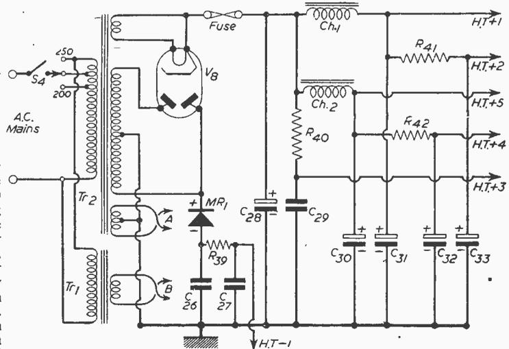
Fig. 2.—Theoretical circuit of the power supply section.
