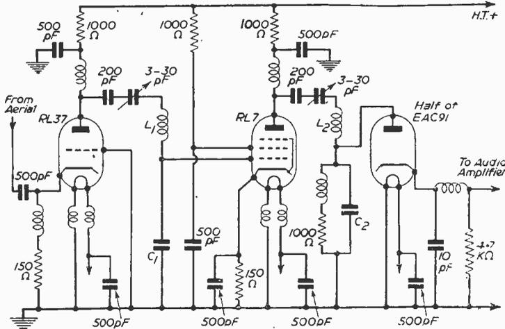
Fig. 49 —A V.H.F. converter.
