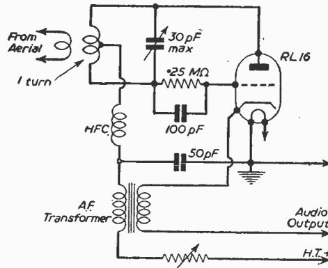
Fig. 53.—One form of super-regenerative circuit.
