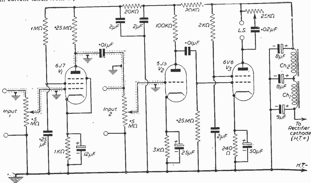
Fig. 1.—Amplifier circuit showing screened leads, etc.
