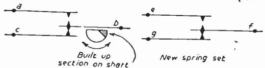
Fig. 6.—Showing the shape of the cam to be built up. Fig. 7.—Diagram of the new spring set arrangement.
