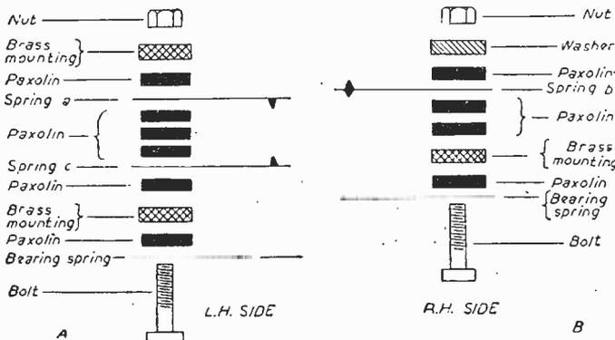
Fig. 8.—Semi-exploded view of the existing spring mounting.
