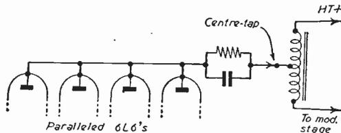
Fig. 3.—Paralleled modulator valves enable higher power output. The centre-tapped high voltage secondary enables a match to be made. A centre-tapped choke is also suitable in such a circuit.
