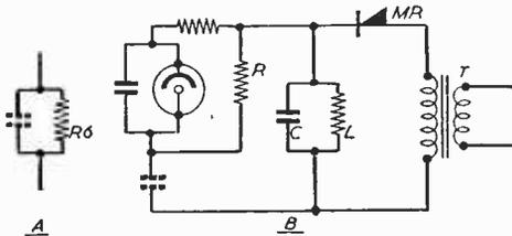
Fig. 2.—“A” shows the discharge resistor in circuit and “B” the simplified circuit of the whole system.
