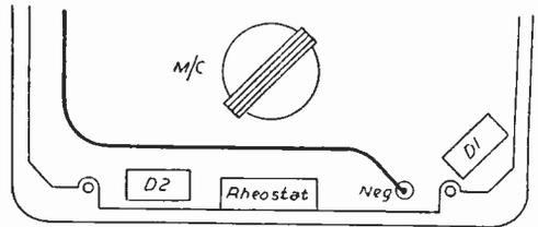
Fig. 14.—The position of the crystals.
