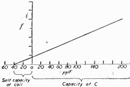
Fig. 2.—A graph of various readings at different frequencies on a "Q" meter in checking the self-capacity of a coil.
