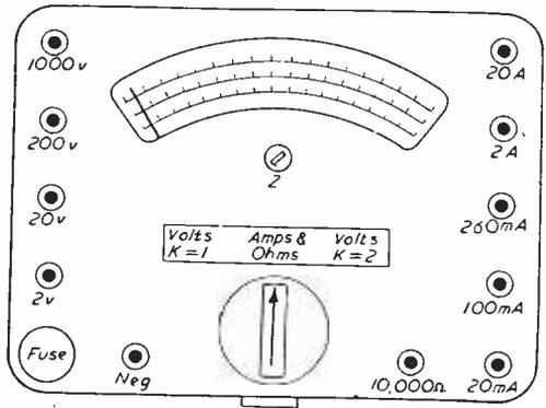
Fig. 1.—Face panel of the meter.
