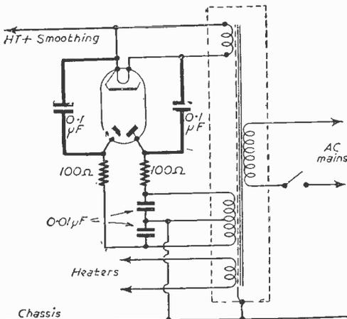
Fig. 1.—The heavy lines show the modifications to be made to avoid modulation hum.
