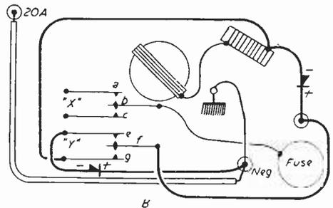
Fig. 13b.—New wiring denoted by heavy lines.
