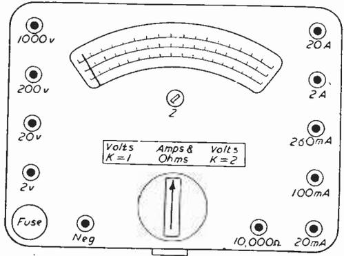
Fig. 1.—Face panel of the meter.
