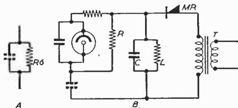
Fig. 2.—“A” shows the discharge resistor in circuit and “B” the simplified circuit of the whole system.
