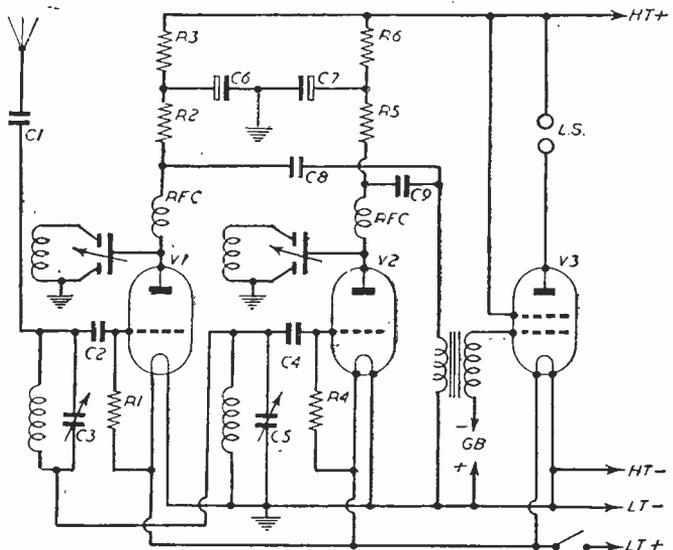
Fig. 1.—A simple dual-channel receiver.
