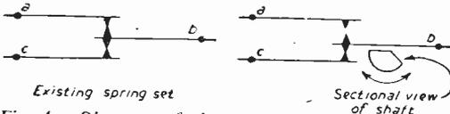
Fig. 4.—Diagram of the existing contacts in the switch.
