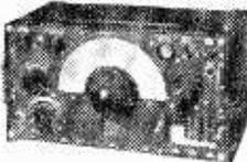
Brand new and unused. 5 Frequency ranges: 12.5-1.5 Mc s.; 7.5-3.0 Mc s.; 1,500-600 Kc s.; 500-200 Kc s.; 200-75 Kc s. Supplied in maker's original wood transit case. LASKY'S PRICE, £11/19/6. Complete. R.1155 Receivers. Second hand, aerial tested. £7/19/6. Carriage and packing 12/6 per unit extra, including 10, which will be refunded on return of packing case.
