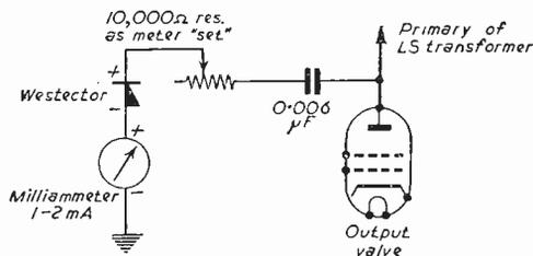
Fig. 6.—A simple output meter.
