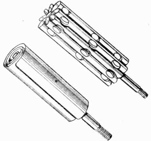
Fig. 50.—Two typical anode designs used in electrolytics.
