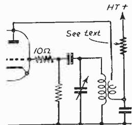
Fig. 5.—Modifying the oscillator section of the frequency changer.
