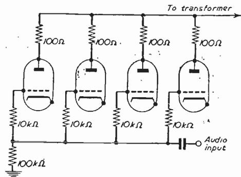
Fig. 4.—Anode and grid stoppers are desirable precautions in the use of paralleled modulator valves.
