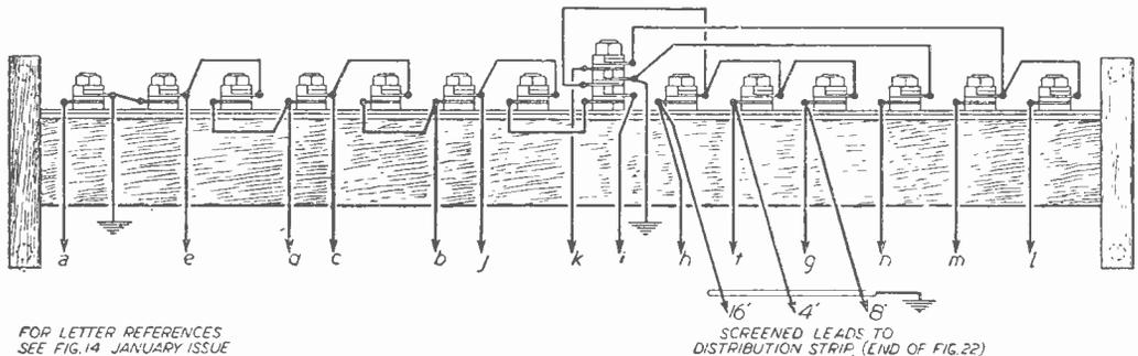
Fig. 23.—Details of connections to the stop-key switches.
