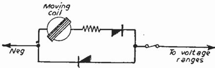
Fig. 2.—Basic circuit.
