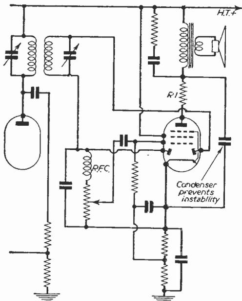
Fig. 1.—Circuit showing how double diode pentode can be used as an output pentode.
