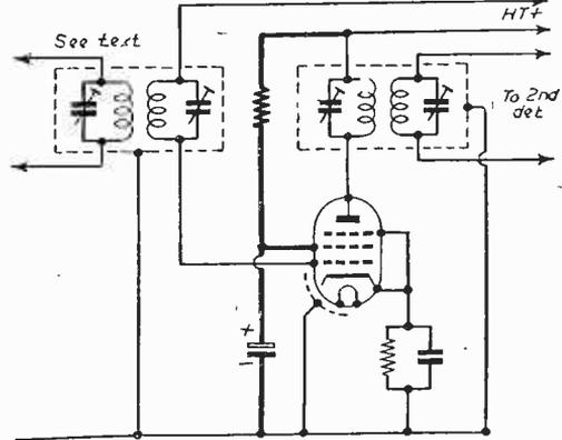
Fig. 4.—Decoupling the screen-grid of an I.F. stage.
