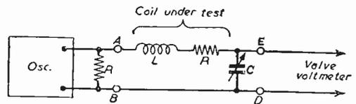
Fig. 1.—Theoretical circuit of an average "Q" meter.
