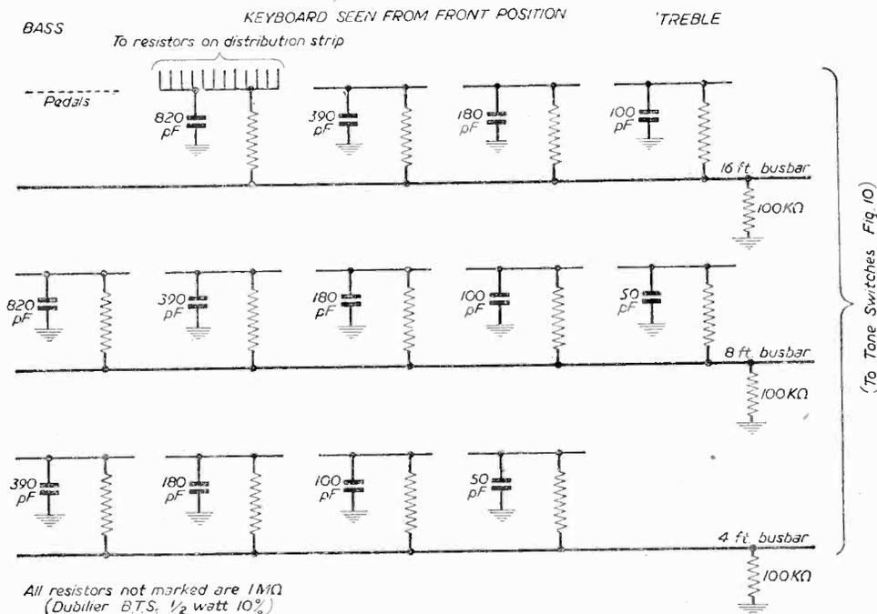
Fig. 22.—Details of main and octave busbar connections—with click filters.
