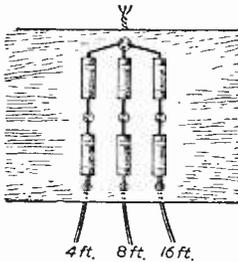
Fig. 24.—Connections to the divider network for the main outputs.
