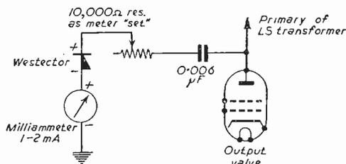
Fig. 6.—A simple output meter.
