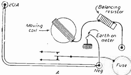
Fig. 13a.—The part of the wiring to be altered.
