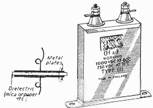
Fig. 46.—Principle of a fixed condenser and a typical "paper" type fixed condenser.
