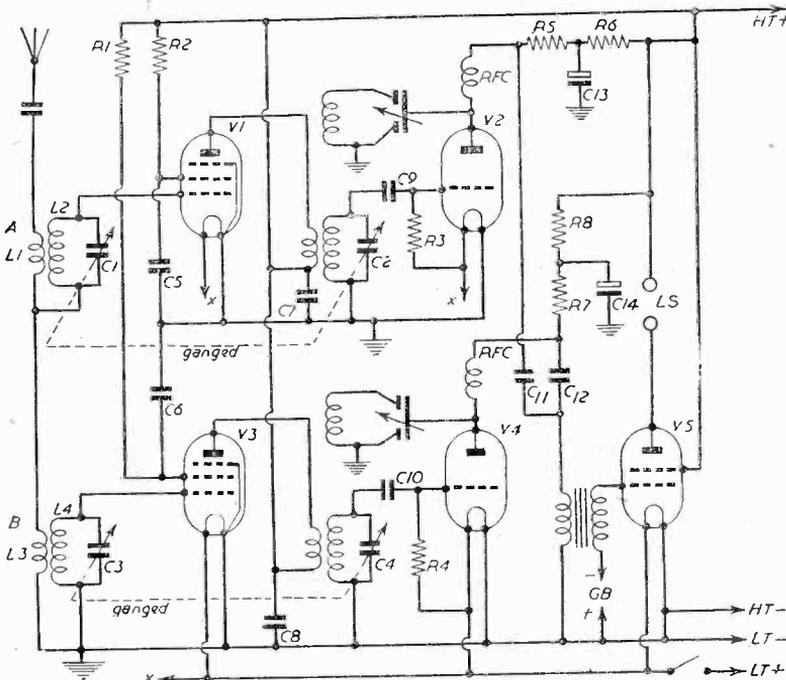
Fig. 2.—A more comprehensive receiver. The wavetraps circuit is associated with V1.
