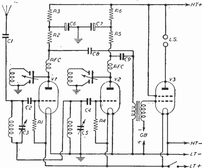
Fig. 1.—A simple dual-channel receiver.
