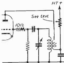
Fig. 5.—Modifying the oscillator section of the frequency changer.
