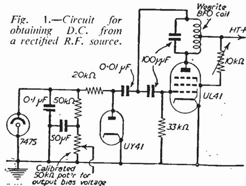
Fig. 1.—Circuit for obtaining D.C. from a rectified R.F. source.
