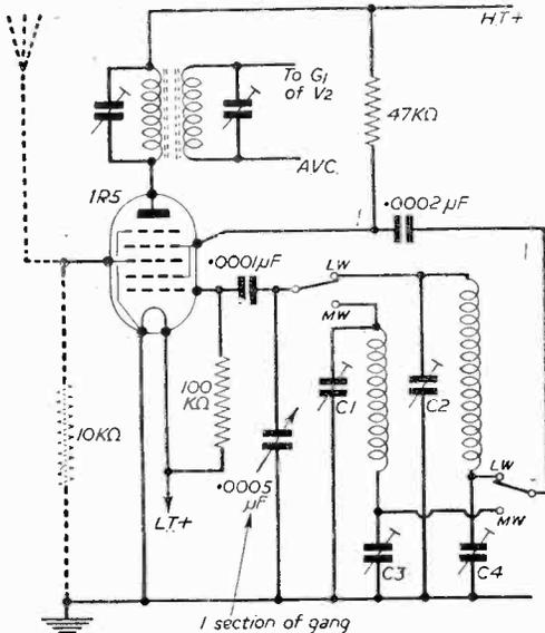
Fig. 1.—Alignment of the oscillator stage.
