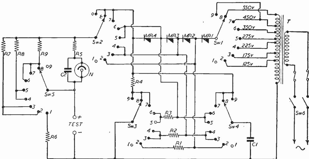
Fig. 1.—Theoretical circuit of the instrument.
