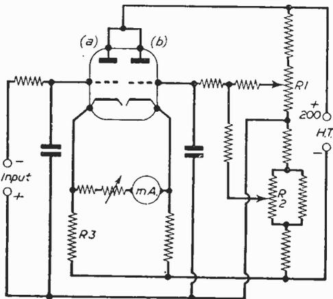
Fig. 27.—A typical valve voltmeter circuit.
