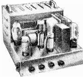
Size approx. 12.9-7in. For A.C. mains 200-230-250v. 50 c/c. Outputs for 3- and 15-ohm speakers. Kit is complete to last nut. Chassis is fully punched. Full instructions and point-to-point wiring diagrams supplied. Unapproachable value at 9 1/4 s.n.s. or ready for use, 50/- extra. Carriage 10/- If required, cover as illustrated can be supplied for 17/6.
