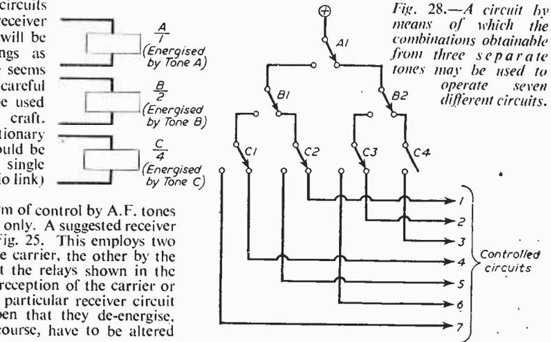
Fig. 28.—A circuit by means of which the combinations obtainable from three separate tones may be used to operate seven different circuits.
