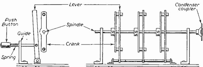
Fig. 2.—System operated by levers.
