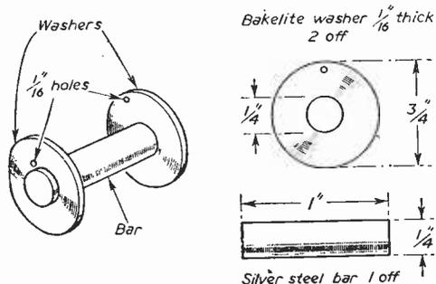
Fig. 2.—The solenoid or winding, fitted with bakelite cheeks.
