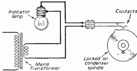
Fig. 4.—Tuning with a bulb indicator.
