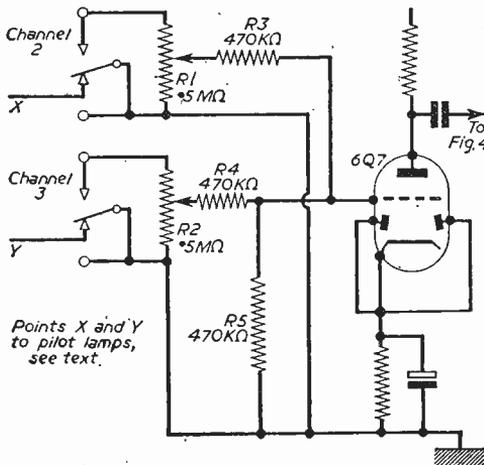
Fig. 2.—The inputs of Channels II and III.
