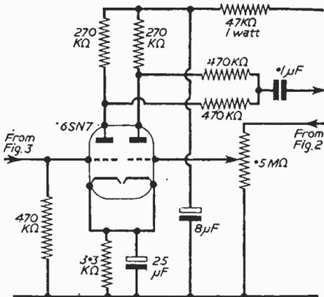
Fig. 4.—Mixer Channels I, II and III.
