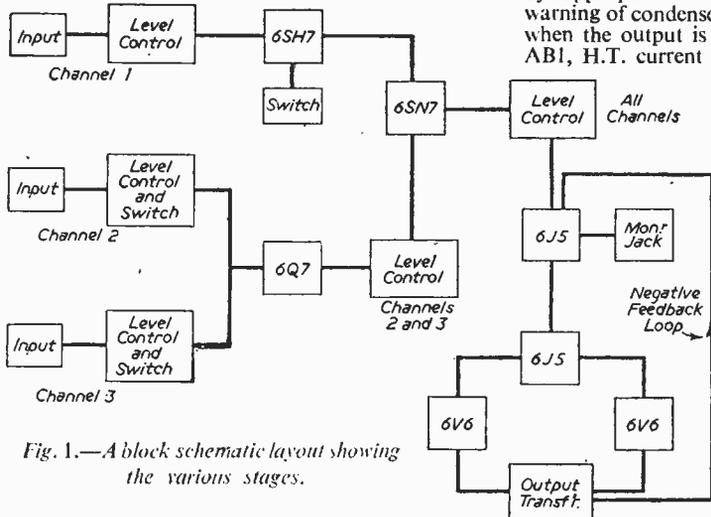
Fig. 1.—A block schematic layout showing the various stages.
