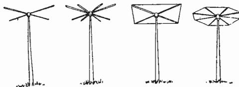
Fig. 6.—Various forms of top-loading skeleton capacities.
