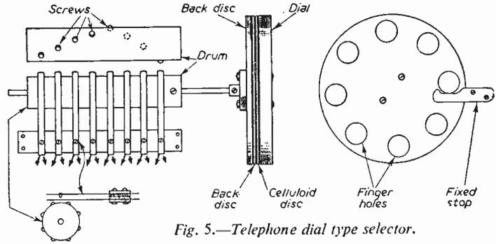
Fig. 5.—Telephone dial type selector.
