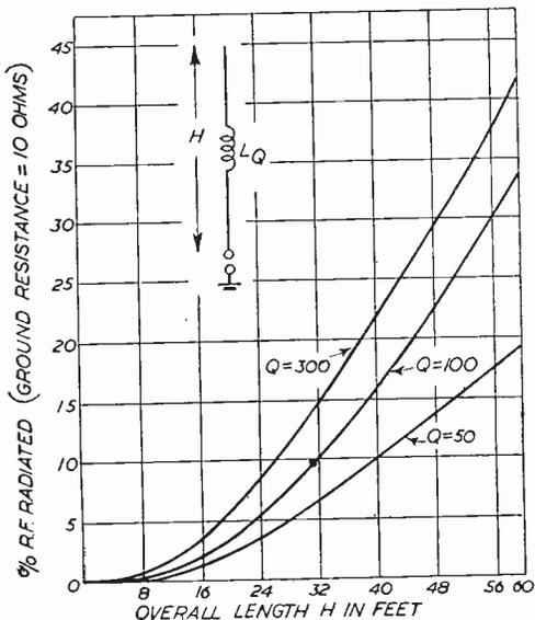
Fig. 5.—Topband efficiency of centre-loaded wires.
