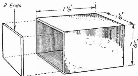
Fig. 1.—The base, made from aluminium tube.
