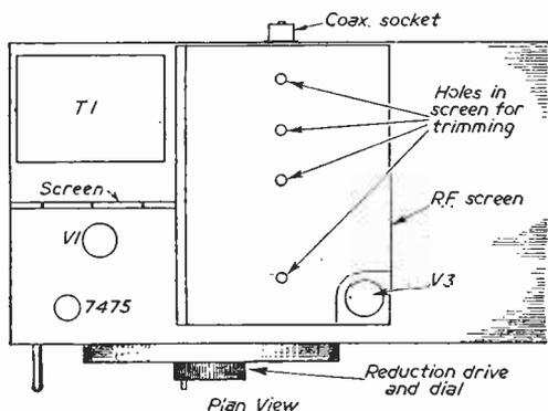
Fig. 1.—Top chassis lay-out.
