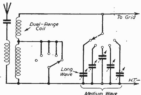
Fig. 2.—Circuit for dual-wave operation.
