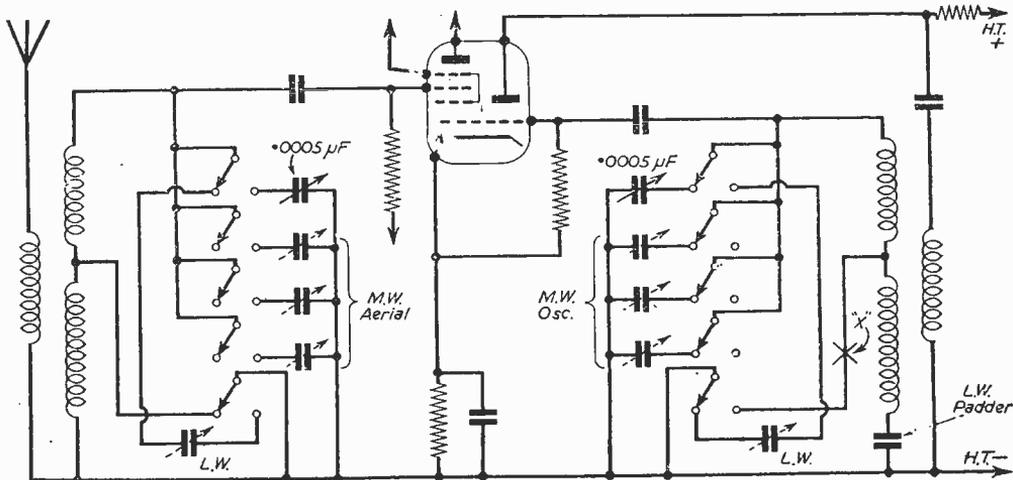
Fig. 4.—Push-button type switching.
