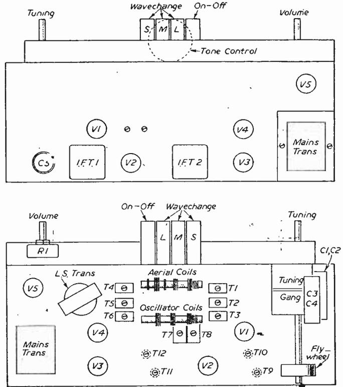
Figs. 2 and 3.—Top and underside views of the chassis showing valve layout and positions of trimmers.
