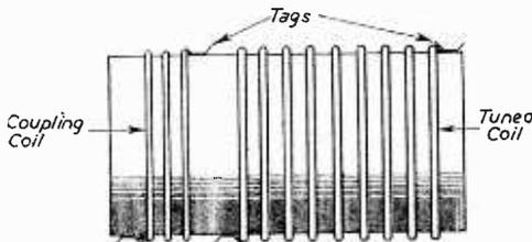
Fig. 6.—A typical short-wave coil, showing how the turns are spaced.
