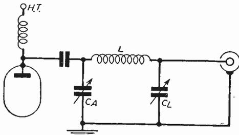
Fig. 1.—The conventional Pi network tank circuit components.
