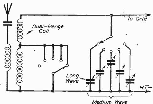
Fig. 2.—Circuit for dual-wave operation.
