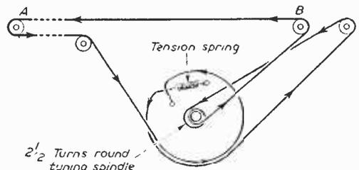
Fig. 1.—Details of the tuning drive.
