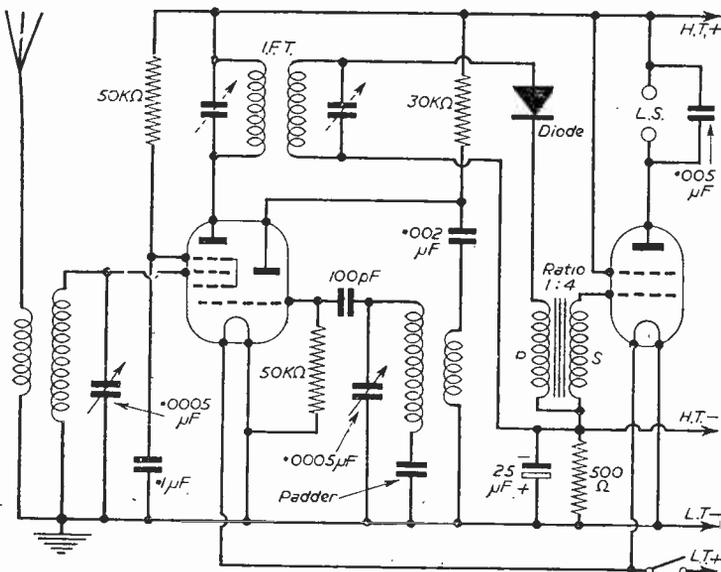
Fig. 1.—2-valve circuit with crystal diode.
