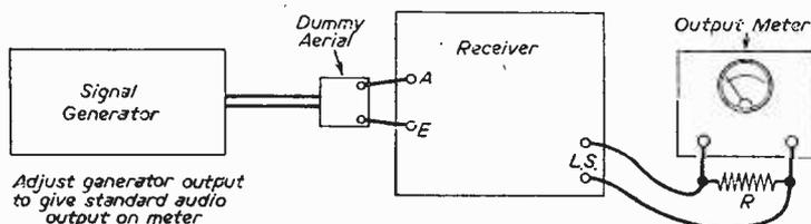
Fig. 38.—An arrangement for measuring the sensitivity of a broadcast receiver.
