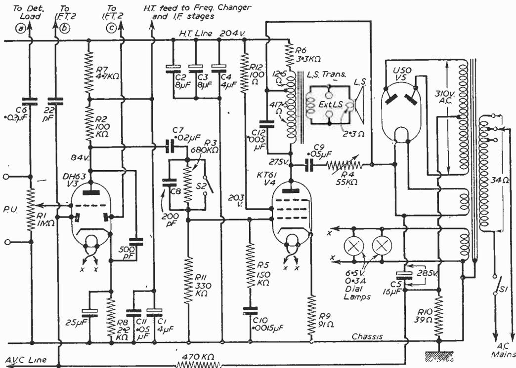
Fig. 4.—Theoretical circuit of the A.F. and Power Pack sections of the G.E.C. BC4850 series.
