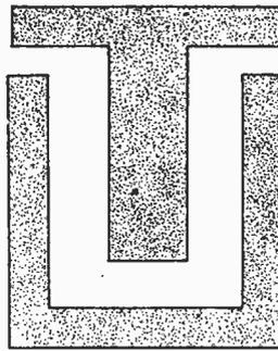
Figs. 1 to 4.—The usual "T" and "U" laminations, core measurements and the bobbin.
