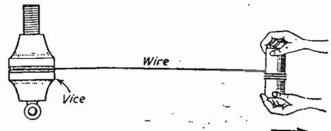
Fig. 8.—A suggested method of winding short-wave coils.
