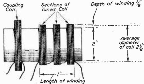
Fig. 5.—Illustrating the long-wave coil mentioned in the text. (The coil need not necessarily have three sections; four could be used in this case, if desired.)
