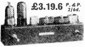
Fits neatly into your record player or portable gramophone leaving room for speaker. Dimensions 10in. x 3 1/2in. x 2in. 4 watts quality output. Suitable for all speakers and with standard or L.P. pickups. Built-in power pack, 200-250 v. A.C. Valves 6J7 and 6V6 available at 20/- for the pair if required.
