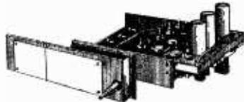
Input 300 ohm balanced line or 80 ohm coax. Coverage 180-200 Mc/s. Vision I.F. — 10.7 Mc/s. Valve line-up 6AK5 R.F. amplifier, 6AK5 mixer, 6C4 separate oscillator. This is a high gain unit, ideal for fringe areas. Can also be used as FM, TUNER. Frequency coverage 80-100 Mc/s. I.F. 10.7 Mc/s. Size 9in. wide, 6 1/2 in. deep, 4in. high, 9in. scale, width including overlap 14in. Complete with 3 valves. P. & P. 3/-. £4/9/6. 10.7 Mc/s I.F.'s to suit above, 4/6 each.
