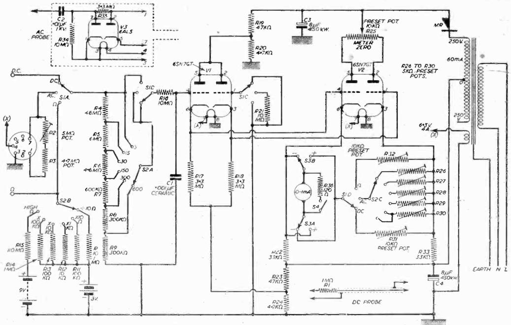
Fig. 1.—Theoretical circuit of the Meter. R and C details are given and the remaining components are listed on page 664.
