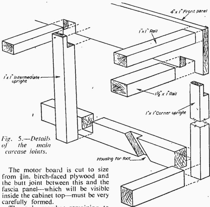
Fig. 5.—Details of the main carcase joints.
