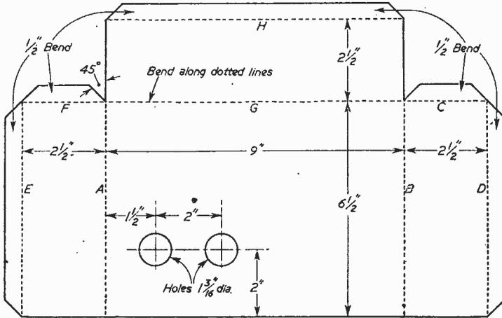
Fig. 3.—Chassis bending and drilling data.
