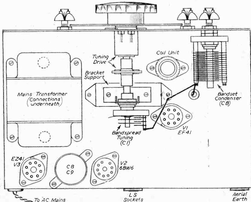
Fig. 5.—Above chassis wiring and layout details.
