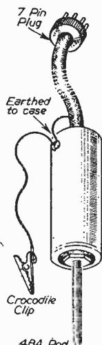
Fig. 8.—The A.C. probe.
