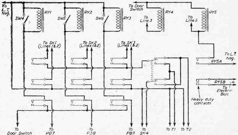
—Complete relay unit wiring.
