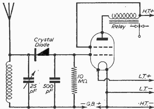
Fig. 2.—A diode-valve circuit.
