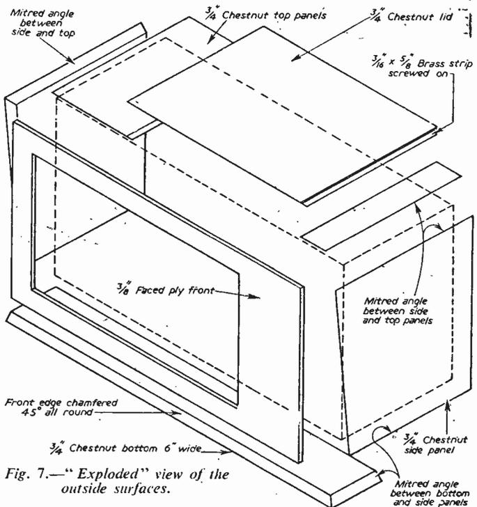
Fig. 7.—“Exploded” view of the outside surfaces.
