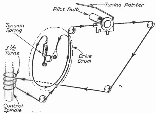
Fig. 4.—Details of the dial drive.
