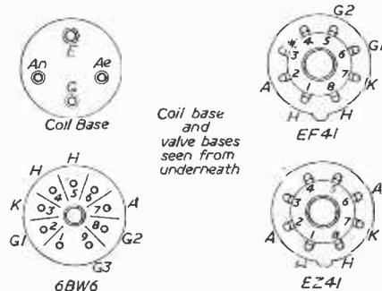
Fig. 7.—Details of valve base connections.
