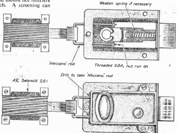
Figs. 5 and 6.—Cylinder lock modifications.
