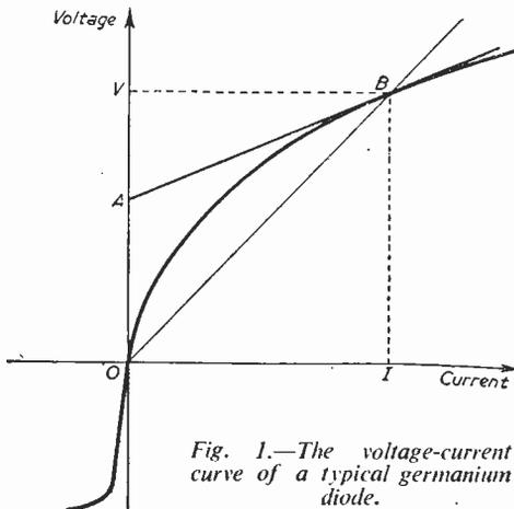
Fig. 1.—The voltage-current curve of a typical germanium diode.
