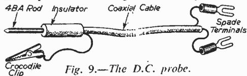
Fig. 9.—The D.C. probe.
