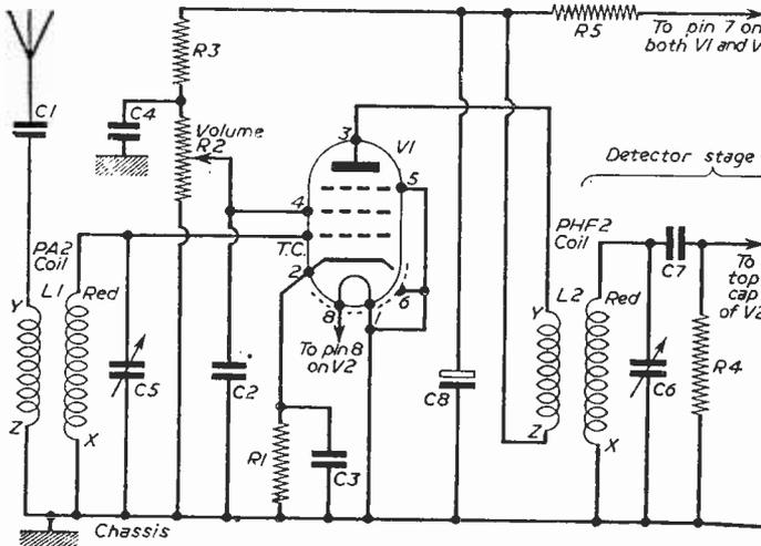
Fig. 18.—Theoretical circuit of H.F. stage.
