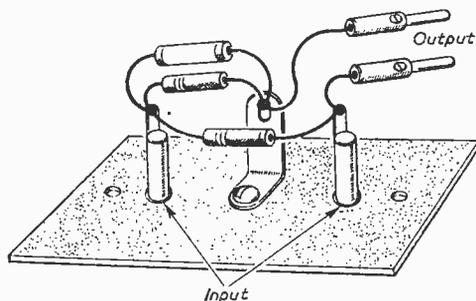
If desired a small wooden box can be made with one side open so that the sockets can be screwed on to it with the "works" inside, and a small hole for the leads to be taken through.
