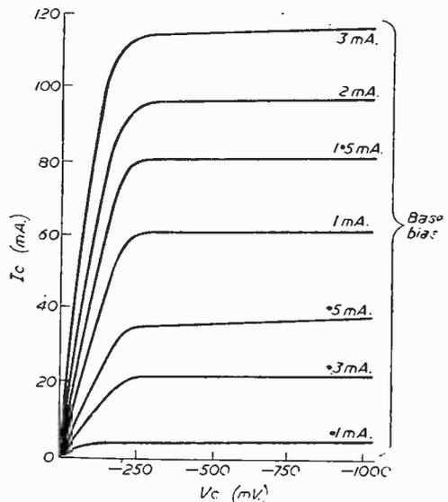
Fig. 39.—Low voltage collector characteristic—OC72.
