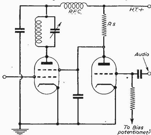
Fig. 3.—The conventional clamp tube modulator is, in effect, a resistance coupled screen grid modulator.
