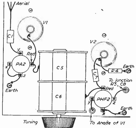
Fig. 19.—Top view of H.F. and detector stages.
