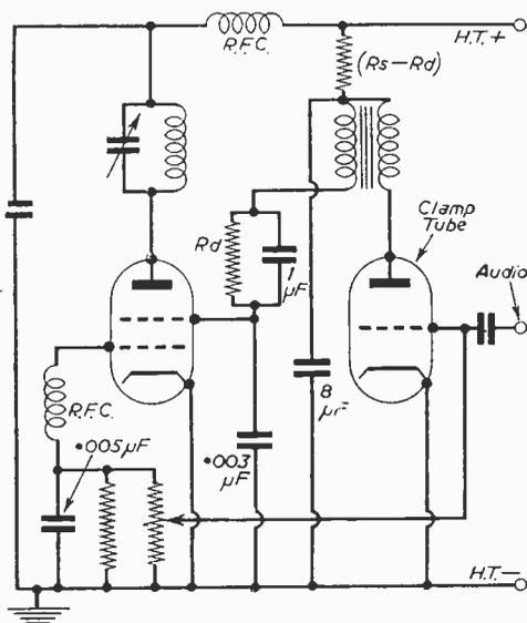
Fig. 6.—A small by-passed auxiliary dropper resistor ( $R_d$ ) enables fuller modulation to be obtained. If  $R_d$  exceeds 1,000 ohms, the screen resistor should be reduced in value to compensate.
