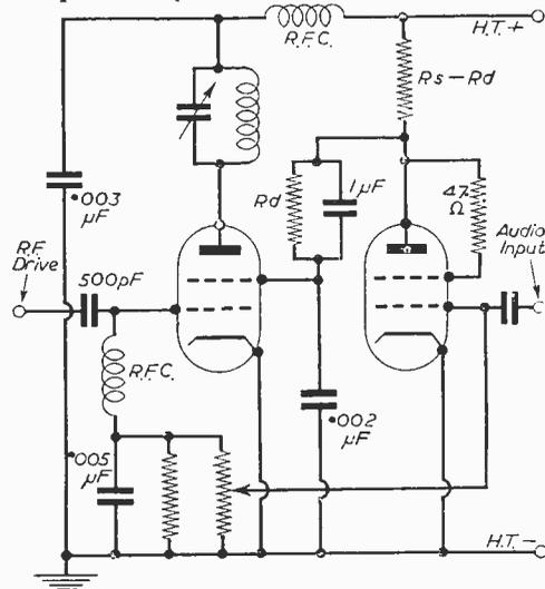
Fig. 7.—A by-passed auxiliary screen dropping resistor will enable even the simple clamp tube modulator to give deeper modulation. The clamp tube operates at a higher voltage than the P.A. screen, and is thus enabled to swing the screen volts to nearly zero volts. The auxiliary resistor should be a few thousand ohms.
