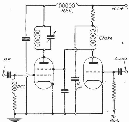
Fig. 2.—A choke coupled screen modulator.
