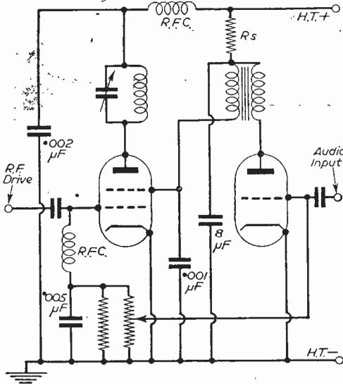
Fig. 5.—Transformer coupling combined with the conventional clamp valve permits of more effective screen modulation.
