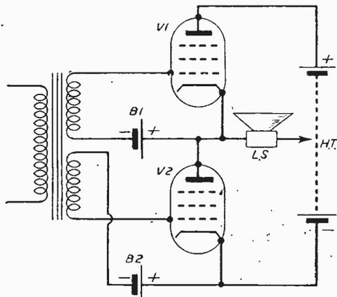
Fig. 3.—The single-ended push-pull output stage, using a tapped H.T. battery.
