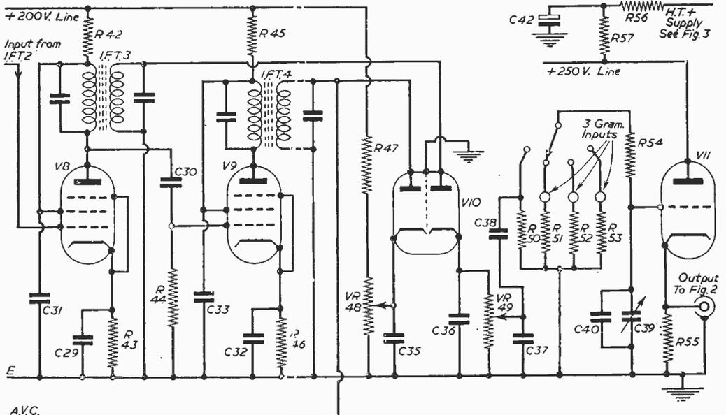
Fig. 1(b).—Circuit of the I.F.s and detector, with the first audio stage.
