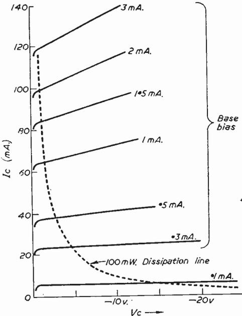
Fig. 42.—Collector characteristic—OC72.
