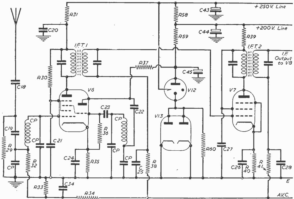
Fig. 1(a).—Circuit of the feeder section.
