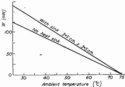
Fig. 40.—Dissipation characteristic—OC72.
