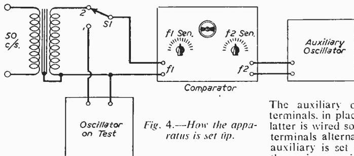
Fig. 4.—How the apparatus is set up.
