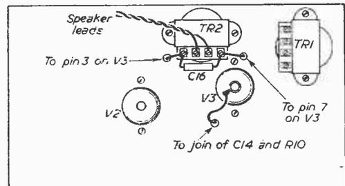
Fig. 17.—Additional wiring when V3 is fitted (top view of chassis).
