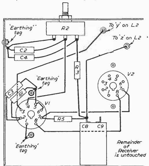
Fig. 21.—View of the underside wiring added to complete H.F. stage.
