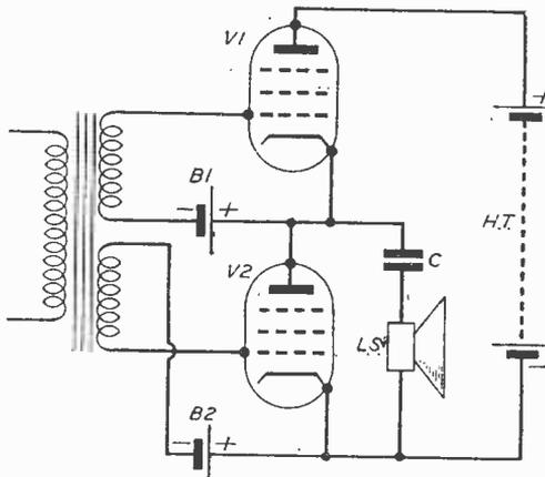
Fig. 4.—The H.T. tap can be avoided by the use of a coupling capacitor, C.
