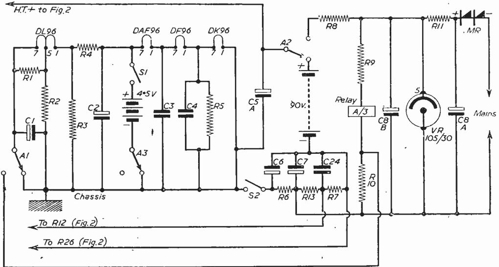
Fig. 1.—The power supply circuit.
