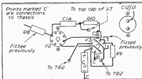
Fig. 16.—New wiring added when fitting V3 (view of underside of chassis).
