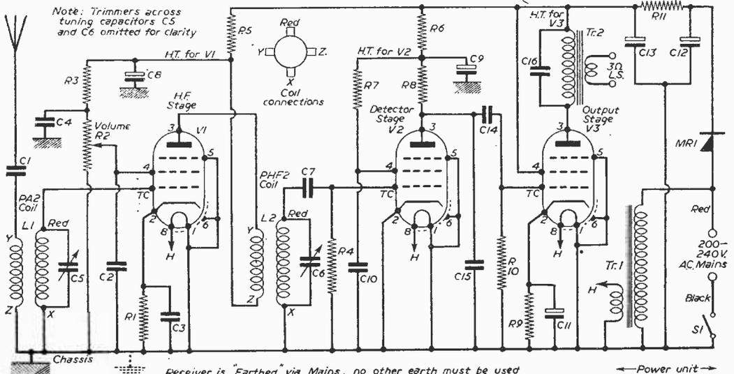
Fig. 22.—The theoretical circuit with this month's additions.
