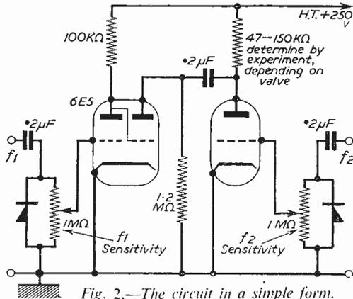
Fig. 2.—The circuit in a simple form.
