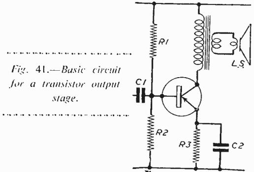
Fig. 41.—Basic circuit for a transistor output stage.
