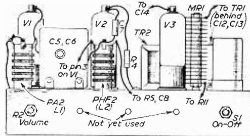
Fig. 20.—Side view of the receiver with this month's modifications.
