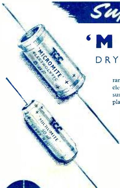
These small but high quality electrolytics have proved so popular that the range has been greatly extended. The use of high-gain etched foil electrodes keeps size and weight down, making the condensers suitable for suspension wiring. Conservatively rated; long shelf life ensured; green plastic insulating sleeving prevents short-circuits.
