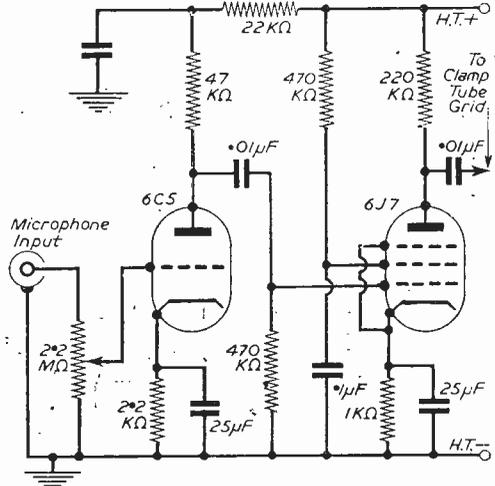
Fig. 4.—A simple two-stage speech amplifier preceding the clamp valve is adequate to give good modulation from a crystal microphone. The current taken need only be a few milliamperes at, say, 250 volts. The preamplifier may generally be fed from the transmitter power supplies without need for a separate power pack.
