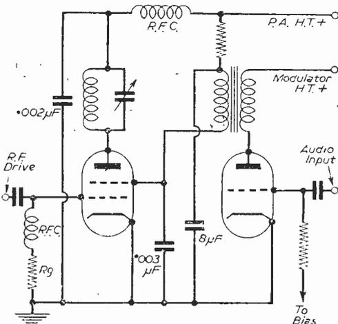
Fig. 1.—A conventional transformer coupled screen modulation circuit.
