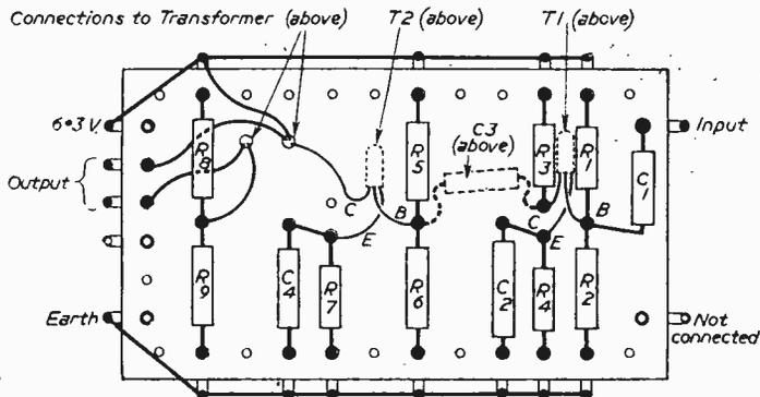
Fig. 47.—Tagboard layout of the audio amplifier.
