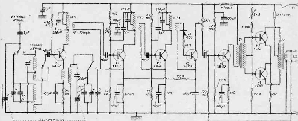
Fig. 1.—Circuit of the Ace transistor portable.
