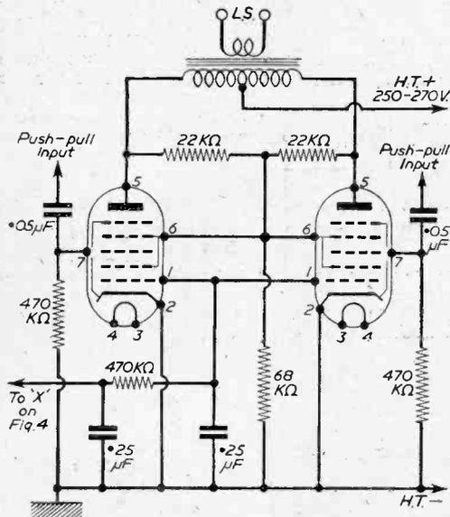
Fig. 2.—Circuit of the output stage of the recorder.
