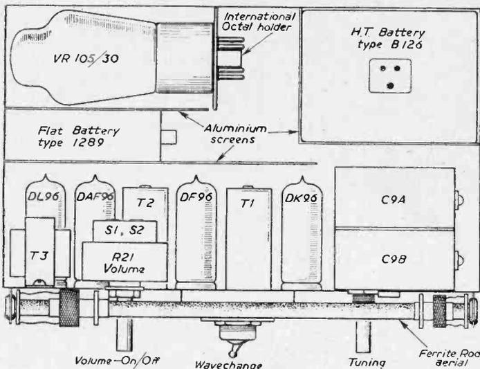
Fig. 5.—Layout of the receiver. The chassis measures 4in. by 2½in.
