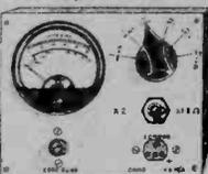
Comprising 2in. moving coil meter, scale calibrated in AC/DC volts, ohms and milliamps. Voltage range AC/DC 0-50, 0-100, 0-250, 0-500. Milliamps 0-10, 0-100. Ohms range 0-10,000. Front panel, range switch, wire-wound pot. (for ohms zero setting), toggle switch, resistor and rectifier. In grey hammer finish case.
