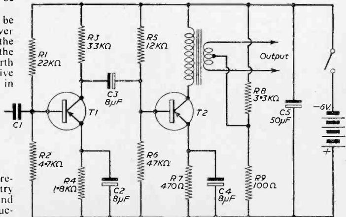
Fig. 46.—A two-stage audio amplifier with output base potentiometer.
