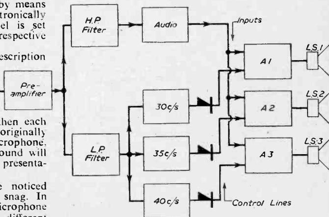
Fig. 1.—Block schematic of a professional form of single track recorder.
