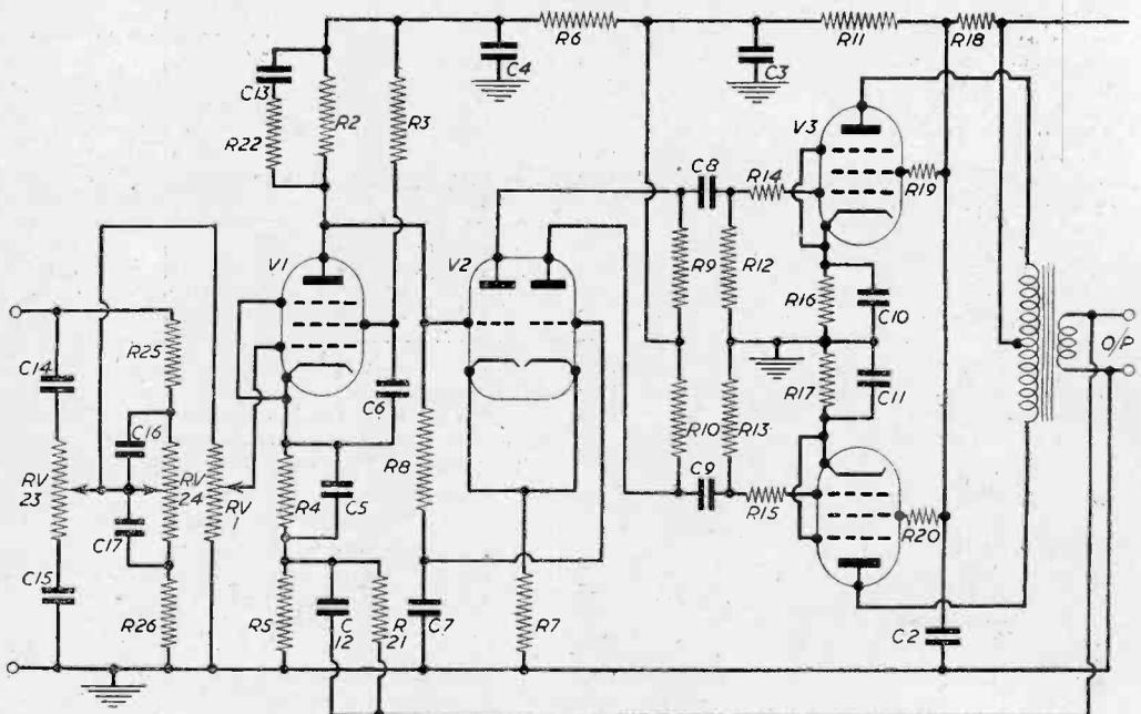
Fig. 2.—The Mullard 5-10 amplifier which the author used in this receiver. If any other amplifier is used the cabinet to be described will have to be modified.
