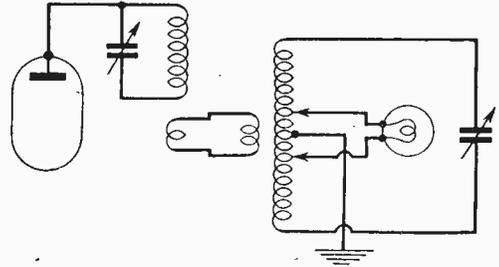
Fig. 6.—The artificial parallel tuned circuit arranged to simulate a parallel tuned twin wire feeder system.
