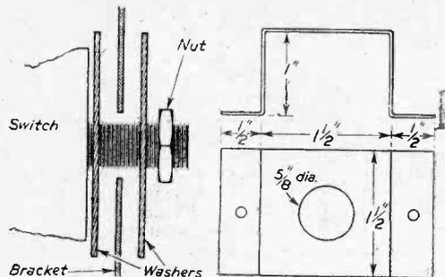
Fig. 4.—Details of wavechange switch mounting.
