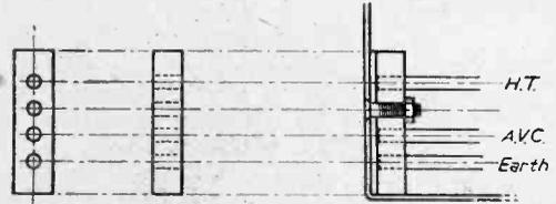
Fig. 6.—Construction of the bus-bars.
