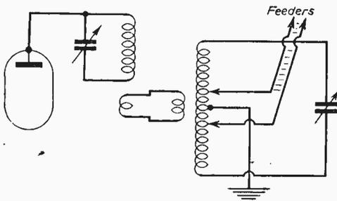
Fig. 7.—Radiating aeriels with twin wire feeders are fed in this manner from a parallel tuned circuit.
