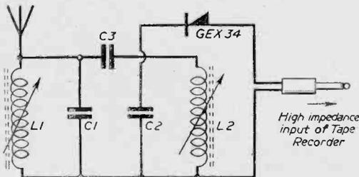
Fig. 1.—Theoretical circuit of the radio jack.
