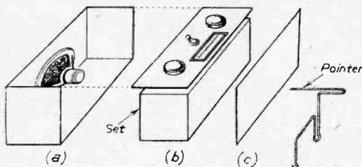
Fig. 7.—How the cabinet is made up, and the dial pointer.
