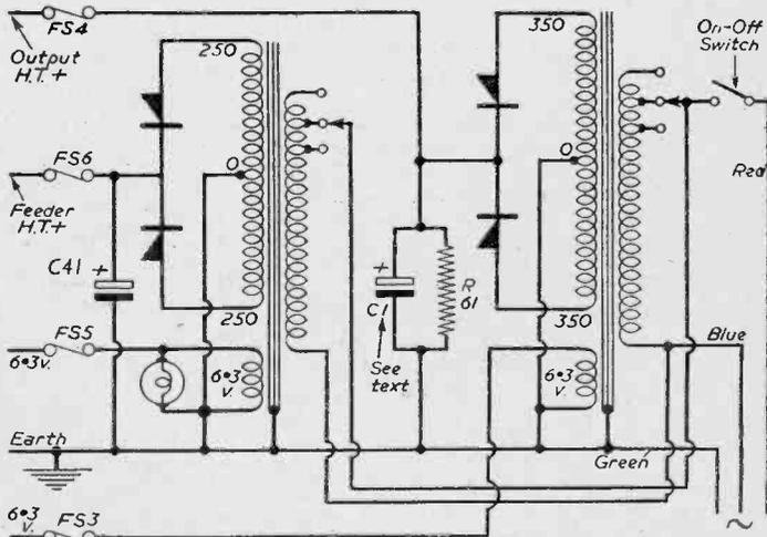
Fig. 3.—Circuit of the power supply.
