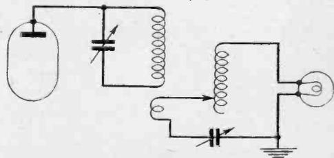
Fig. 2.—A series tuned artificial aerial circuit using a lamp bulb as a combined load and power output indicator.
