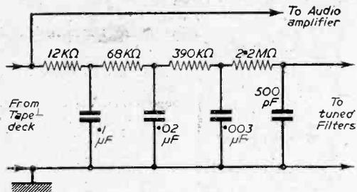
Fig. 3.—The low-pass filter which is employed.
