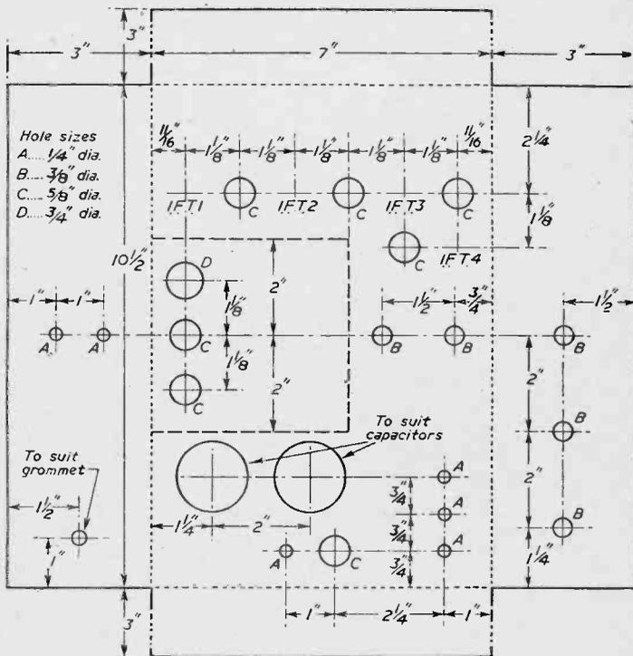
Fig. 5.—Drilling details for the feeder unit chassis.
