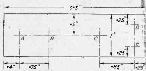
Fig. 2.—Details of the "chassis."
