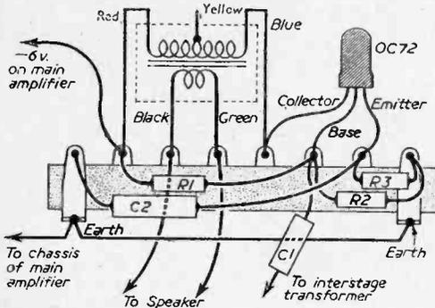
Fig. 45.—Wiring diagram of the audio stage.
