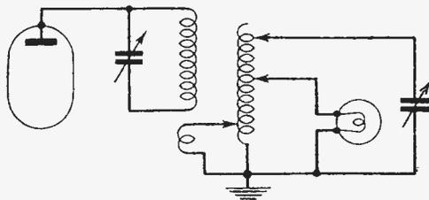
Fig. 3.—A parallel tuned artificial aerial using a lamp bulb as load and indicating device.
