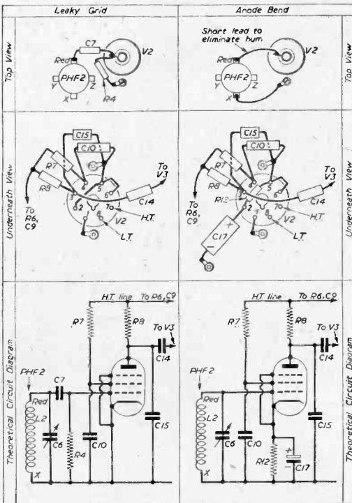
Fig. 24.—Grid leak and anode bend detector stages.
