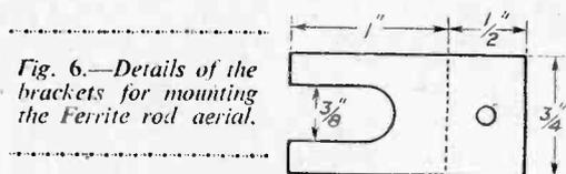
Fig. 6.—Details of the brackets for mounting the Ferrite rod aerial.
