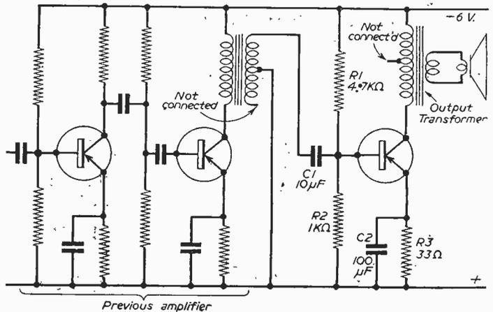
Fig. 44.—Circuit of the complete amplifier.
