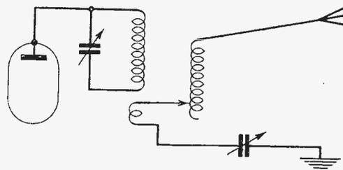
Fig. 4.—The series tuned Marconi aerial corresponds to the artificial aerial equivalent shown in Fig. 2.
