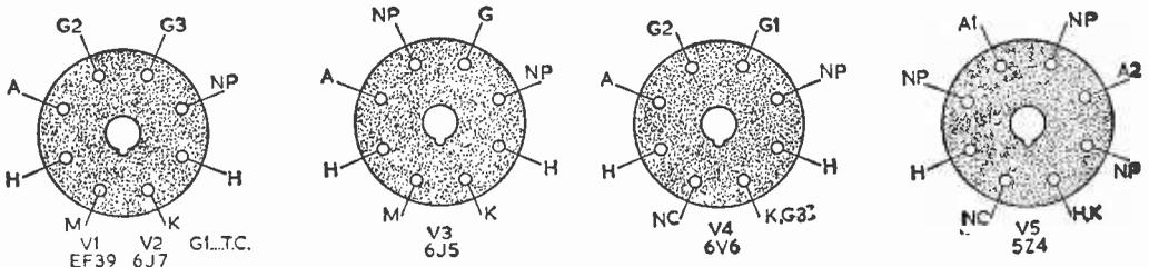
Fig. 7.—The valve base connections.
