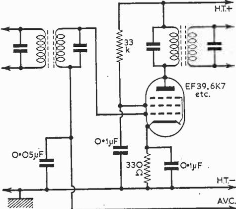
Fig. 7.—An I.F. stage with a dropper for the screen grid.
