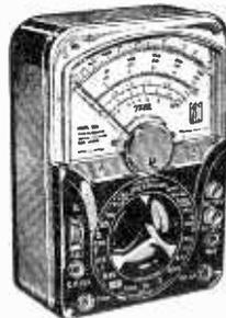
**30,000 O.P.V. Model 506.** Volts to 1,000 D.C. at 30,000 O.P.V., A.C. at 20,000; 12 Amps D.C. Current; 60 Megs Resistance; -20 to +56 Dbs; Internal buzzer short circuit warning. Size 3 5/16 in. x 6 5/16 in. x 2 1/2 in. **£8.19.6**
