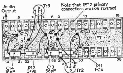
Fig. 19.—The wiring of the extra components necessary for neutralisation of the I.F. amplifier (see text).
