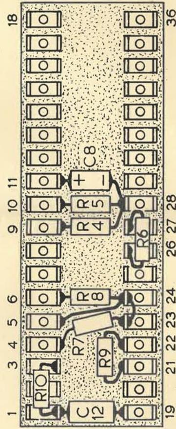
Fig. 10 - WIRING OF RESISTORS AND CAPACITORS
