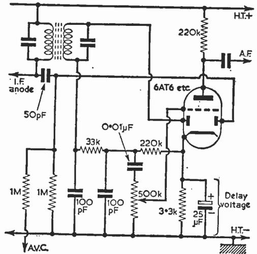
Fig. 5.—Double diode triode circuit with cathode bias.
