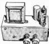
★ A UCL 82 valve provides a triode amplifying stage, and a pentode output stage (3 watts), enabling good amplification and sparkling reproduction to be combined with physical compactness (amplifier size, 7 x 3½ x 6½ in. high).
