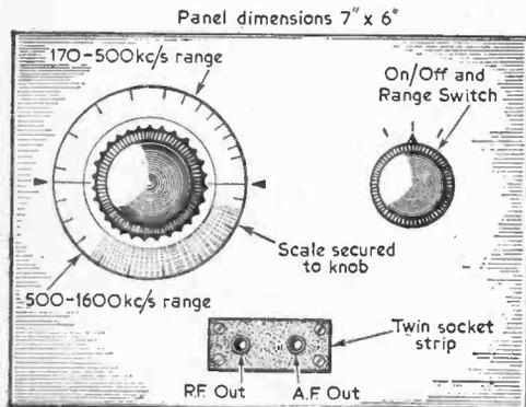
Fig. 2.—The layout of the front panel.
