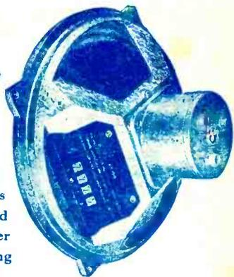
This range of Stentorian loudspeakers, incorporating the patented cambric cone, was developed to provide reproduction that takes full advantage of the television and V.H.F. sound transmissions and high fidelity recordings now available. The cone of the loudspeaker is made from uncured cambric and bonded pulp, the whole being completely cured together and made into one composite cone.
