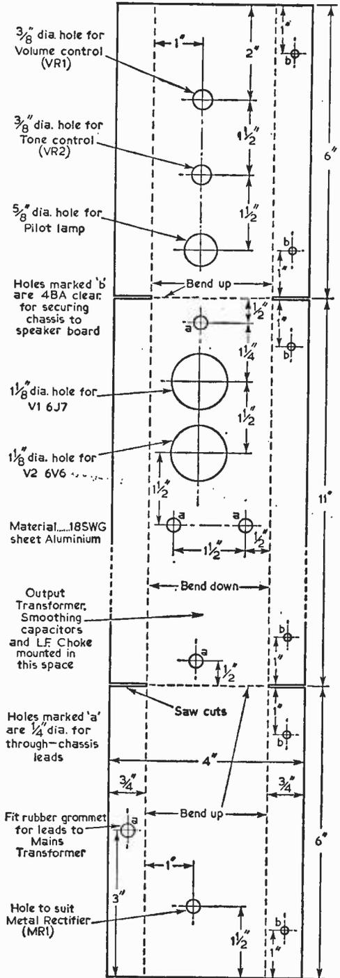
Fig. 4.—The chassis drilling details.
