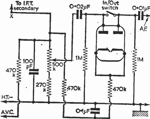
Fig. 3 (above).—A double diode full-wave noise limiter.
