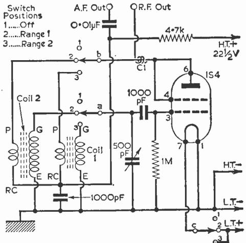
Fig. 1.—The circuit of the instrument.
