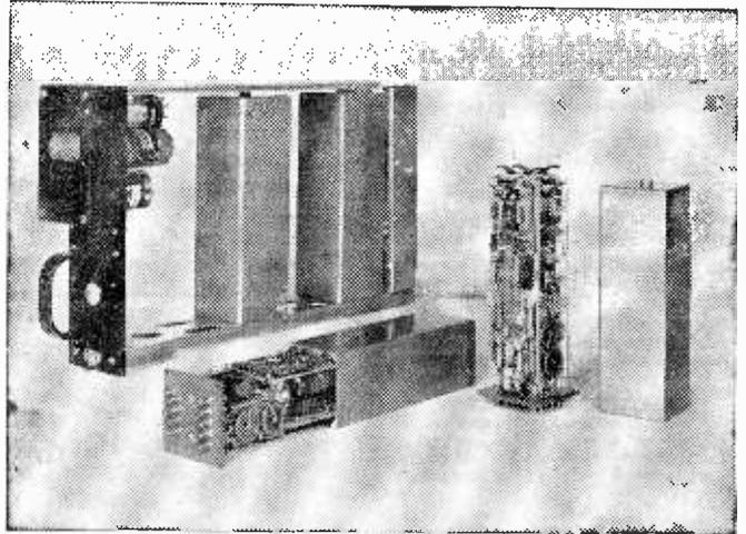
The Marconi navigation unit type 6402 with two of the sealed modules opened for maintenance. Each module may be reassembled and sealed with only four screws, and filled with dry nitrogen to give the added protection of a dry, inert atmosphere.
