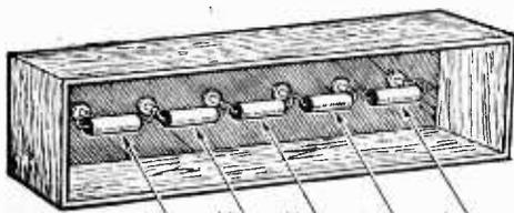
Fig. 6.—Rear view of the volt-box showing the resistors in position.
