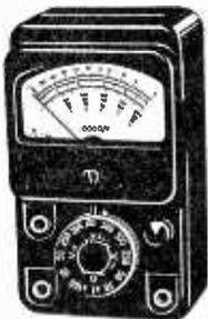
**1,000 O.P.V. Model U.I.** Reads A.C. & D.C. Volts up to 1,000; D.C. Current to 500 mA; Resistance to 200K. Basic movement 300 $\mu$ A. Easily read open scale. Size 5 1/2 in. x 3 1/2 in. x 2 1/2 in. **£2.19.6**
