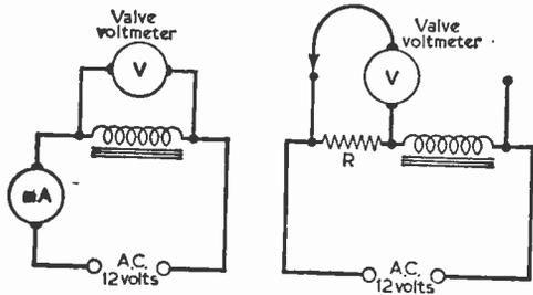
Fig. 1 (left).—Testing an A.F. choke.
