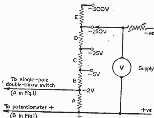
Fig. 3 (above).—Circuit for testing high-range meters.
