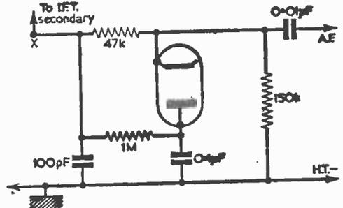
Fig. 2.—Another single diode limiter (see also Fig. 1).
