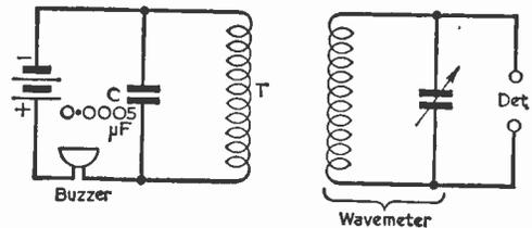
Fig. 3.—Testing an R.F. coil.
