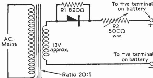
Fig. 1.—The circuit of the instrument.
