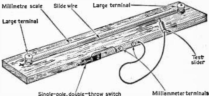
Fig. 1.—The basic slide wire potentiometer.
