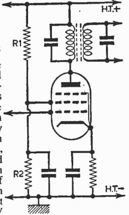
at about the usual figure. The lower the value of these resistors, the more stable will the screen grid voltage become. Unfortunately, very low values are impossible because the bleeder current taken from the H.T. supply would be excessive. Even quite high values will, however, help to avoid so much fluctuation in voltage. A total value of about 50k will require an additional H.T. current of 5mA, with a 250V supply.
