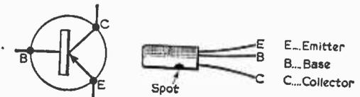
Fig. 2.—The connections of a transistor.
