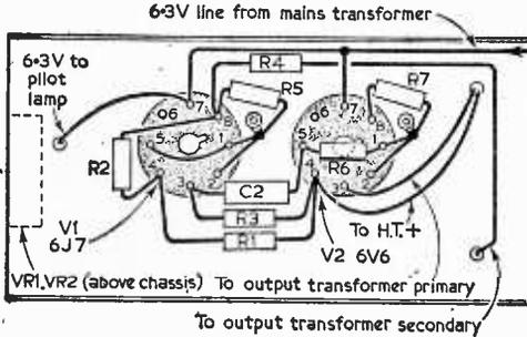
Fig. 3.—The under-chassis wiring.
