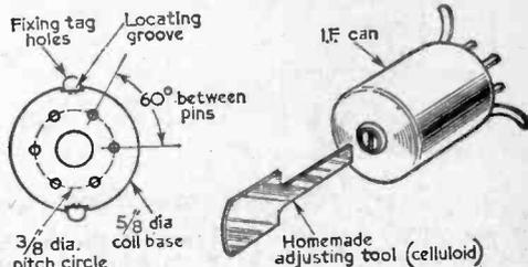
Fig. 15 (left).—The layout of the coil pins (actual size).
