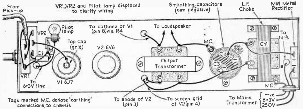
and C4 in conjunction with the choke Ch1 and, as the hum is very well taken care of by negative feedback, it is not necessary that the choke should have a large inductance.
