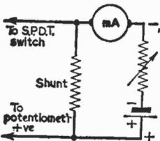
Fig. 5 (left).—Testing a milliammeter.
