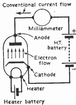
Fig. 1.—The current flow through a diode valve.
