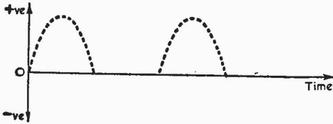
Fig. 5 (above).—The voltage output from a half-wave rectifier.
