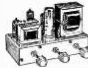
Designed for Hi Fi reproduction of records. A.C. Mains operation. Ready built on plated heavy gauge metal chassis, size 7 1/2 in. w. x 4 in. d. x 4 1/2 in. h. Incorporates EOC83, EL84, EZ80 valves, heavy duty double wound mains transformer and output transformer matched for 3 ohm speaker, separate Bass, Treble and volume controls. Negative feed back line. Peak output 4 1/2 watts. Front panel can be detached and leads extended for remote mounting of controls.
