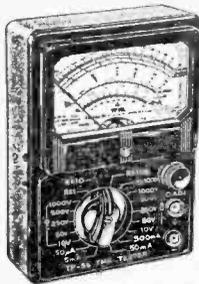
**20,000 OHMS PER VOLT MODEL TP-5S** (Illustrated). Reads voltages up to 1,000 V.C. at 20,000 ohms per volt and A.C. at 10,000 ohms p.v.; D.C. current to 500 mA; Resistance to 10 Mega. Capacitance to 0.1 μF; Decibels from -20 to +36. Size 3 1/2 x 5 1/2 x 1 1/2 in. £5.19.6.
