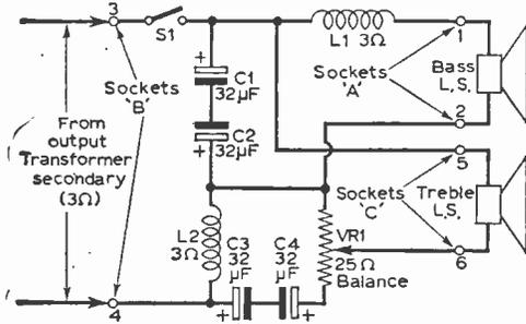
Fig. 1: The simple circuit of the Euphon.
