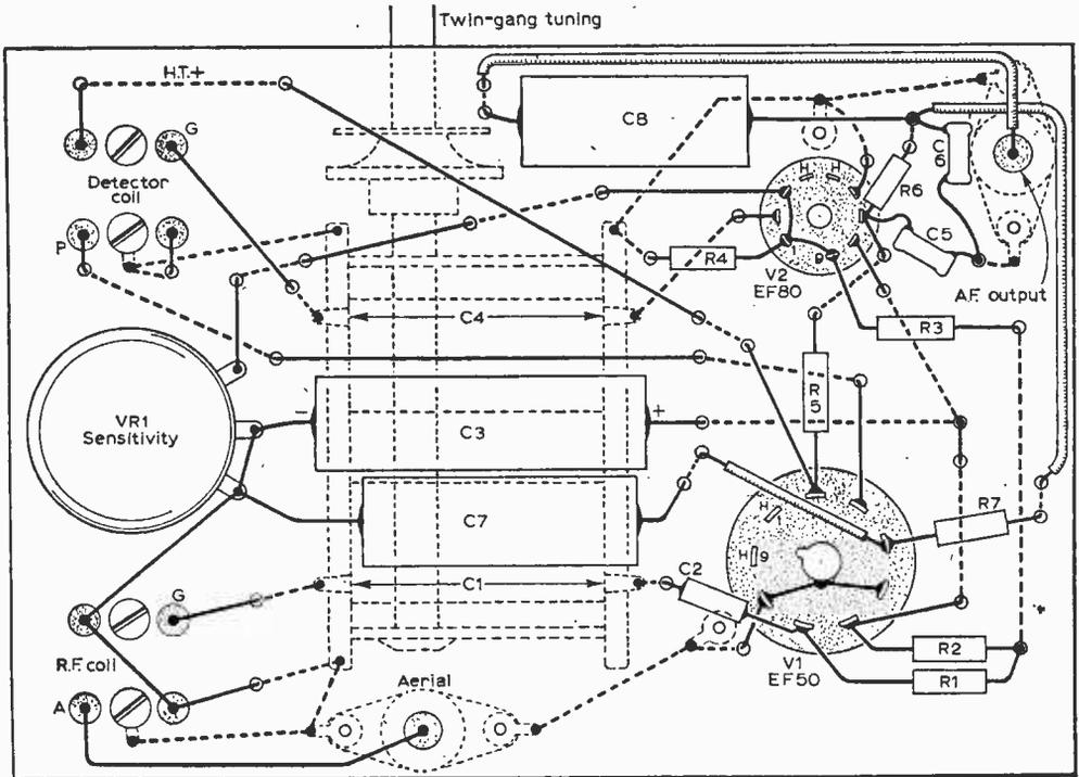
Fig. 2: Underside view of the "bread-board" wiring.
