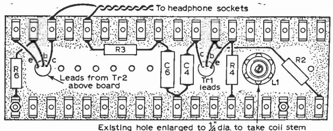
Fig. 6: The reverse side of the tag board.
