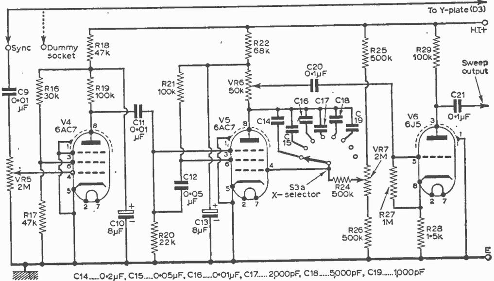
Fig. 10: Timebase generator, timebase and sync amplifiers.
