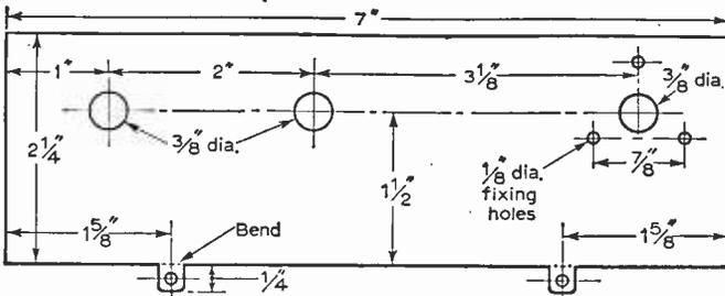
Fig. 4: Dimensions of the control support panel.
