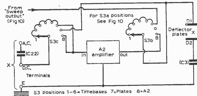
Fig. 13: Selector switching (with amplifiers): a (left); "X" (sweep) selector: b (below); "Y" selector.
