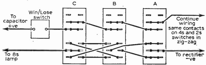
Fig. 7: The wiring of keys in 8s, 4s and 2s rows. The upper half of each key carries the relay control switch; the lower half controls the lamp in the D pile.
