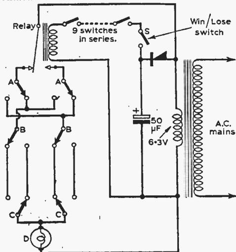
Fig. 3: The circuit of the bottom row of switches and power supply.
