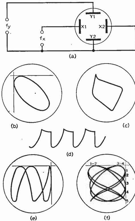
Fig. 12: Frequency comparison: (a) shows the basic connections; (b) ellipse formed when  $f_y = f_x$  — phase angle  $90^\circ$ ; (c) distorted trace of (b) when input is non-sinusoidal; (d) X-waveform producing (c); (e)  $f_y = 3f_x$ , waveform distorted; and (f)  $f_y : f_x = 4 : 5$ ; note superimposed loops.
