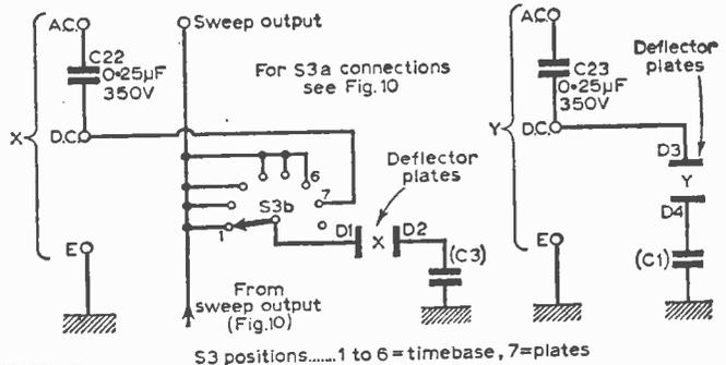
Fig. 11: Selector switching (without amplifier).
