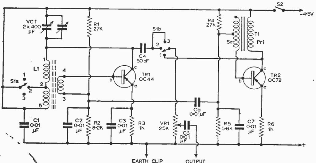
Fig. 1: The complete circuit of the generator.
