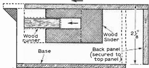
Fig. 4: How the top is slid into place along the runners and tops of the sides.
