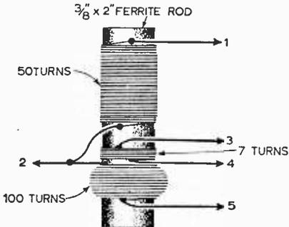
Fig. 2: Winding details of the tuning coil, L1.
