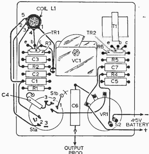
removing, to reach about 500kc/s on the l.w. band, with VC1 fully open.
