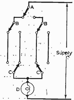
Fig. 2: The basic switching circuit.
