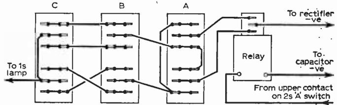
Fig. 8: Wiring the keys in 1s row.
