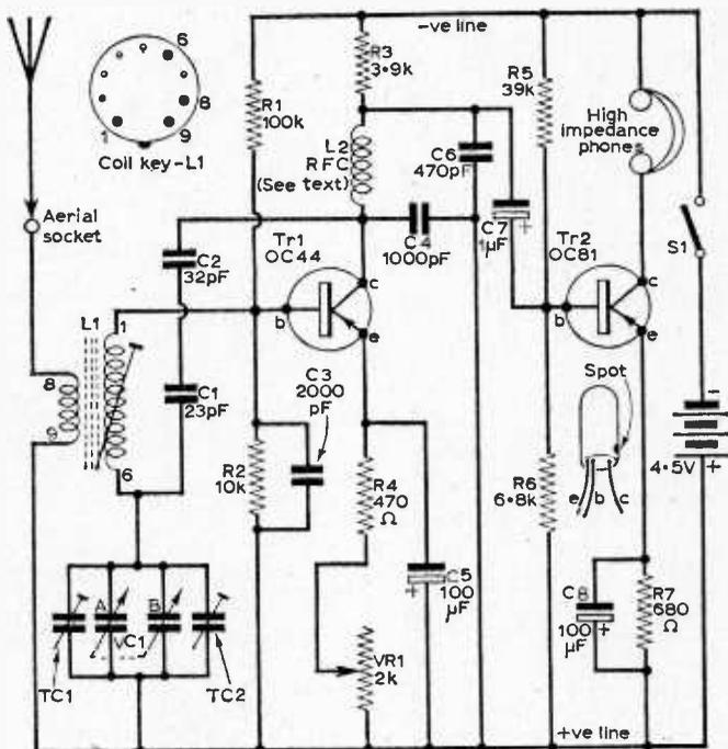
Fig. 1: The circuit.
