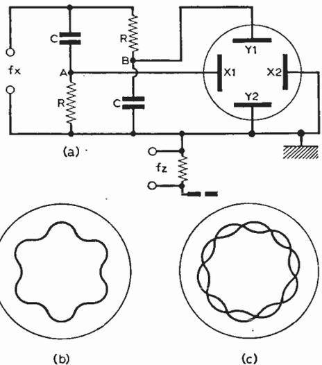
Fig. 13: Phase-splitting network for circular timebase; (b)  $f_z = 6f_x$ ; (c)  $f_z = 9/2f_x$  — double trace.
