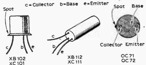
Fig. 2: Lead identification of types of transistors that can be used in this circuit.
