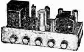
A 12 watt quality amplifier incorporating negative feedback, with a pre-amp for mic. and provision for mic./gram mixing. Frequency response  $\pm 1$  dB 15-20,000 c/s. Distortion only 0.15%, with noise and hum -50 dB. Separate Bass, Middle and Treble lift controls. Valve line-up: 6X7, 12AX7, 6L6, EL84 and EZ81. Push-pull output with matching to 3 or 15 $\Omega$ . Fully isolated power supply from 200/250 v. A.C. input, with take-off for tuner etc. Size 12 x 6 x 6 in. high.
