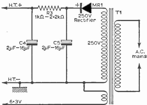
Fig. 4: The circuit of a suitable power supply.
