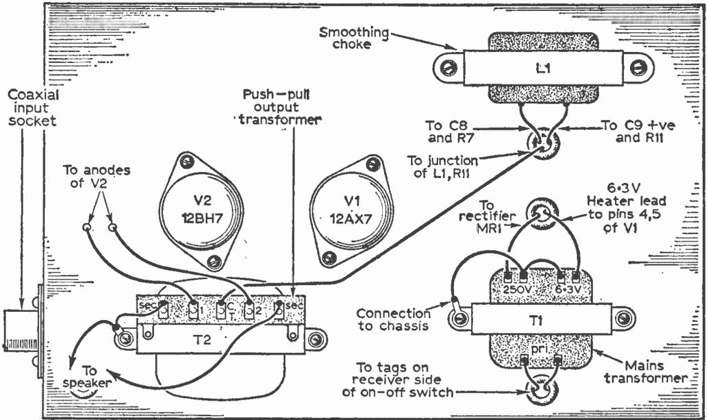
Fig. 2: The above-chassis layout of the amplifier
