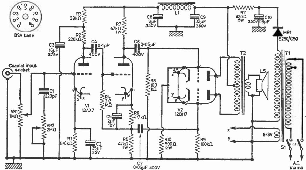
Fig. 1: The simple two-valve circuit.
