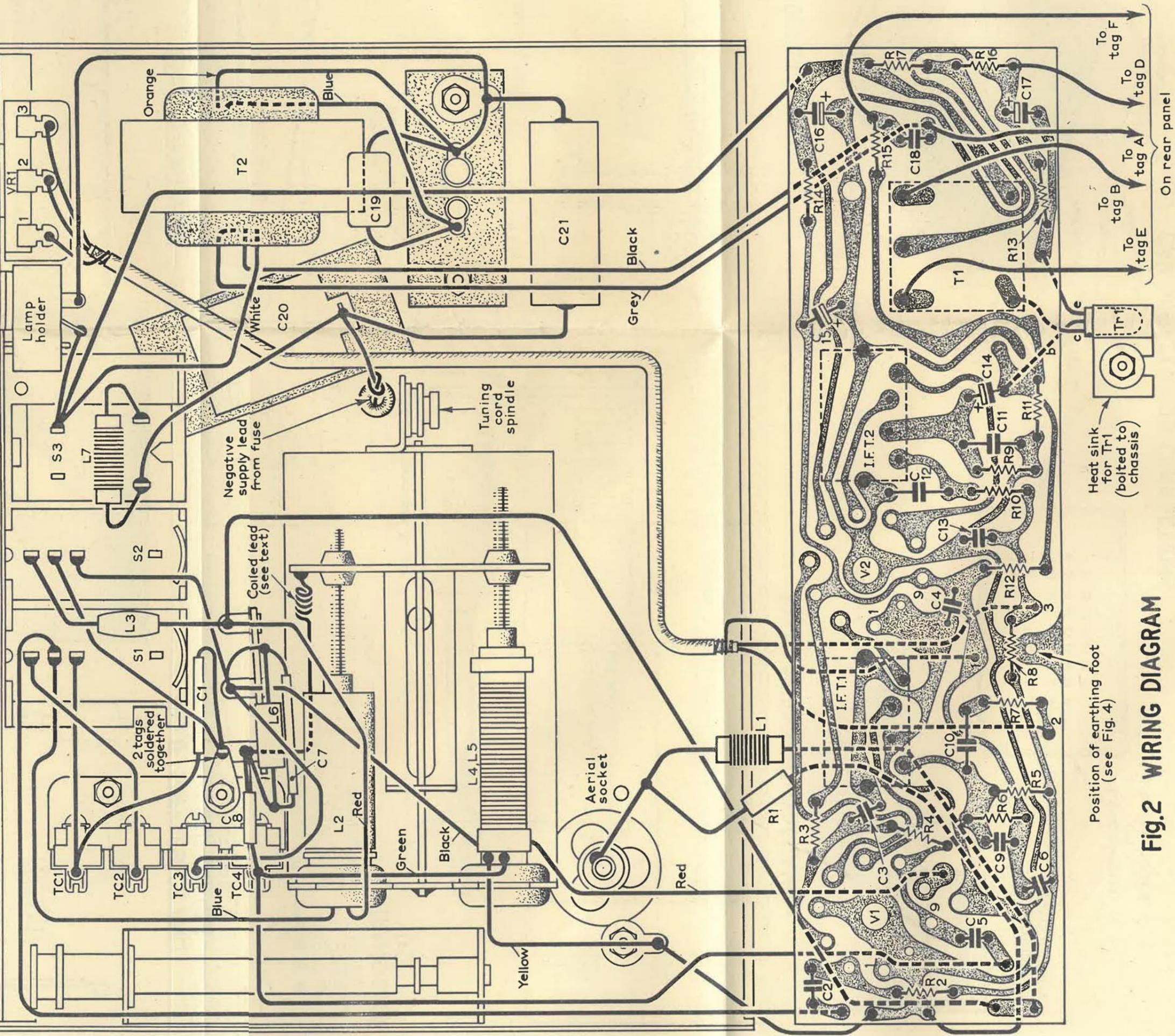
Fig.2 WIRING DIAGRAM
