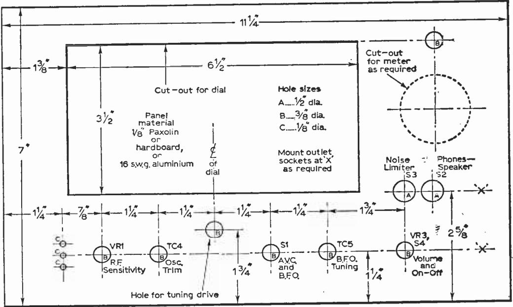
Fig. 7: Front panel control layout and dimensions.
