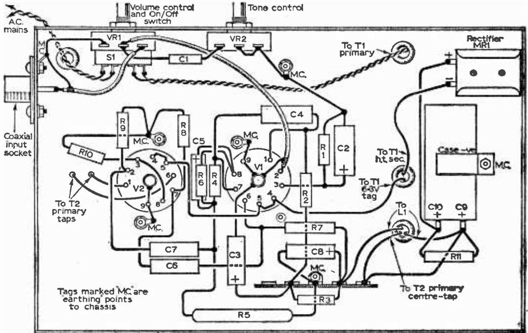
Fig. 3: The underchassis wiring diagram.
