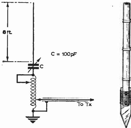
Fig. 2 (left): The theoretical set-up for the basic antenna. Fig. 3 (right): The element may be attached to a shaped piece of wood for simple erection in any convenient plot of ground.
