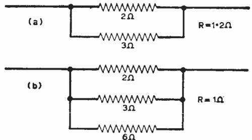
Fig. 6: Examples of resistances in parallel.
