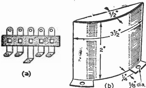
Fig. 6(a): The type of tag strip used in the construction of the “Ten-Five”; (b): details of the coil screen.
