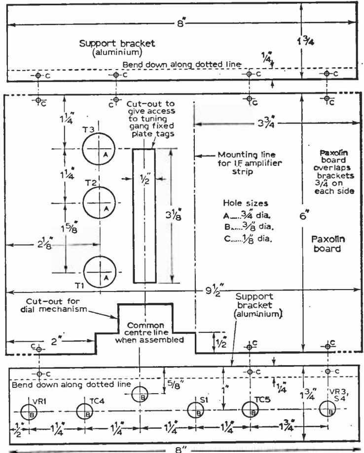
Fig. 4: Dimensions of the paxolin board and its aluminium supports.
