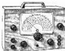
A precision signal generator of extremely high accuracy and quality. Six ranges from 120Kcs to 130Mc/s on fundamentals with calibrated harmonics from 130-300 Mc/s. 400 cps. INT. MOD. OR EXT. MOD. OUTPUTS MOD. RF. UNMOD. RF. or 400 c/s audio. R.F. output in excess of 100 mV. Large clear 5 inch dial. Handsome metal case with handle. Size 7 1/2 x 10 x 4 1/4 in. Complete with leads. Operation 220/240 volts A.C. Supplied brand new and guaranteed. £12-19.6. Carr. 5/-.
