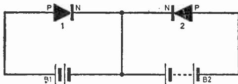
Fig. 12: Joining the two circuits of Fig. 11 produces the same current flow through each transistor, i.e. flows through diode 1 and only leakage current through diode 2.
