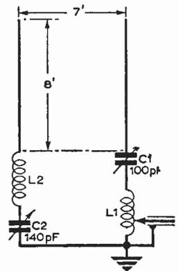
Fig. 4: The arrangement used in the setting-up procedure.
