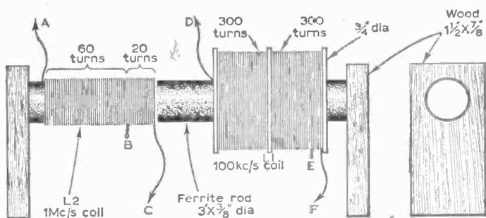
Fig. 2: Coil winding details for L1 and L2.
