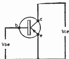
Fig. 15: A p-n-p transistor in common emitter connection.
