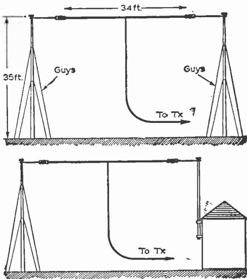
Fig. 1: Two variations on the aerial apparently necessary for efficient reception on 20m.
