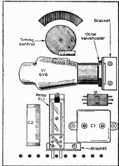
Fig. 7: A suitable layout of components for the timer.
