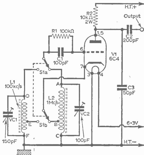
Fig. 1: The simple, single-valve circuit.
