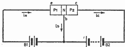
Fig. 13: When the n-type material is made extremely thin, current flows through both junctions.
