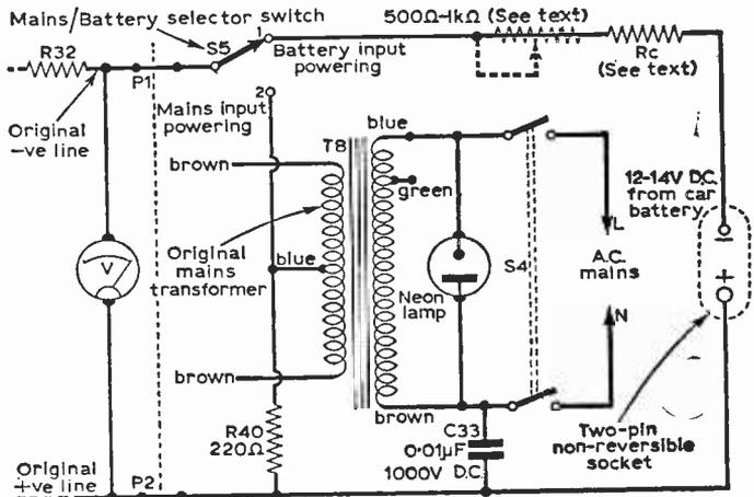
Fig. 8: Modifications for mains/battery operation. See page 661.
