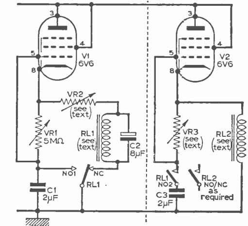
Fig. 8: Using two timer circuits in cascade to provide long timing periods.
