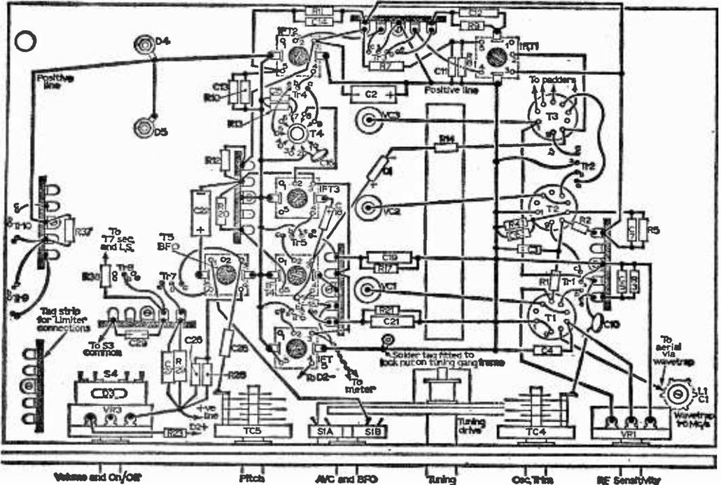
Fig. 5: An underside view showing most of the wiring. Note positive bar and orientation of i.f.t.'s.
