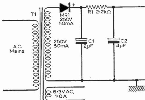
Fig. 5: A power pack for the timer.
