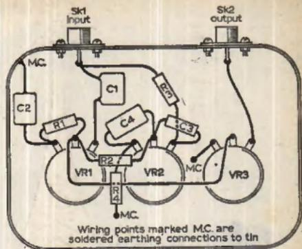
Fig. 6: Tone control wiring and component layout.
