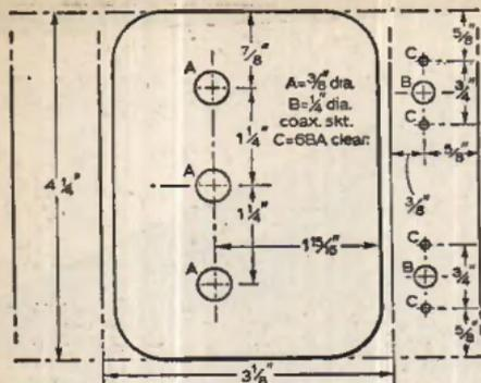
Fig. 5: Tone control chassis drilling details.
