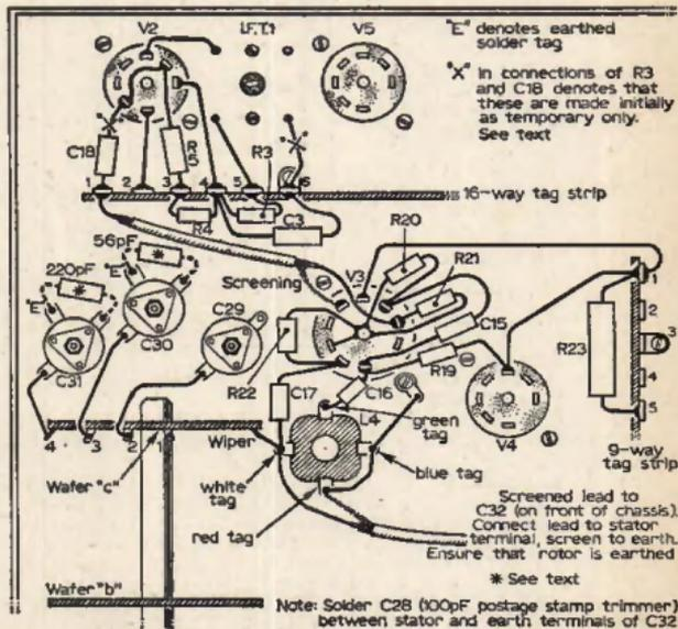
Fig. 8: Wiring and layout for stage 4 of construction.
