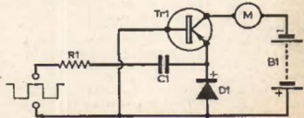
Fig. 1: Circuit of the basic frequency discriminator.
