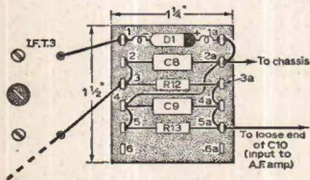
Fig. 10: Wiring and layout of detector/filter.
