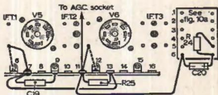
Fig. 11: A.G.C. wiring.
