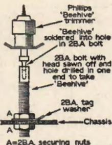
Fig. 7: Method of mounting the beehive trimmers.
