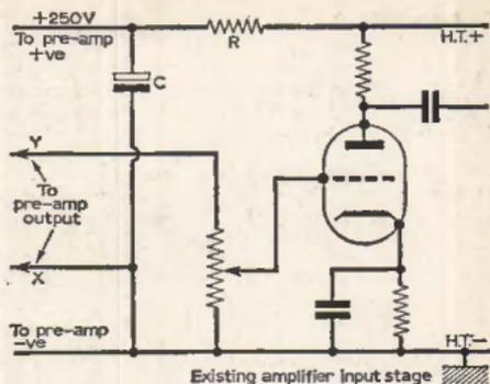
Fig. 2: The arrangement of a valve amplifier input stage for connection of the preamp. R has a value to regulate the amplifier h.t. to 250V for the preamp. C = 8 $\mu$ F 350V.
