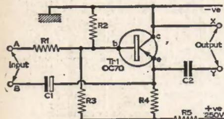
Fig. 1: The single-transistor circuit of the unit.
