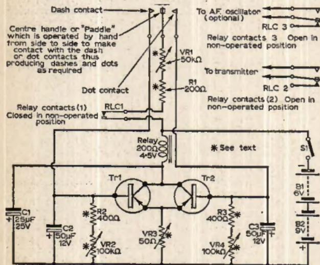
Fig. 1: Circuit diagram of transistorised key.
