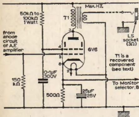
Fig. 4: Output stage, showing monitor point.
