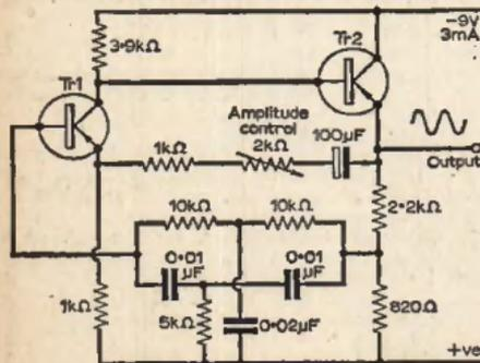
Fig. 6: Parallel-T -ve feedback oscillator.
