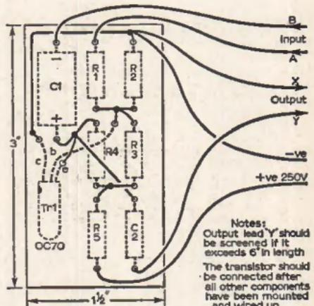
Fig. 3: Construction of the unit is on a piece of paxolin and the above layout was used successfully by the author.
