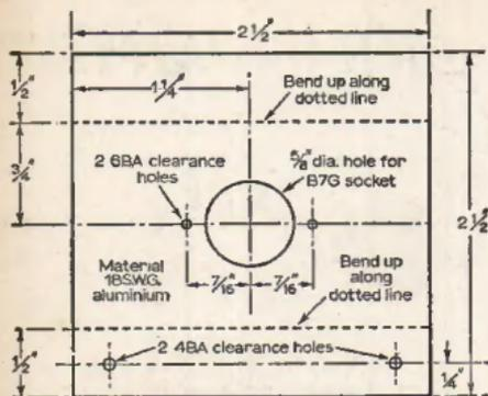
Fig. 2a: Drilling and bending details of valveholder bracket.
