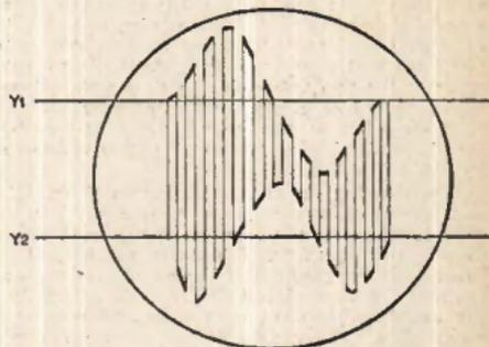
Fig. 2: The effect of a slow gating speed. The Y1-Y2 waveforms are composed of positive and negative peaks of the gating waveform.
