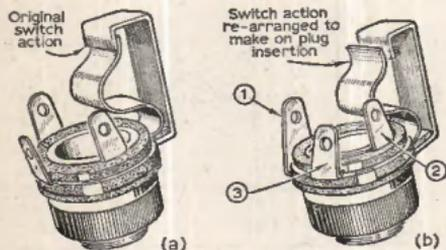
Fig. 2: Modifications for the phone socket.
