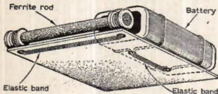
Fig. 5: Method of connecting battery and ferrite rod.
