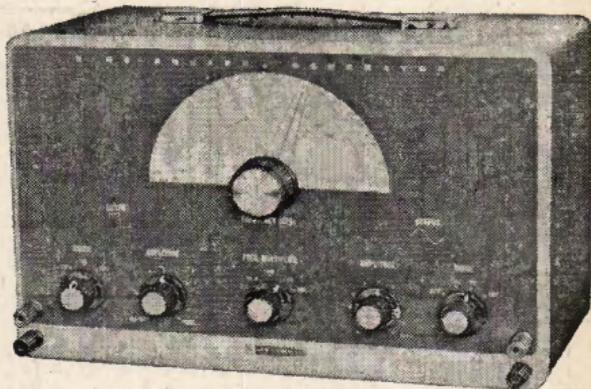
From Heathkit comes the 1G-82U sine-square wave generator which has a frequency range of 20c/s to 1Mc/s in 5 bands. Sine and square wave outputs are available separately or simultaneously and there is less than 0.15 $\mu$ Sec. rise time on square wave and less than 0.5% distortion on sine wave. Separate output terminals and attenuators permit individual control. In kit form, the price is £24 10s. and assembled and tested £36 10s.
