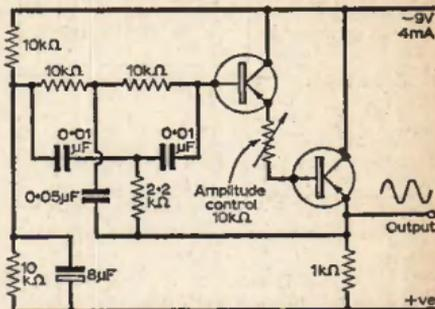
Fig. 7: Parallel-T +ve feedback oscillator.
