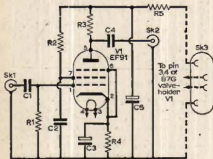
Fig. 1: The circuit diagram of the preamplifier.
