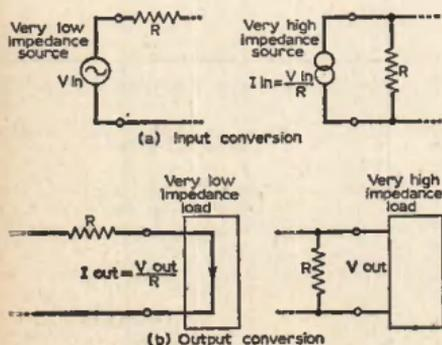
Fig. 1: Alternative arrangements at end of network where there is a resistance.
