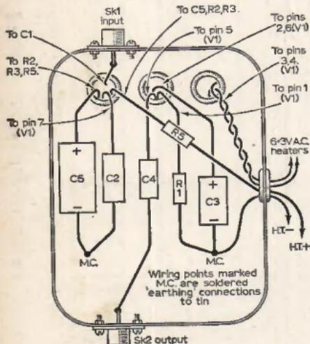
Fig. 3: Preamplifier component layout and wiring.
