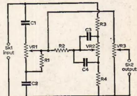
Fig. 4: Circuit diagram of tone control network.
