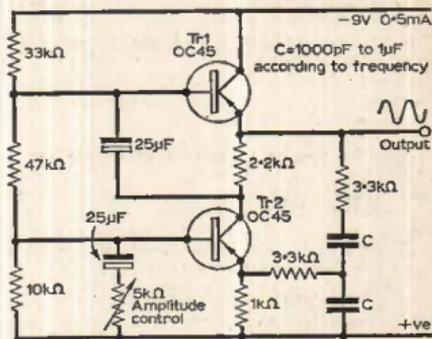
Fig. 5: Oscillator with modified Wien network.
