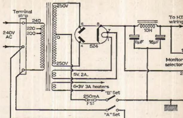
Fig. 5: Power supply circuit, showing monitor points and h.t. control.
