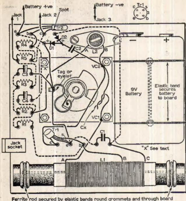
Fig. 4: Component layout and wiring details.
