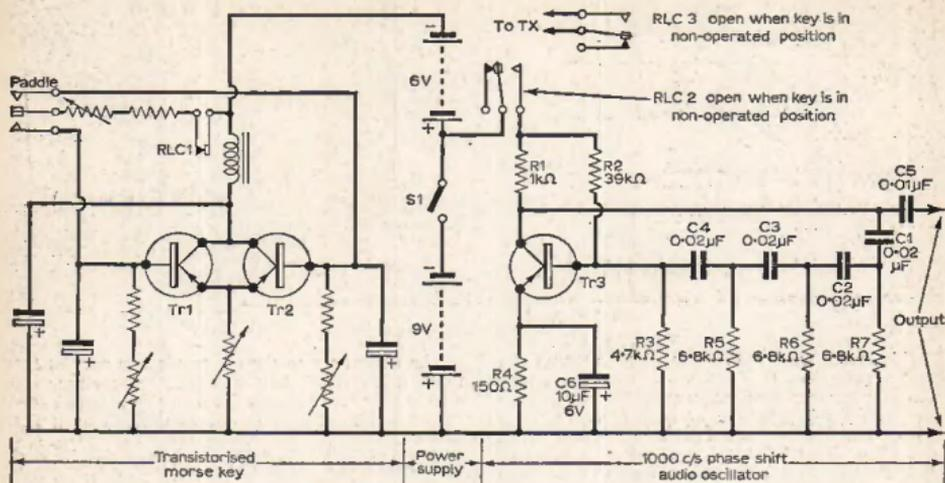
Fig. 2: Diagram of electronic key and phase-shift audio oscillator.
