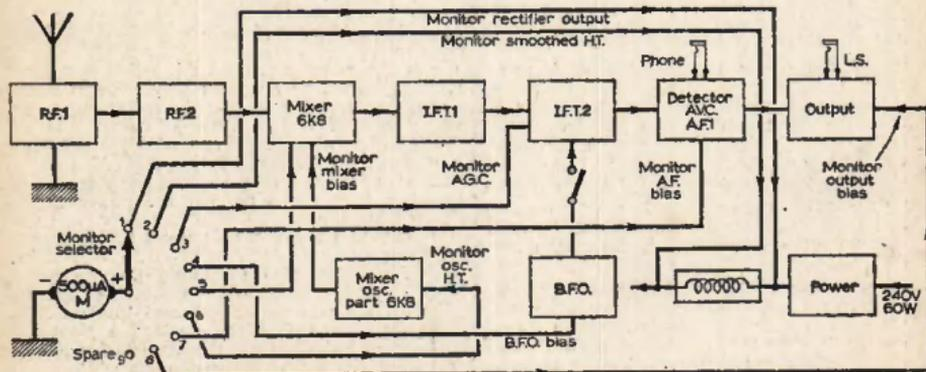
Fig. 6: Monitoring system in modified W.S.19 receiver.
