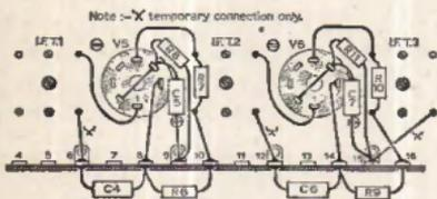
Fig. 9: Wiring and layout for stage 5 of construction
