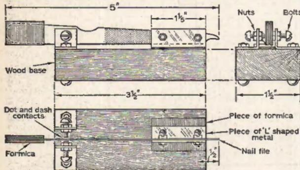
Fig. 3: Complete "paddle" for the key.
