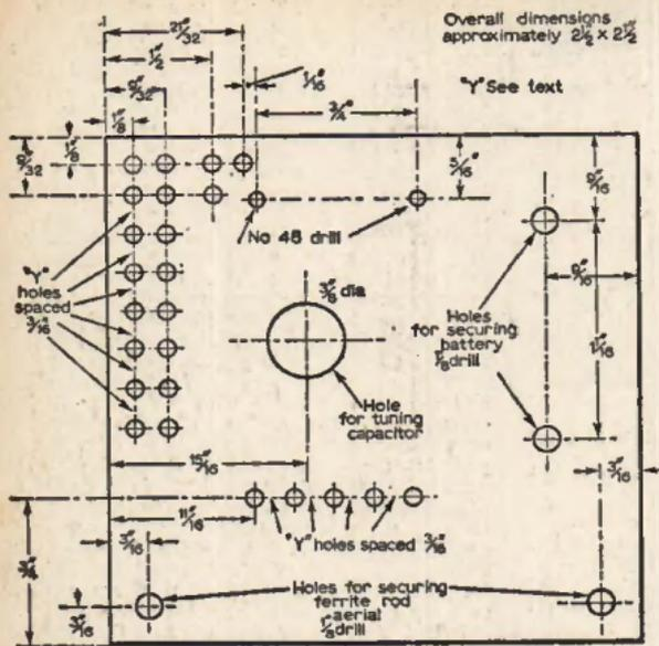
Fig. 3: Drilling details for the panel.
