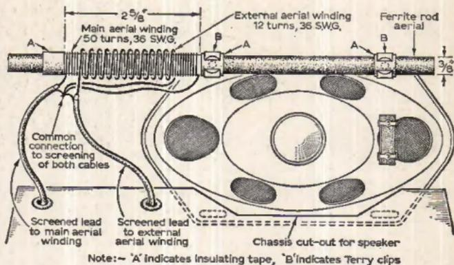
Fig. 5: (above) Aerial winding and mounting details
