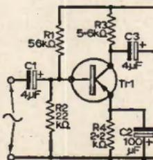
Fig. 6: Circuit of common-emitter amplifier for increasing the sensitivity of the instrument, as described in the text.
