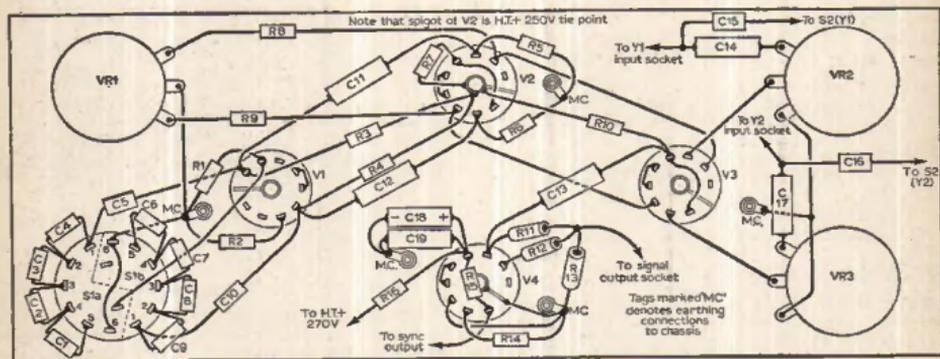
Fig. 4: Chassis wiring. The centre spigot of V2 is used as an h.t.+ point.
