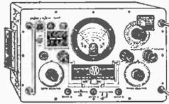
High quality 97 range instrument which measures A.C. and D.C. Voltage, Current, Resistance and Power Output. Ranges D.C. volts 250V-10,000V. (10 megΩ-110 megΩ input). D.C. current 10μA-25 amps. Ohms: 0-1,000 megΩ. A.C. volt 100 mV-250V. (with R.F. measuring head up to 250 Mc/s). A.C. current 10μA-25 amps. Power output 50 micro-watts-5 watts. Operation 0/110/200/250V. A.C. Supplied in perfect condition complete with circuit lead and R.F. probe. £25. Carr. 15/-.
