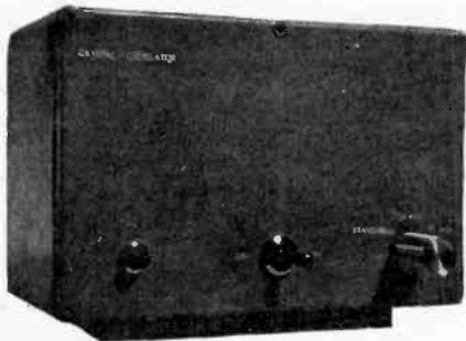
This unit provides frequency marker points at every 100Kc/s up to 32Mc/s.
