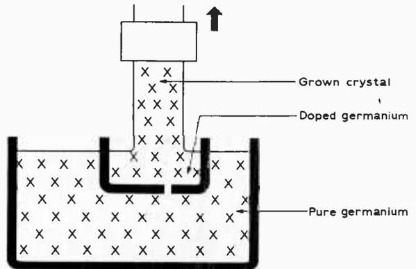
Fig. 5: The double-crucible method of growing doped crystals.
