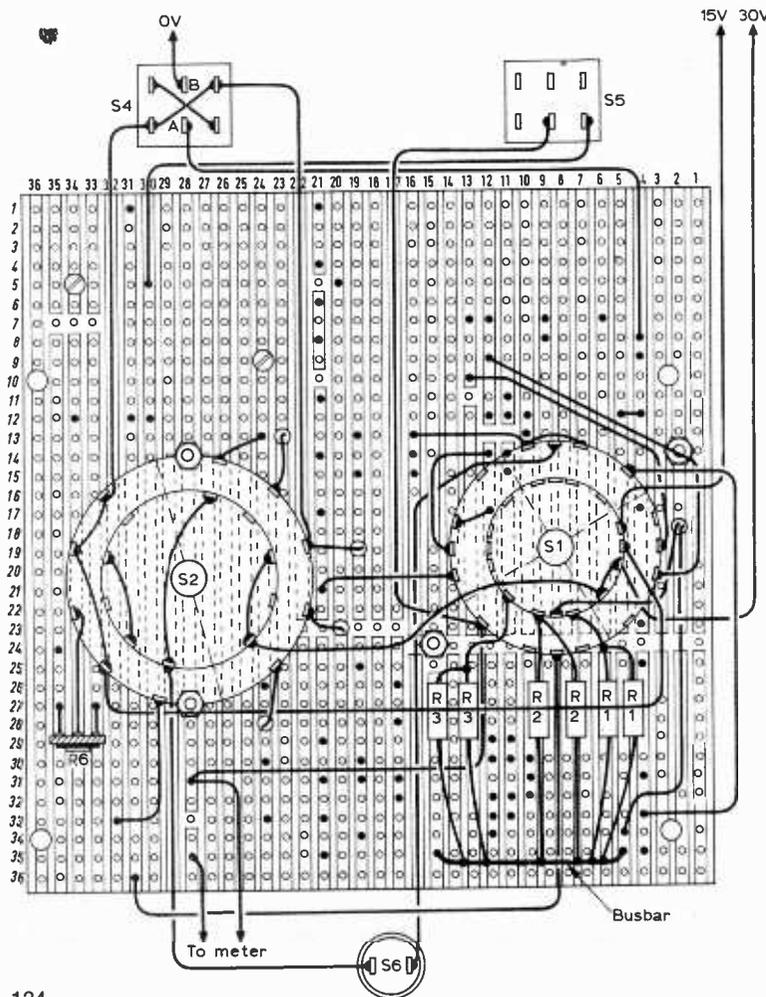
Fig. 2 (left): The copper side of the Veroboard showing the switch connections and the breaks in the laminate. Note that S6 was incorrectly labelled R5 in the circuit last month.
