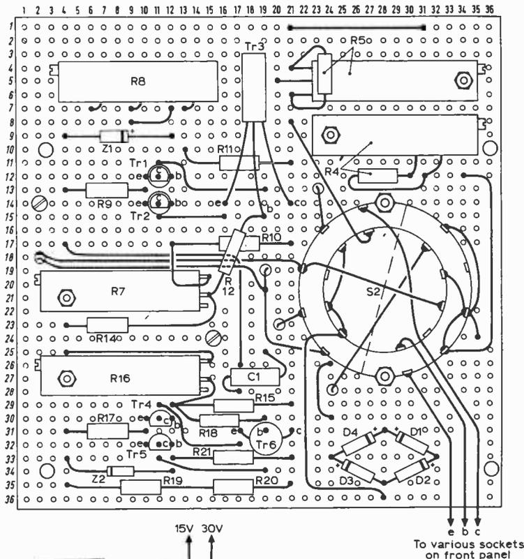
Fig. 1 (above): The location of the main components.
