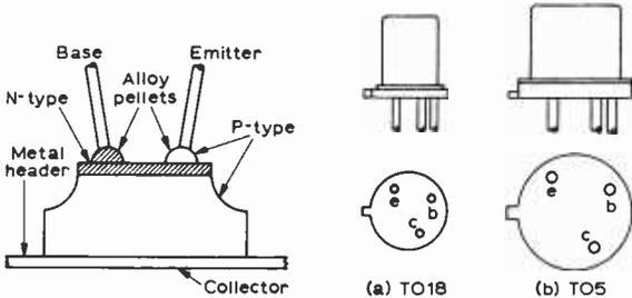
Fig. 1: Mesa transistor construction.
