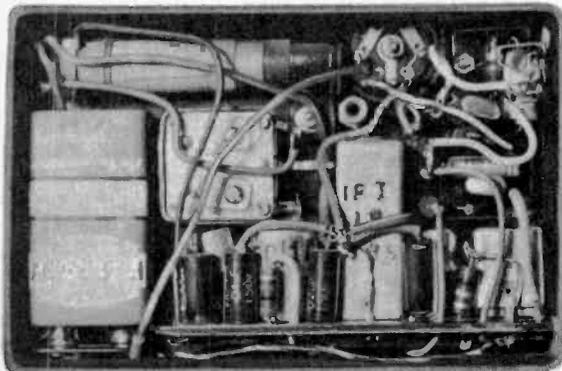
**P**OCKET receivers often use reflexed t.r.f. circuits, and although these can give good results, some constructors may prefer a superhet. The one described here is built with standard and readily available transistor type components, and is approximately  $4\frac{3}{8} \times 2\frac{7}{8} \times 1$  in. external dimensions, including battery. It is a 4-transistor superhet circuit giving excellent head-phone results.
