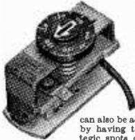
From thermal runaway or overheating. Thyristors, rectifiers, transistors, etc., which use heat-sinks can easily be protected; simply make the contact thermostat part of the heat-sink. Motors and equipment generally, can also be adequately protected by having thermostats in strategic spots on the casing. Our contact thermostat has a calibrated dial for setting between 90°-190°F. or with the dial removed range setting is between 80 to 800°F. Price 10/-.
