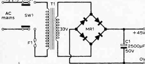
Fig. 3: The circuit of the power supply.
