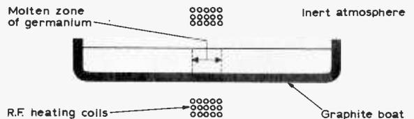
Fig. 2: Zone refining apparatus.
