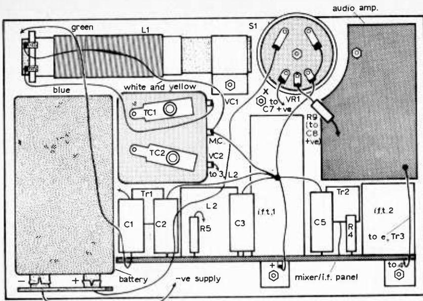
Fig. 2: General layout and inter-module wiring.
