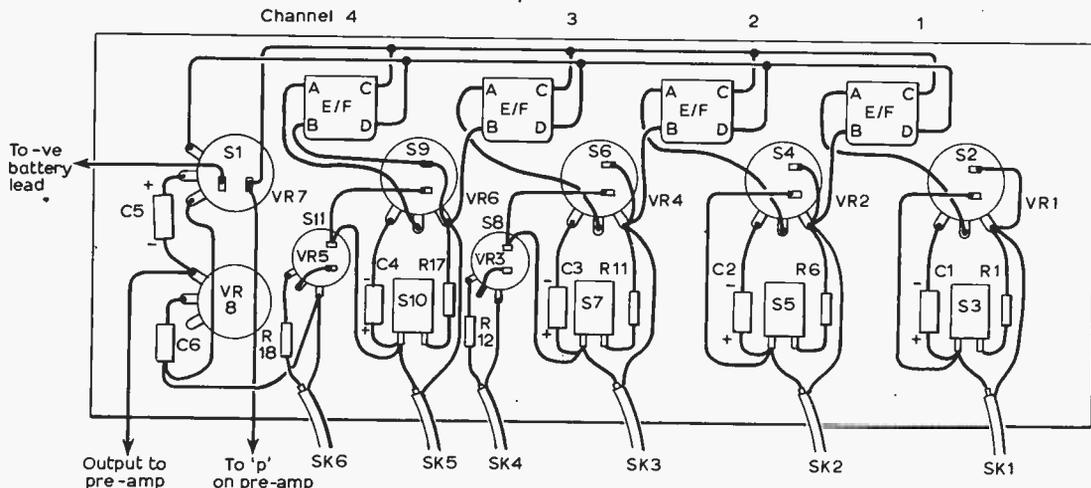
Fig. 7: Wiring of the main panel.
