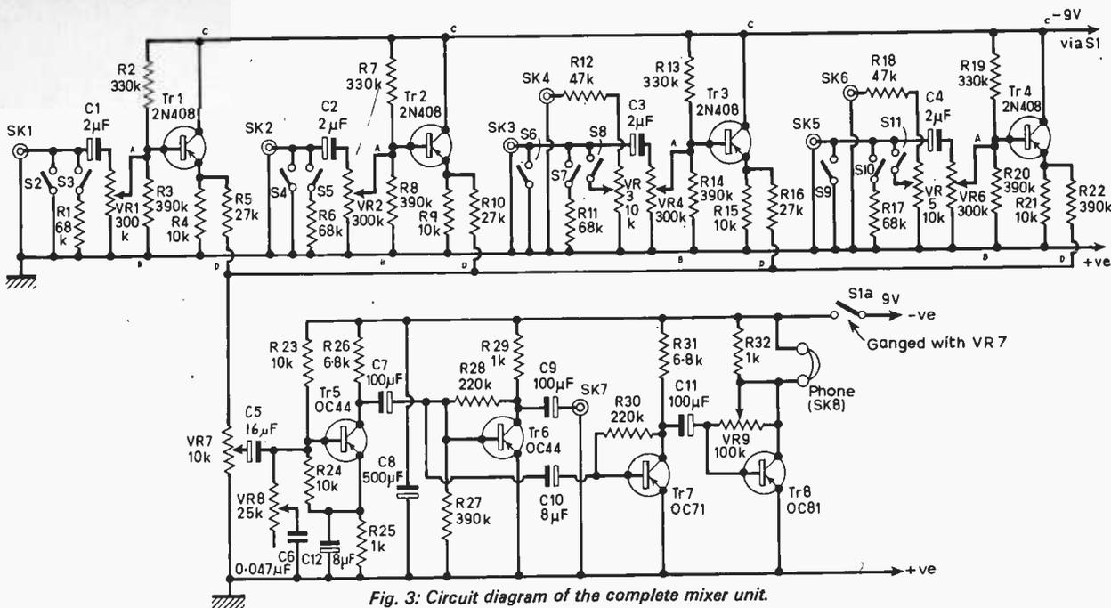
Fig. 3: Circuit diagram of the complete mixer unit.
