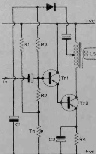
Fig. 3: A sliding bias amplifier. The current fed back by the rectifier must exceed the input signal current, and C1 must be chosen so that there is not too much time-lag between the signal and bias. Too small a value of C will cause severe distortion of low frequencies.
