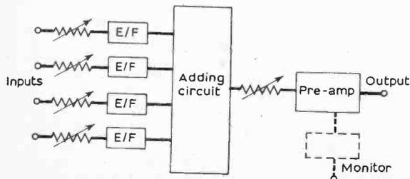
Fig. 1: Block diagram of an active mixer.
