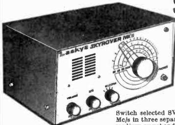
A completely new short wave receiver exclusive to Lasky's, at a real economy price. Four valve line up using one each 6BE6, 6BA6, 6AV6 and 6AR5 valves, gives highly sensitive reception and powerful gain.
