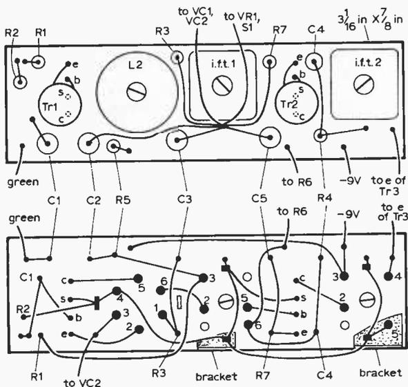
Fig. 3: The r.f. and i.f. amplifier component board.
