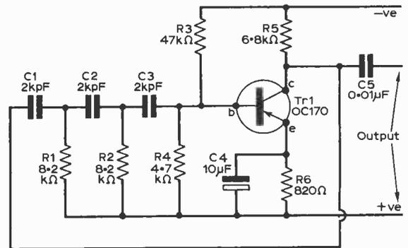
Fig. 1: The circuit of the phase shift oscillator. The voltage is 9v, supplied by any battery.
