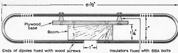
Fig. 3.4: The folded dipole.
