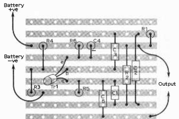
Fig. 2: The component layout; there are no breaks in the Veroboard copper strip.
