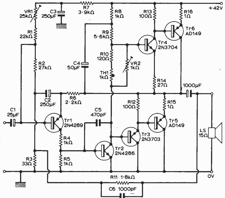
Fig. 1: The circuit of the power amplifier.
