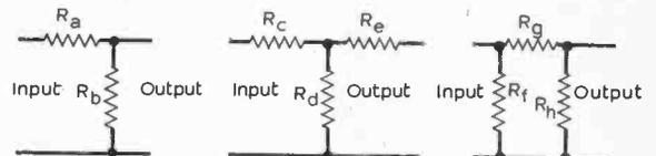
Fig. 2: Three types of resistive attenuator—L, T and  $\pi$ .
