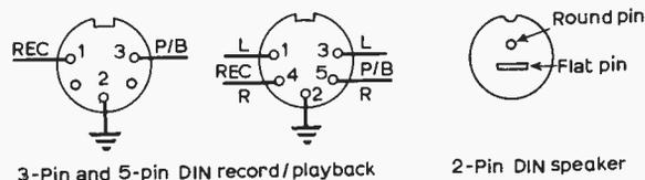
Fig. 4: Pin connections for 2, 3 and 5-pin DIN plugs.
