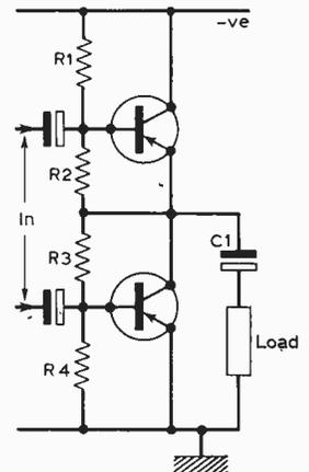
Fig. 6: A single-ended push-pull or totem-pole amplifier.
