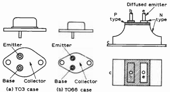
Fig. 3: Power transistor encapsulations.
