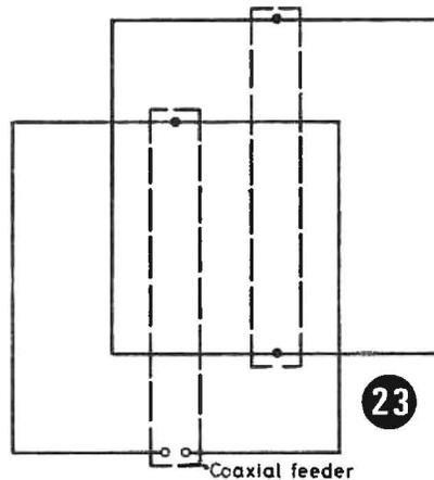
Mount each element on small insulators on vertical pieces of wood, shown dotted. Use another piece of wood as a boom to fix the elements 450mm (18in) apart.
