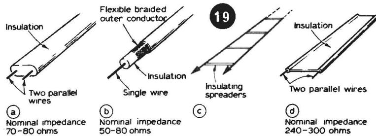
The wire used for these SW aerials should be copper, preferably enamelled or plastic-covered. The gauge may be as small as 22SWG for short spans of a few metres with heavier gauges up to 16 or 14SWG for longer lengths. All joints must be soldered and then waterproofed thoroughly.
