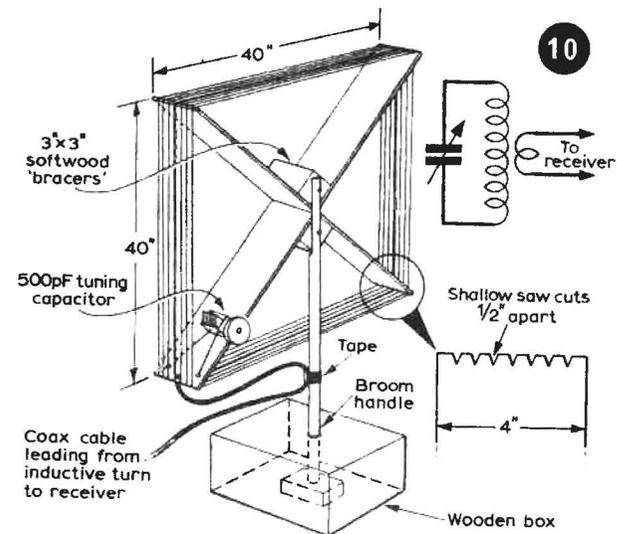
Seven turns of wire are wound round the frame and connected across the tuning capacitor. A single insulated turn of wire is wound over the fourth turn of the main winding and connected to the coaxial cable going to the receiver.
