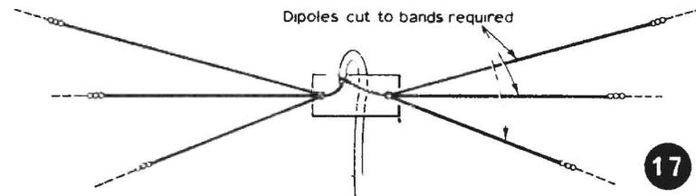
assembly. The directivity of this aerial is the same as the half-wave dipole.
