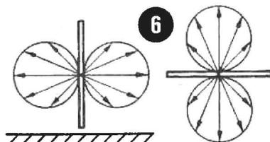
Left, A vertical Hertz aerial is also omnidirectional. The plan view of the horizontal Hertz aerial, right, shows maximum radiation at right angles to the line of the aerial.
