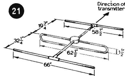
dipole by about four times, restored by the transformer action of the folded dipole.
