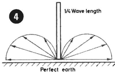
The Marconi aerial radiates equally well in all directions round the aerial, i.e. it is omnidirectional.
