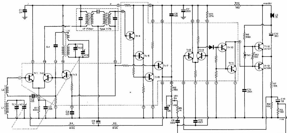
Fig. 1: A practical circuit for a m.w. radio using the TAD100 and an i.f. filter type 1175. The thermistor and C11 junction should be shown connected to the base of Tr13.
