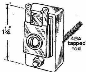
This padder can be omitted if the correct value of 175pF is available. Difficulty was experienced in obtaining this exact value so a 250pF variable was used, but adjustment of long-wave section was found to be very tricky.
