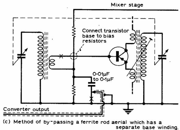
(c) Method of by-passing a ferrite rod aerial which has a separate base winding.
