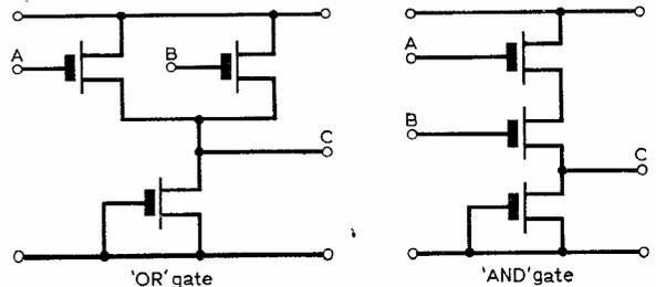
Fig. 5: MOST logic gates.
