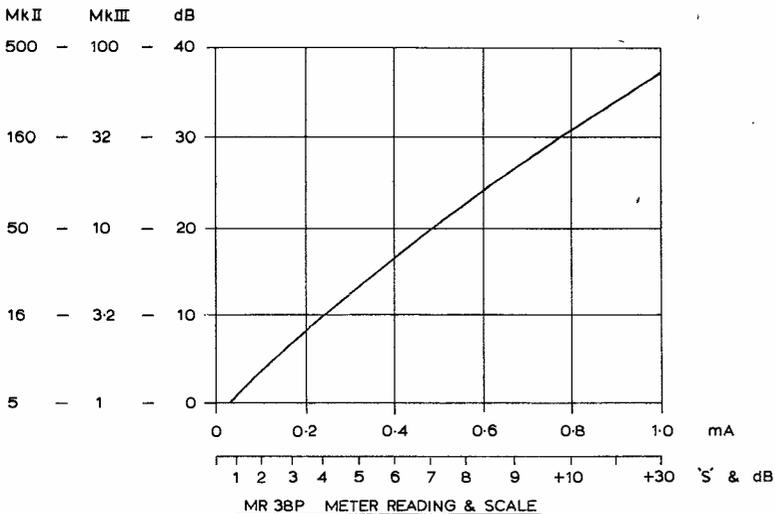
Fig. 45: Graph showing input signal/'S' meter readings for Mk. II and Mk. III Clubman.
