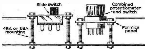
Fig. 4: Details of the sub panels, control mountings, chassis feet and l.w. trimmer capacitor support. Tag panel A is shown on the left, panel B on the right.
