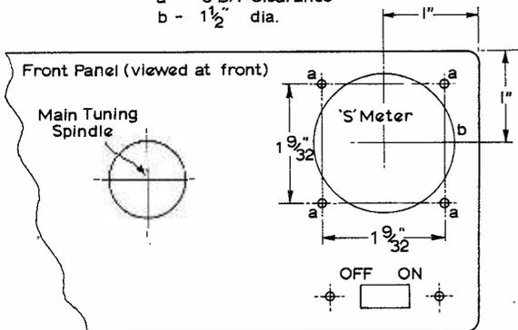
Fig. 46: Front panel drilling for the 'S' meter.
