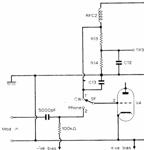
Fig. 3: Suggested modification to permit clamp type modulation.
