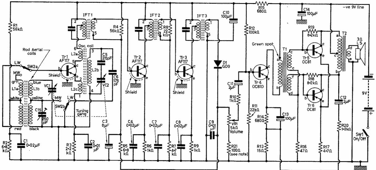
Fig. 1: The complete circuit of the six transistor two waveband Chelmer Six.
