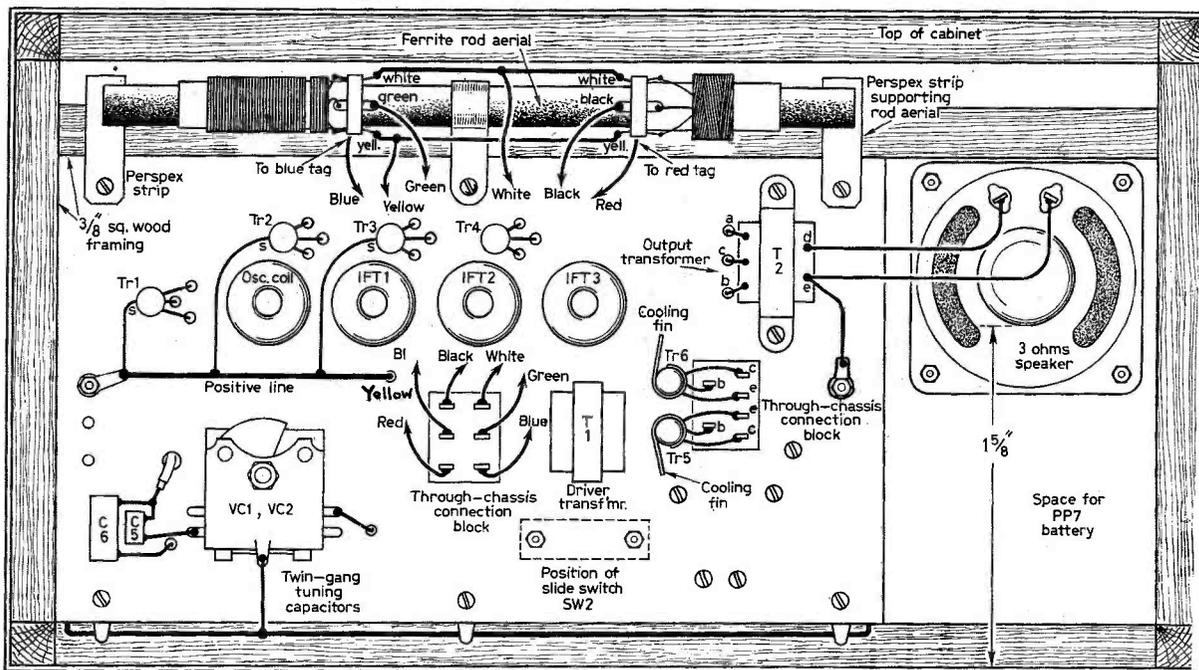
Fig. 5: (above) The component layout viewed from the rear of the case, the drilling plan is shown in Fig. 2.
