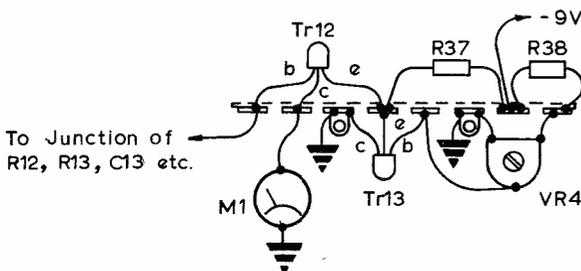
Fig. 47: Component layout and wiring for the 'S' meter circuitry.
