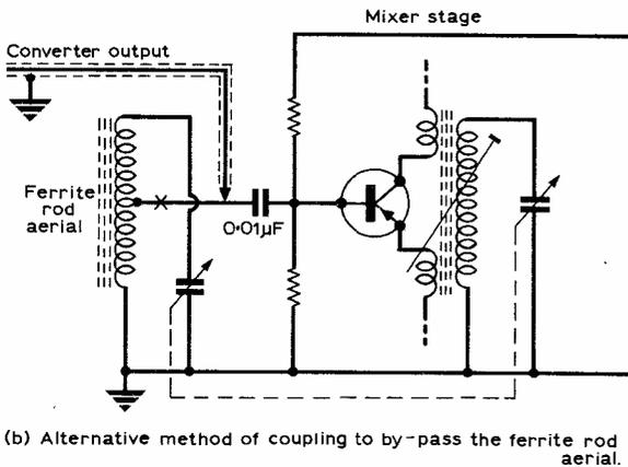
(b) Alternative method of coupling to by-pass the ferrite rod aerial.
