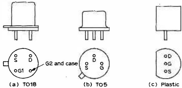
Fig. 18: F.E.T. encapsulations.
