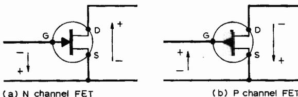
Fig. 13: B.S. preferred symbols and applied polarities for junction F.E.T.'s.
