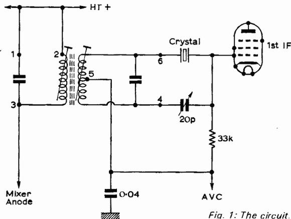
Fig. 1: The circuit.
