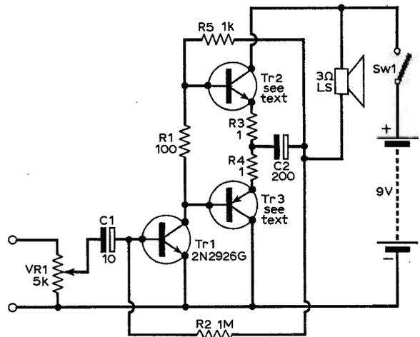
Fig. 1: The circuit diagram of the Take 20 amplifier.
