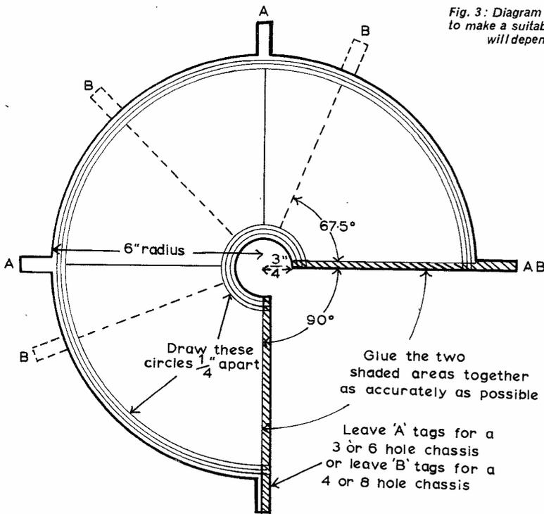
inside of the chassis level with the rim. The outer diameter can be trimmed to size by cutting all round one of the lines that you draw. The inner diameter should be made a snug fit around the outside of the voice coil former, again by trimming all round inside the template, using the lines as a guide. Then mark the template to indicate the degree of overlap required to get the correct angle.
