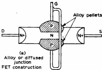
Fig. 16a: Alloy or diffused junction F.E.T. construction.
