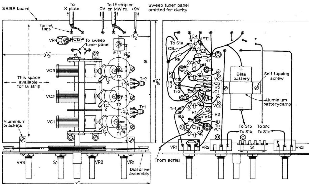
Fig. 6: The layout and wiring diagram.
