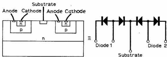
Fig. 2: Integrated circuit isolation achieved by means of back-to-back diodes.
