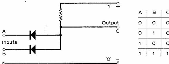
Fig. 4: Simple diode-resistor logical AND gate with corresponding truth table.
