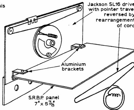
(b) Method of mounting "sweep" tuner panel on top of tuning capacitor
