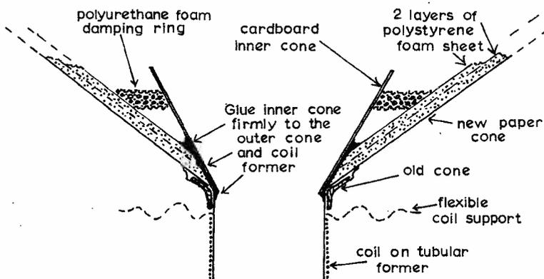
Fig. 7: Diagram showing the fitting of the h.f. radiator cone to the large cone and the siting of a damping ring of polyurethane foam.
