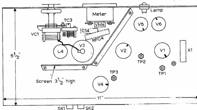
Fig. 2: The above-chassis layout.
