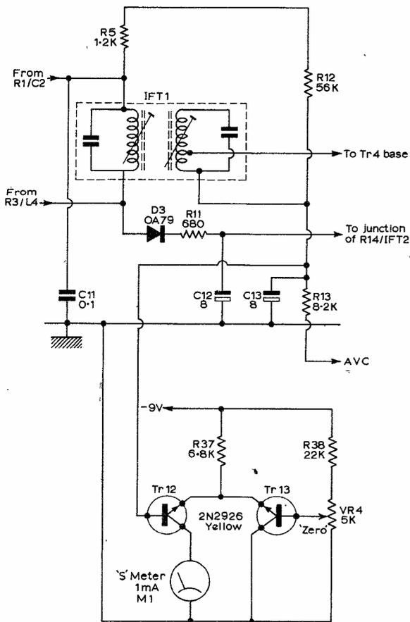
Fig. 44: 'S' meter circuitry as fitted to the Clubman Mk. II receiver.
