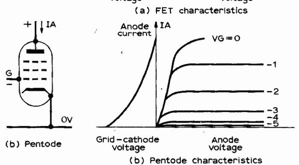
Fig. 14: (left) Comparison of F.E.T. and pentode symbols. Fig. 15: (right) Comparison of F.E.T. and pentode characteristics.
