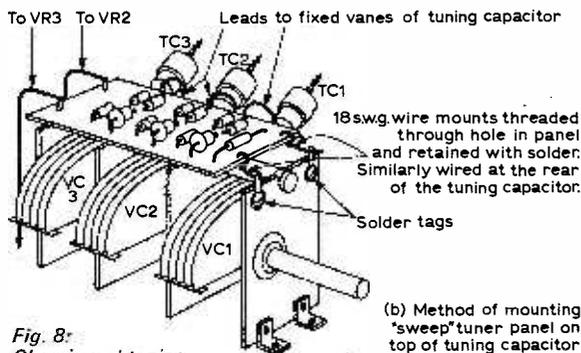
Fig. 8: Chassis and tuning constructional details.
