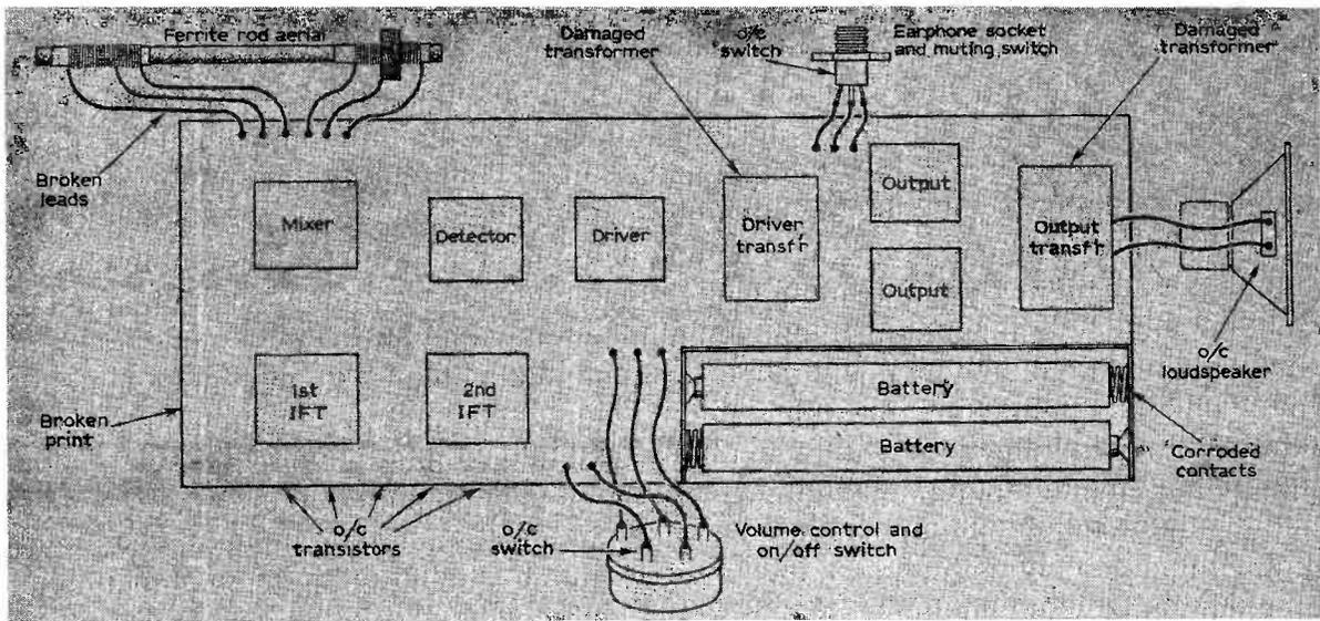
Fig. 1: The most common faults in a normal a.m. transistor radio.
