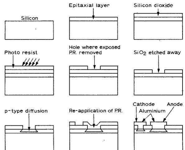
Fig. 1: Planar technology: the stages involved in the manufacture of an epitaxial planar diode.
