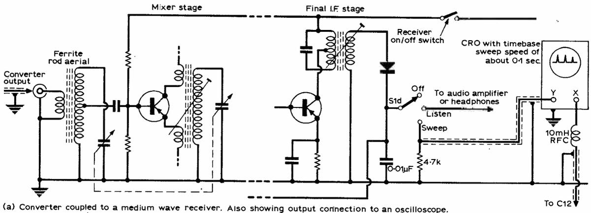
(a) Converter coupled to a medium wave receiver. Also showing output connection to an oscilloscope.
