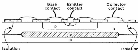
Fig. 3: Construction of an integrated circuit planar epitaxial transistor.
