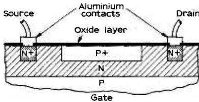
Fig. 16b: Planar junction F.E.T. construction.
