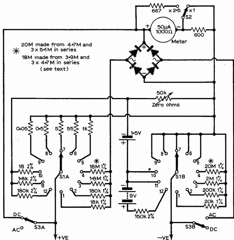
Fig. 1: The complete circuit of the Microtest.
