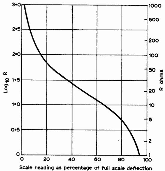
Fig. 2: Resistance measurements can be calculated from a graph stuck on the bottom of the case.
