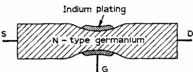
Fig. 17: Tectron construction.
