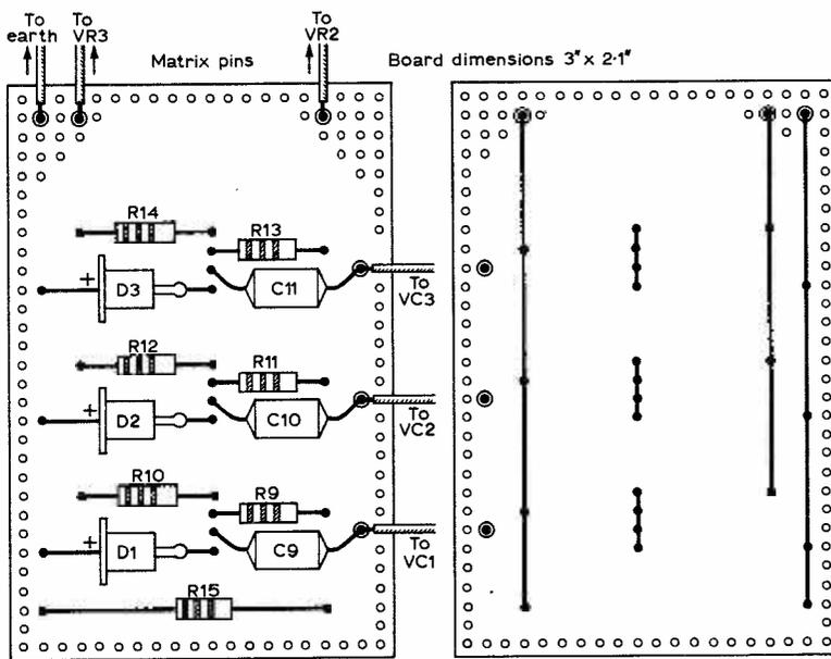
Fig. 7: The component layout and wiring of the sweep tuner panel.
