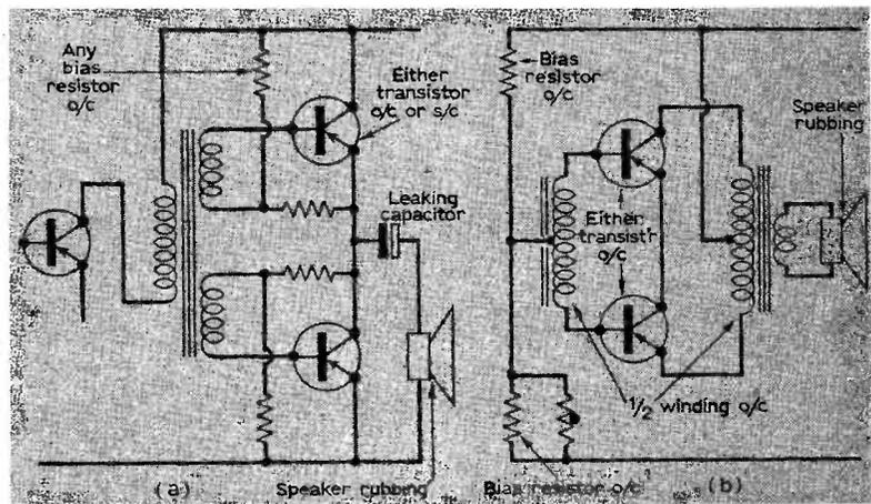
Fig. 2: Faults associated with the two commonest output stages.
