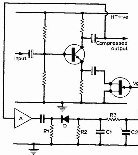
Fig. 5: The compressor circuit principle.
