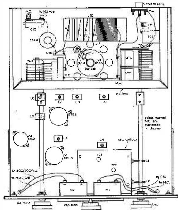
Fig. 2: Plan view of transmitter chassis.
