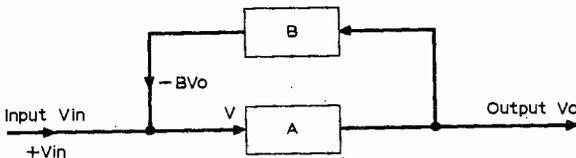
Fig. 5.1. Basic circuit of a feedback network
