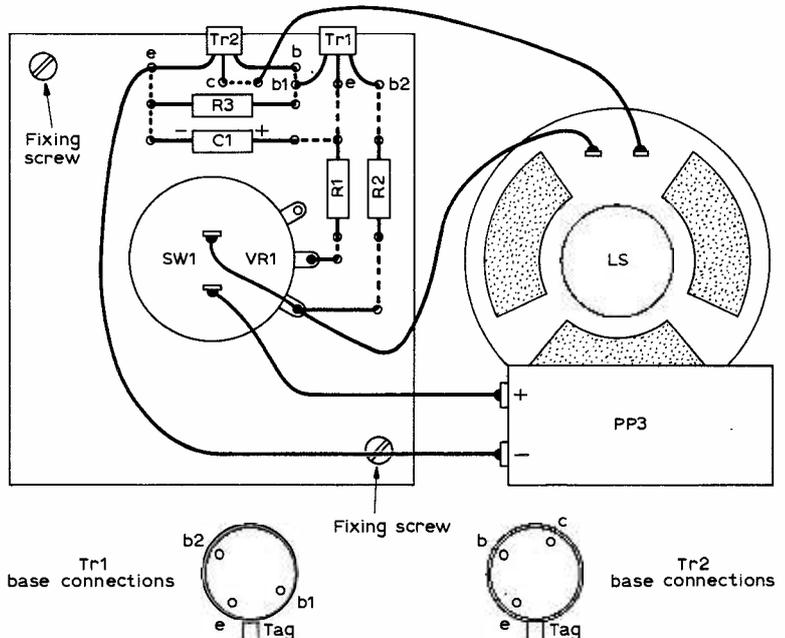
Fig. 2: The component layout and transistor base connections
