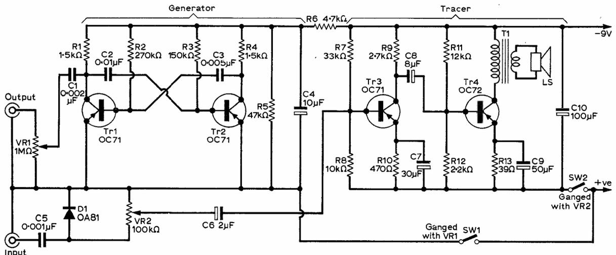
Fig. 1 : Circuit of the Genetracer. The "generator" and the "tracer" are built on separate circuit boards
