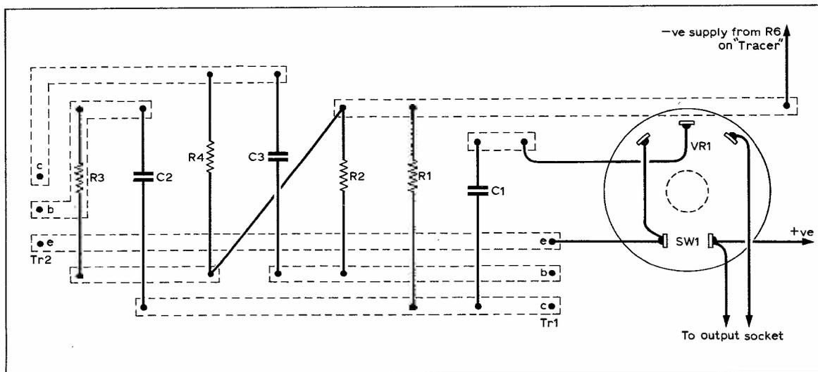
Fig. 2 : Full scale layout of the "generator" circuit board
