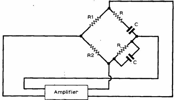
Fig. 5.5. Basic circuit of the Wien bridge oscillator
