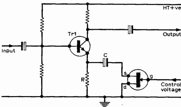
Fig. 4: The basic control circuit used in the final circuit.
