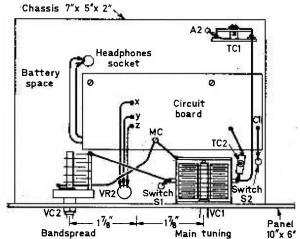
Fig. 4 : Top view of chassis and circuit board.
