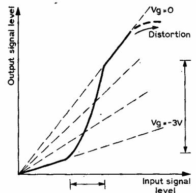
Fig. 8: (left) Expansion circuit principle. Fig. 9: (above) The arrows on the graph show how a small range of volume in the input is expanded to a wider range.
