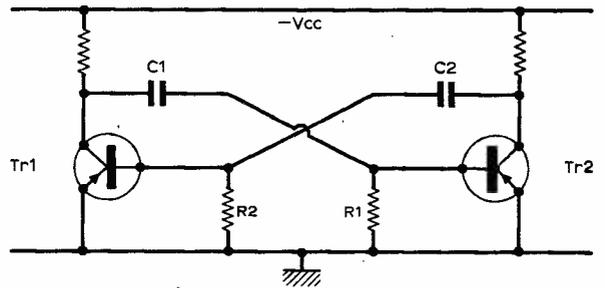
Fig. 5.6. Relaxation oscillator using two feedback networks C1R1 and C2R2
