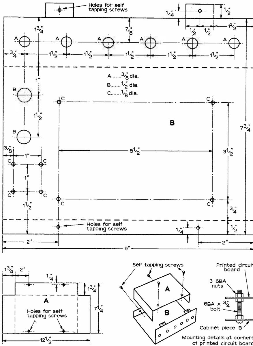
Fig. 12: The cutting and drilling details of the two piece aluminium cabinet.
