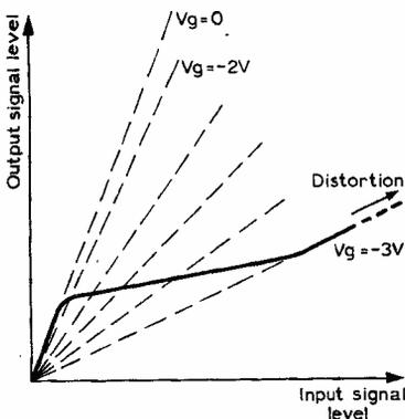
Fig. 6: The dashed lines on the graph show the audio stage gains at different f.e.t. gate voltages for the circuit in Fig. 5.
