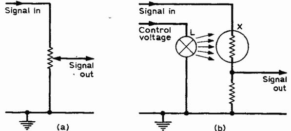
Fig. 1: A standard volume control and a simple method of audio expansion or compression using an L.D.R.
