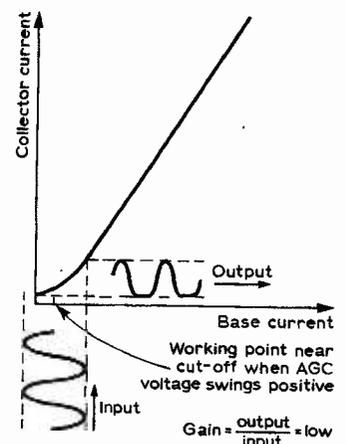
Fig. 2: Radio receiver a.g.c. circuit and graphs showing effect of a.g.c. on gain.
