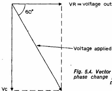
Fig. 5.4. Vector diagram showing 60° phase change produced by the CR network
