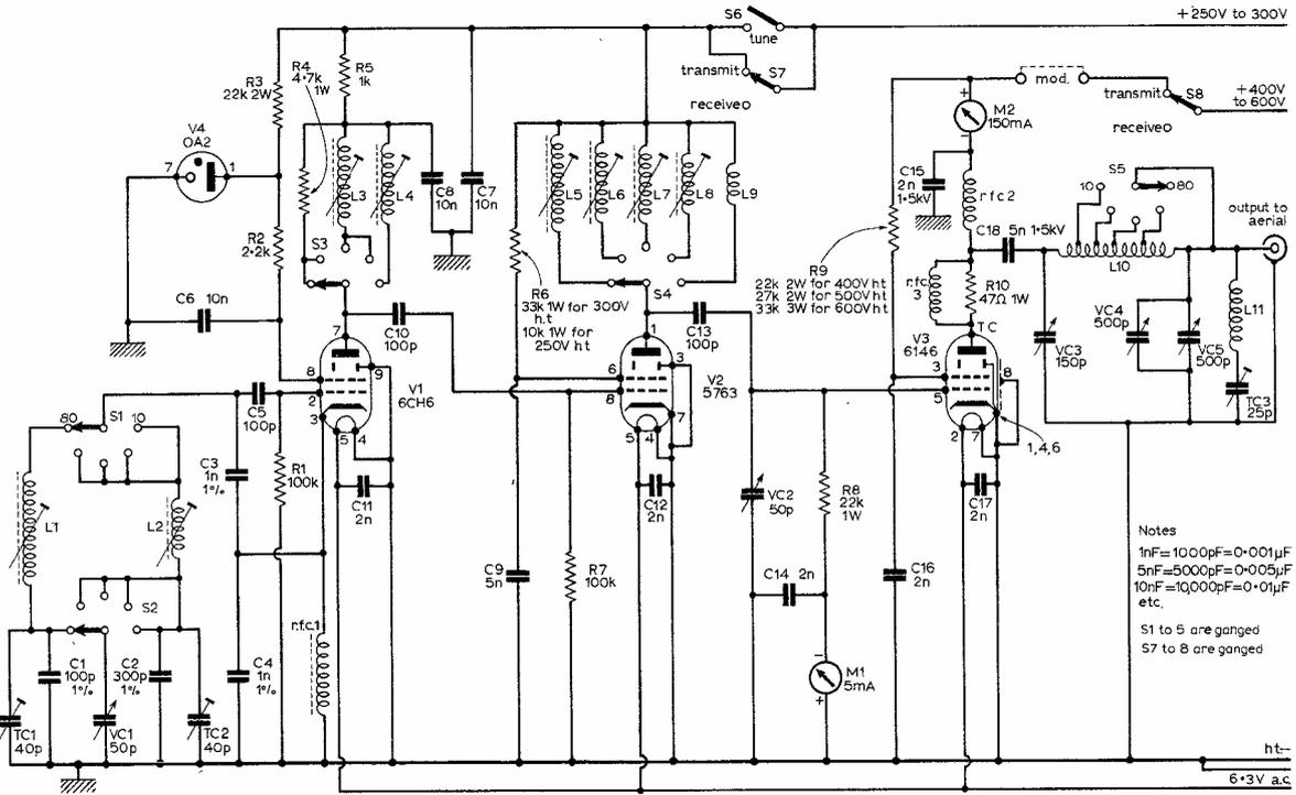
Fig. 1: Complete circuit diagram of the 5-band transmitter.
