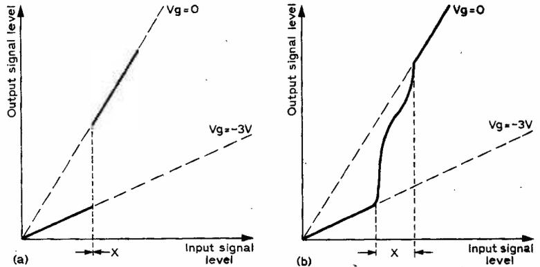
Fig. 7: Volume expansion characteristics of circuits discussed in text. In (a) expansion operates over an infinitely small range; in (b) the range is real but expansion is non-linear.
