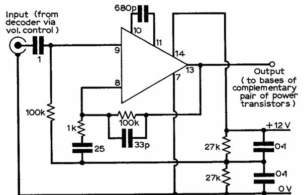
Typical circuit of one channel of a stereo preamplifier built around the MC1303.
