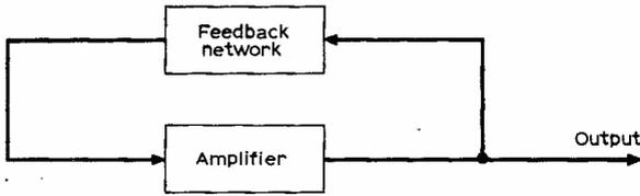
Fig. 5.2. Feedback network employed to produce an oscillator
