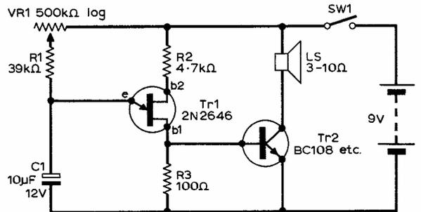
Fig. 1: The circuit of the metronome
