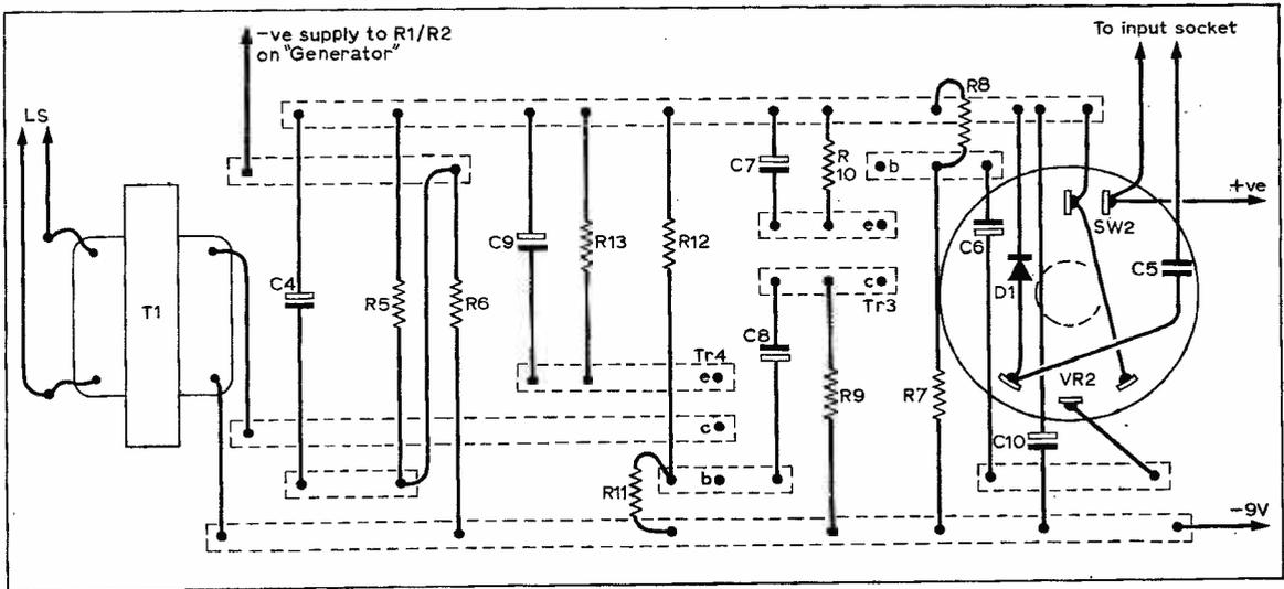
Fig. 3: Layout of the "tracer" circuit board, also full scale
