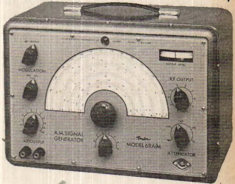
Fig. 16: The still popular Taylor Model 68A/M signal generator. Frequency range is from 100kHz to 240MHz (all on fundamentals) over 8 ranges. Although a.m. only, the instrument is suitable for the alignment of ratio detectors and f.m. r.f. and i.f. stages. A variable 400Hz audio output is available and an r.f. monitoring meter allows accurate setting of the signal applied to the attenuators.
