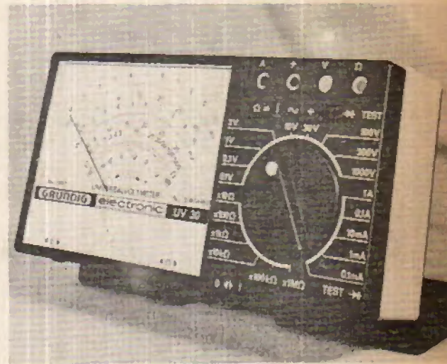
Fig. 10: A Universal Voltmeter by Grundig. Model UV30. This uses field effect transistors, is battery powered and pocket size. Impedance as high as 30M and resistance measurement from 1Ω to 500MΩ.
