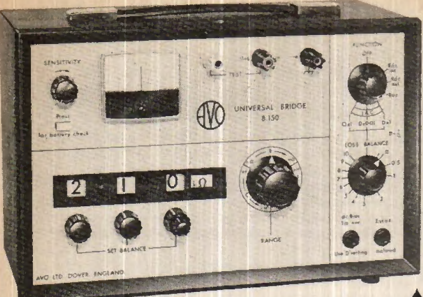
Fig. 13: For more advanced measurements and tests, this Universal Bridge by Avo, Model B.150, caters for a wide range of inductance, capacitance and resistance measurements. Balanced null point is indicated by a meter, while the value of the component under test is automatically presented in digital form.
