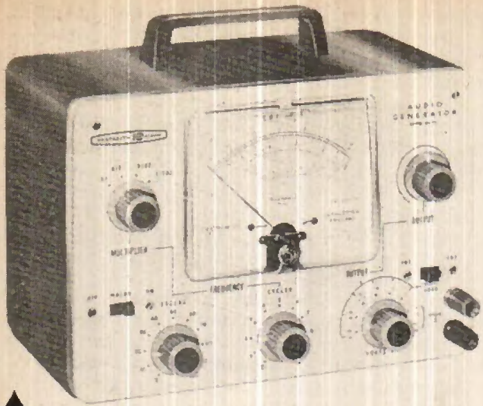
Fig. 7: Heathkit Audio Generator, Model AG-9U. Frequency range is from 10Hz to 100kHz with less than 0.1% distortion from 20Hz to 10kHz. Output voltage is indicated on a 4½in. meter with three scales of 1 and 3 volts and -10 to +2dB.
