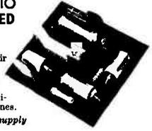
Especially designed by S.G.S. incorporating their proven Linear I.C. Audio Amp. TA(821) providing unlimited applications for the enthusiast in the construction of radios, record players, Audio and Stereo units. Also ideal for intercom systems, monitoring applications and phone answering machines.
