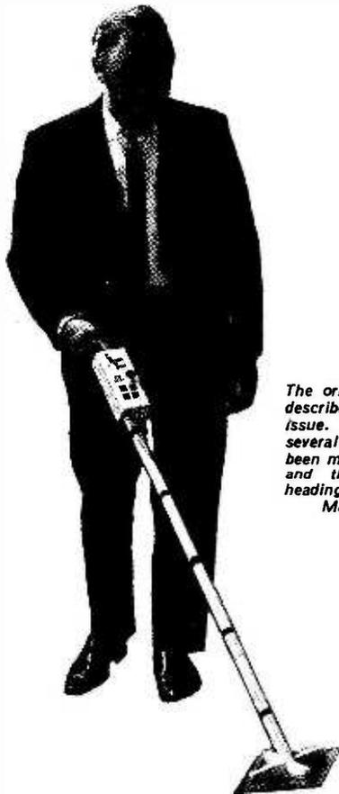
*The original Treasure Tracer, described in the August 1971 issue. The text mentions several improvements that have been made, both to the circuit and the construction. The heading photograph shows the Mark II in operation.*
