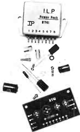
The HY41 supersedes the popular HY40 introduced by ILP last year. This highly improved module achieves true High Fidelity with a dramatic reduction in distortion (typically 0.05% at 1KHz into 8 ohms!) and is electronically and mechanically compatible with the HY40.
