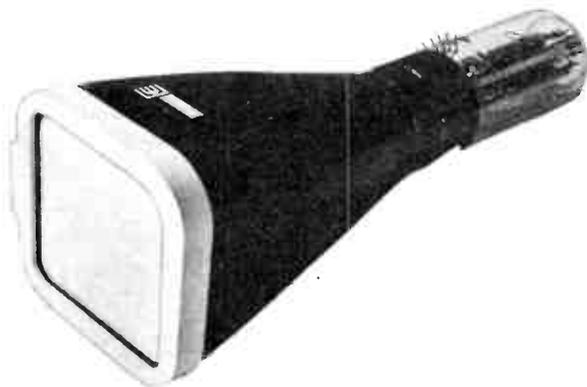
This E716A direct-view storage CRT is manufactured by the English Electric Valve Company has a viewing area of  $10 \times 10$  cm. Because of its good deflection sensitivities it is particularly suitable for compact transistorised equipment. The normal storage time is from less than one second to several minutes but this can be extended to several days!
