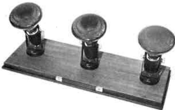
Photograph shows the lamps unit that is used with the P.W. *Tricolour*
