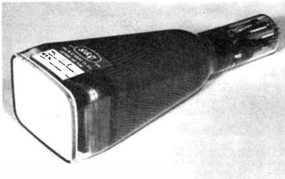
The Marconi-Osram Valve Company's 1400A single gun oscilloscope tube has a flat face with a display area of  $10 \times 8$  cm. The maximum final anode voltage is 4kV.
