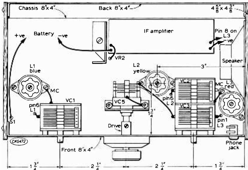
Fig. 2: Layout of the major components on top of the chassis.
