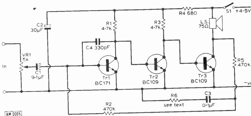
R4, and C2 are the supply decoupling components. The loudspeaker itself forms the collector load for Tr3. Speakers of other impedances can be used, but must have an impedance of at least 35Ω. Due to the large amount of d.c. negative feedback used in the circuit, altering the speaker impedance should not drastically change the operating parameters of the circuit.
