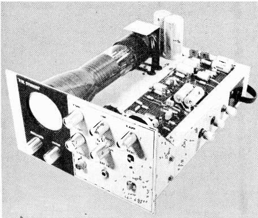
*Photograph showing the completed oscilloscope. The three controls on the right hand side of the chassis are X linearity, X shift and astigmatism.*
