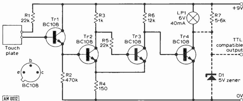
Circuit of the touch-sensitive switch, with alternative TTL output circuit.
