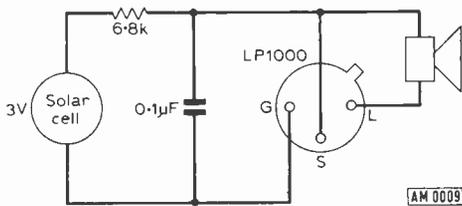
Fig. 3: Circuit using the LP1000 in a light-to-sound indicator.
