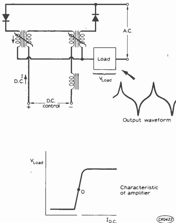
Fig. 7: Circuit of full-wave self-saturating magnetic amplifier with output waveform and amplifier characteristic curve.
