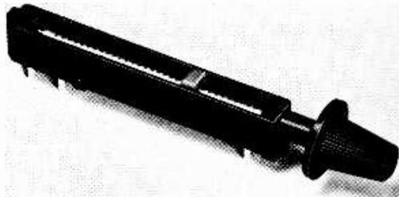
This 25-turn preset potentiometer by AB Electronic Components Ltd. is of carbon composition construction intended for use with varicap tuners. Resistance ranges up to 100kΩ in linear, logarithmic or diode characteristic law.
