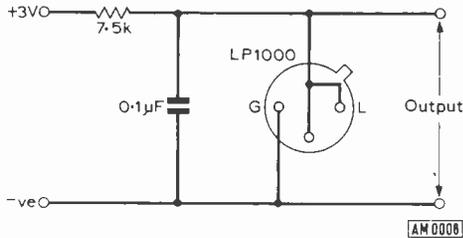
Fig. 2: LP1000 in a multivibrator circuit at 1kHz.
