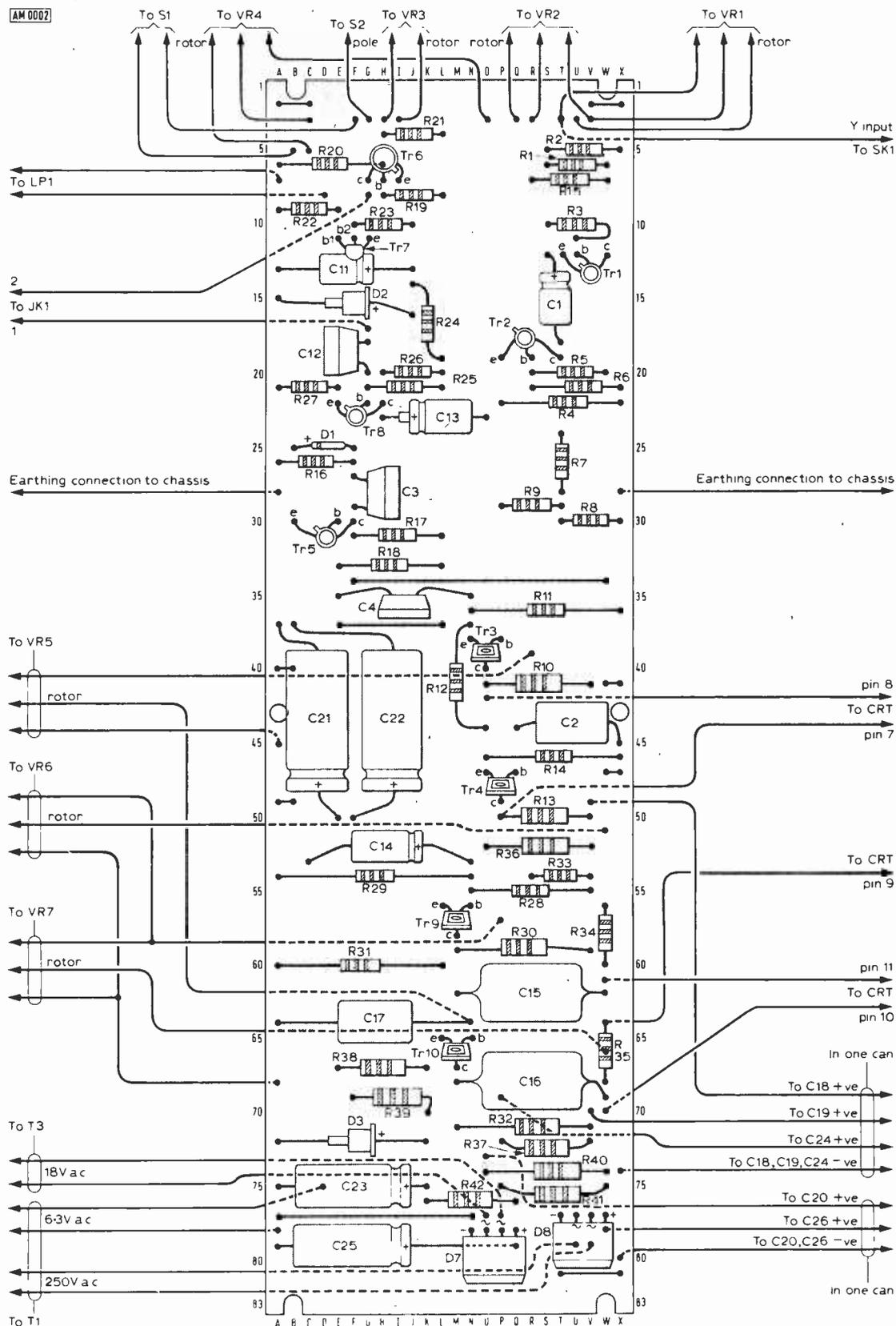
Fig. 2 The complete Veroboard layout for the oscilloscope.
