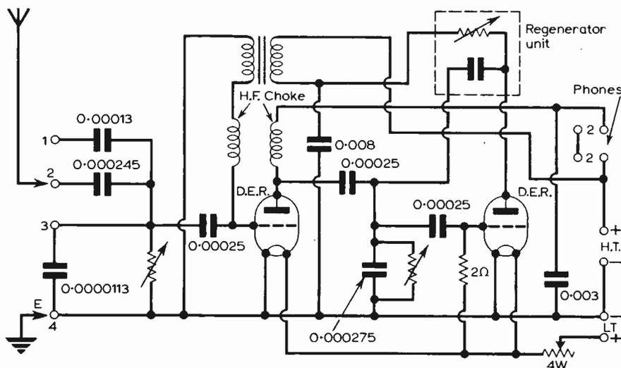
Fig. 1: The circuit of the Marconi V2 receiver re-drawn from the information supplied by Mr. J. Turner.
