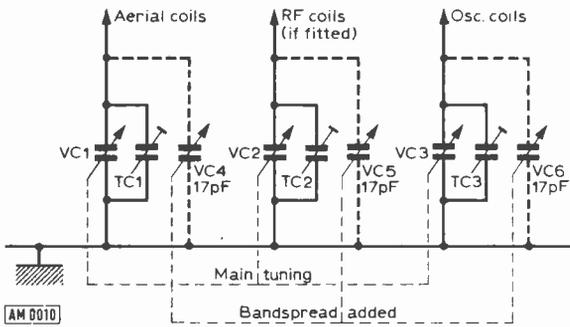
Fig. 1 Circuit showing the bandspread ganged capacitor added to the existing circuit.
