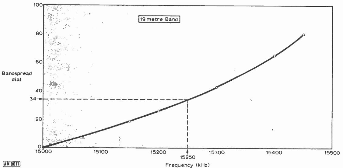
Fig. 2 A typical calibration chart produced by the method described in the article.
