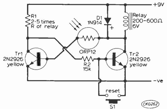
Fig. 4: Circuit for operating in a dark room.
