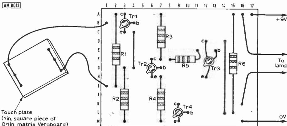
Layout of components on the Veroboard with details of the touch plate.
