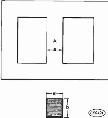
Fig. 9: The cross sectional area of the core can be obtained by multiplying 'a' and 'b' measured in cms.
