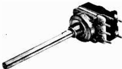
One of the Series C16 Cermet potentiometers by AB Electronic Components Ltd. Standard models range from 100Ω to 2.5MΩ, linear, but special models down to 50Ω and up to 10MΩ are available, with soldering tags or printed circuit terminals.
