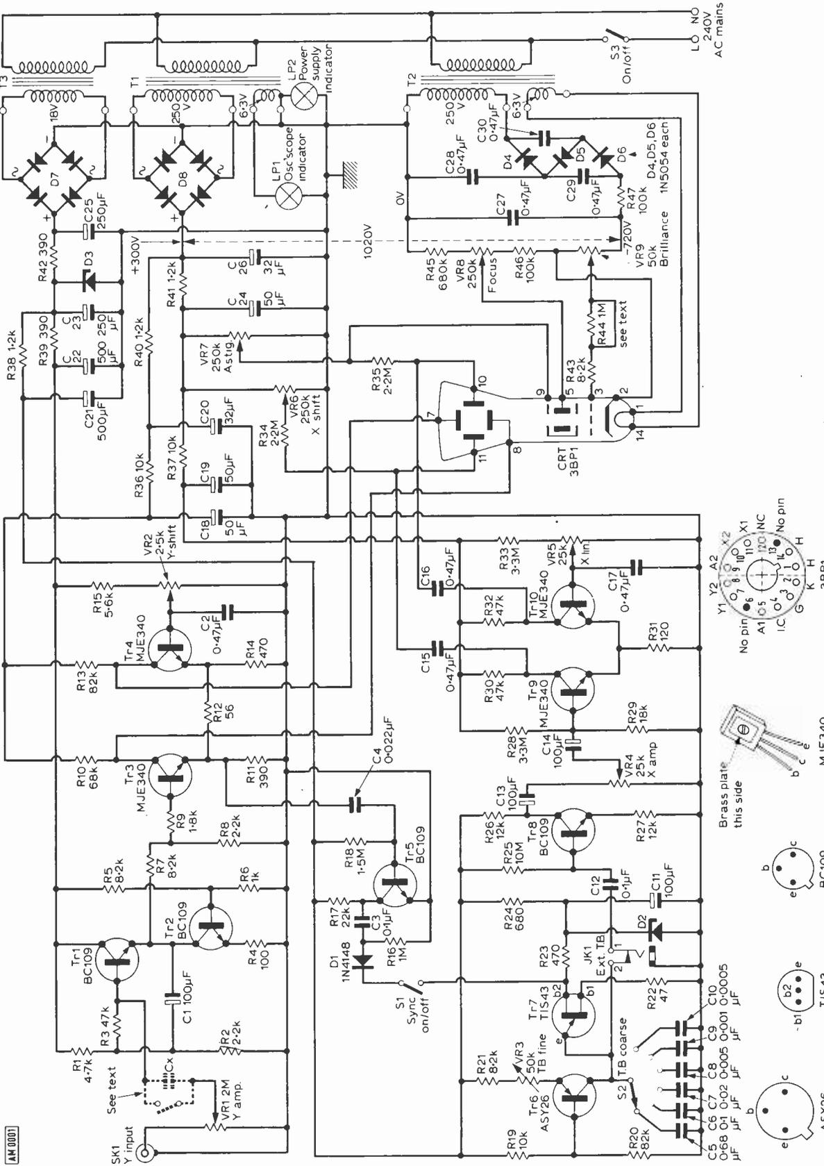
Fig. 1: Complete circuit of the P.W. Student Oscilloscope.
