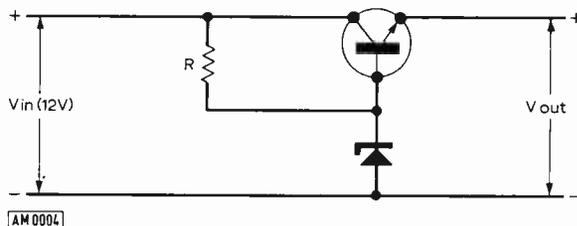
Fig. 1: Stabilising circuit for cassette recorders.
