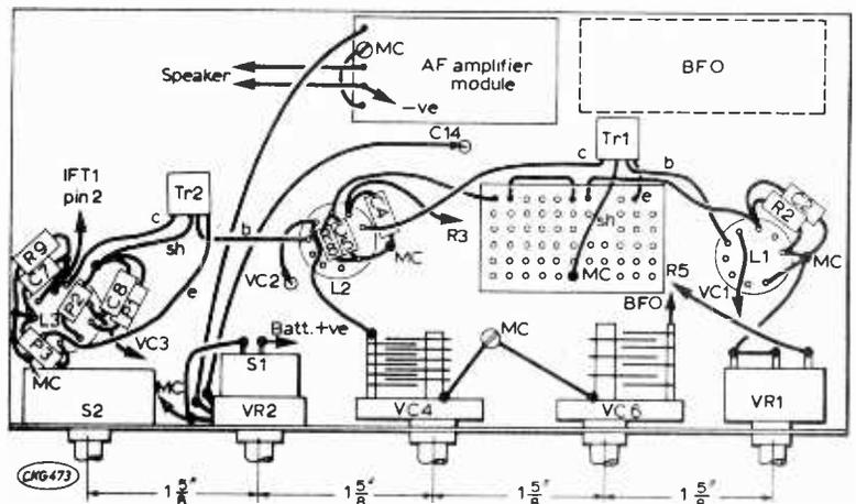
accuracy, to use a very small round file to enlarge the holes until the IFT's fit. A central hole is necessary under IFT1 and IFT2 to reach the lower cores.
