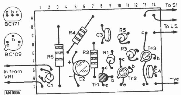
▲ Fig. 2: Component layout on the Veroboard.
