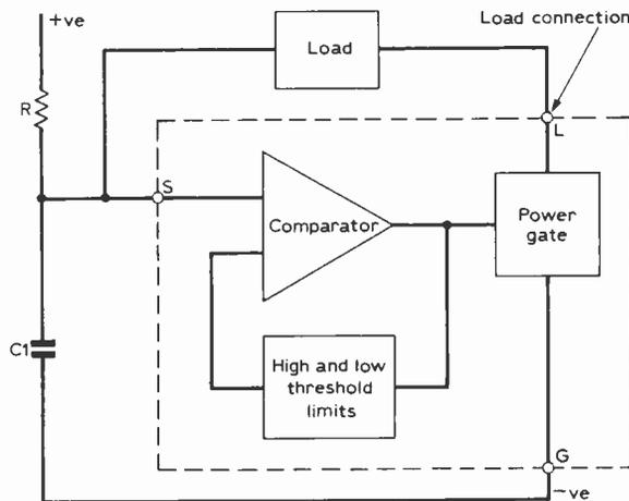
Fig. 1: Circuit diagram of the LP1000, together with a functional block diagram. The IC is produced in a TO-18 package.
