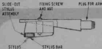
**STYLUS ARM/BAR.** Cantilever which carries the pickup stylus. It is suspended at one end so that it can be allowed to vibrate in a magnetic field or transmit mechanical stresses through a piece of piezo-electric material.
