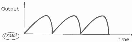
Fig. 1: Typical waveform of a timebase oscillator, used to control the sweep of the wobulator.
