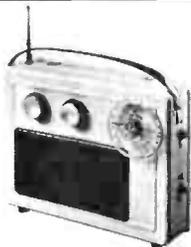
Nine Transistors, 9 Tunable wavebands as Roamer Ten Built in ferrite rod aerial for MW/LW. Retractable chrome-plated telescopic aerial for VHF and SW. Push Pull output using 600mW transistors, 9 Transistors and 3 diodes, tuning condenser with V.H.F. section, separate coil for aircraft, moving coil loudspeaker, volume ON/OFF and wavechange controls. Attractive all white case with red grille and carrying strap. Size 9½" x 7" x 2½" approx. Parts Price List and Plans 30p (Free with parts).
