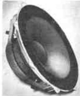
**15" 14A/780.** Bass unit on a rigid diecast chassis. Superior cone material handles up to 50 watts RMS, and is treated to give a smooth frequency response. Resonance 30 Hz. Flux density 360,000 Maxwells. Impedance at 1 kHz is 8 ohms. 3" voice coil.
