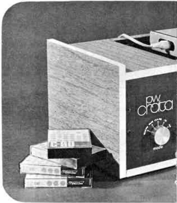
**T**HIS constructional feature describes a stereo-multiplex AM/FM tuner-amplifier providing 10 watts RMS output per channel into  $8\Omega$  loads with facilities for incorporating a cassette tape recorder. The integrated unit provides very good results which, although not to true high fidelity standards, will give satisfying listening for a moderate outlay.
