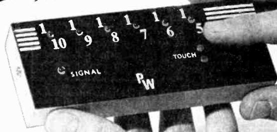
Here is an amusing device that will enable you and your friends to compare reaction times without any further argument! Full details given for the construction and calibration of the timer.
