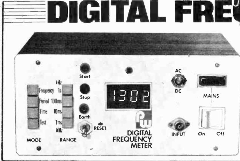
You'll probably find that you have a lot of the components already! An interesting constructional project which will give much satisfaction when it's completed. Readout to, typically, 27MHz or more depending upon the IC's used. Gate times of 100 $\mu$ s to 1s. Input 60mV to 10V and time intervals 1ms to 9999s.
