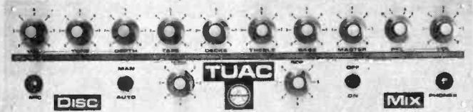
Designed for the discerning D.J. of professional standard. Offering a vast variety of functions. Controls: Mic Vol; Tone, over-ride depth, auto/Manual Sw; Tape Vol; L & R Deck Faders; Deck Volume; Treble and Bass; H. Phon Vol Selector; Master Vol on/Off Sw. Max output 1V RMS.
