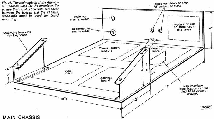
It only remains to make the final chassis and to assemble the Power Supply module, the three major boards, the keyboard interface board just described and the keyboard itself on it. Fig. 36 shows the chassis details as used for the prototype.
