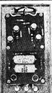
View of the first model of the Transistor Checker in which two boards were bolled together. The test sockets are at the bottom and the LED's at the top.
