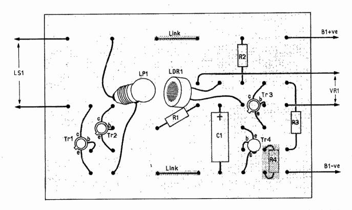
Full size drawing of the S-DeC showing the numbered holes into which the components are plugged. The LDR is soldered to long leads, to enable it to be 'waggled' in front of the bulb.
