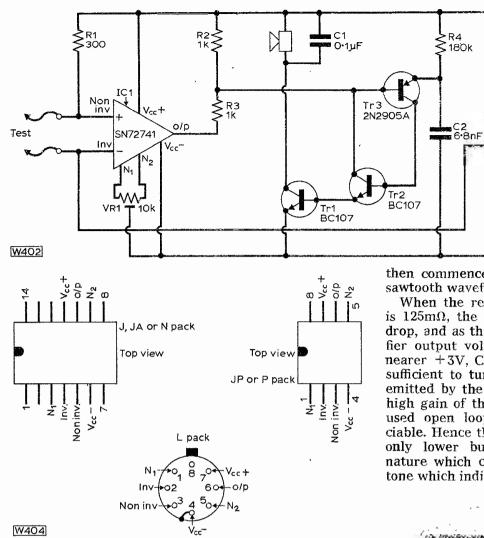
Fig. 2: Circuit of the unit developed by the author, which is much more precise in its indications.
