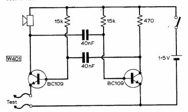
Fig. 1 : Circuit of a simple continuity tester with an earpiece or small speaker as indicator.
