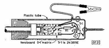
Fig. 7(a) above, shows the method of constructing the simple probe while (b) below, illustrates the location of the few components in the control box and the wiring.
