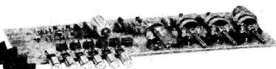
A top quality stereo pre-amplifier and tone control unit. The six push-button selector switch provides a choice of inputs together with two really effective filters for high and low frequencies, plus tape output.
