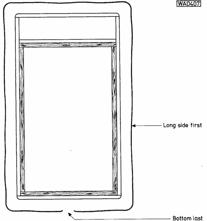
Fig. 3: Applying covering material to the cabinet
