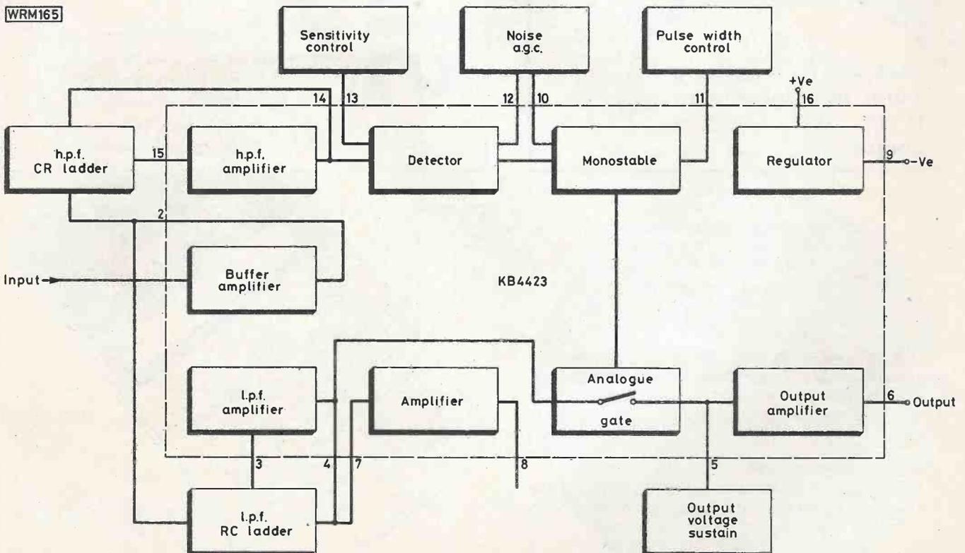
Fig. 1: General arrangement of the f.m. noise blanker based on the KB4423 i.c.
