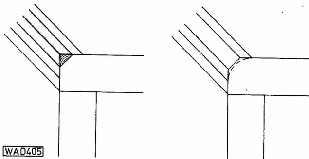
Fig. 2: (a) (left) marking for rounding edges; (b) (right) Initial planing of edge completed
