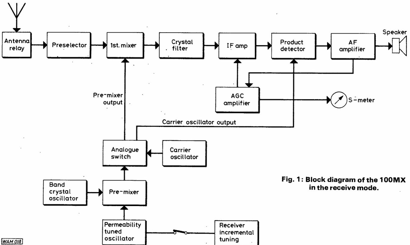
Fig. 1: Block diagram of the 100MX in the receive mode.
