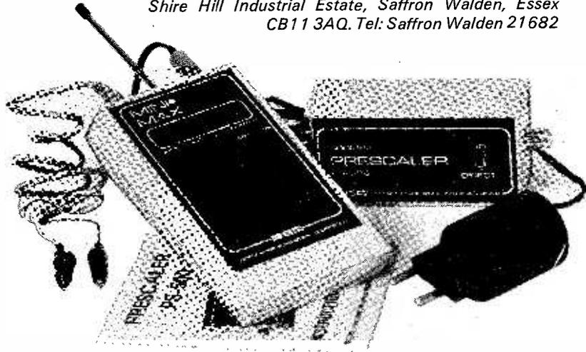
For the radio amateur some means of accurately measuring frequency is a must. The price of a reliable and simple to use counter has been beyond the reach of many amateurs, but the Mini Max counter from Continental Specialties Corporation should help to put this right.
