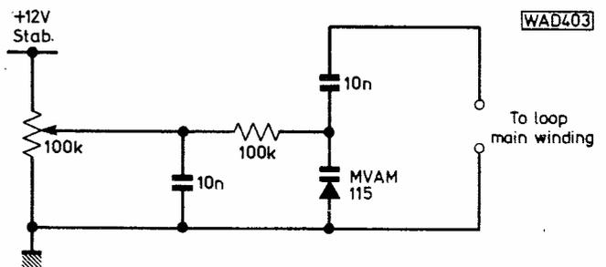
**Fig. 1: A medium-wave loop tuning circuit using a varicap diode**
