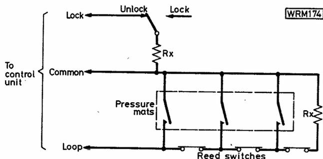
**Fig. 3. A very basic 2-wire security circuit. Devices are shown in the "non-alarm" condition**
