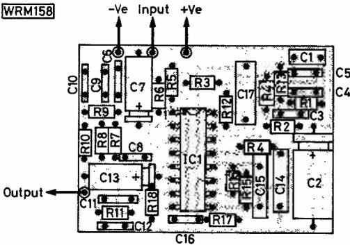
Fig. 4: Component layout and copper pattern of the p.c.b. (shown full size).
