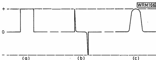
**Fig. 2: The output of the high pass filter (b) and low pass filter (c) for a rectangular pulse input (a)**
