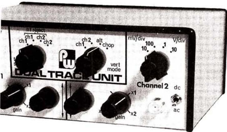
front panel mounted control is marked to indicate gain settings of  $\times 0.5$ ,  $\times 1$ , and  $\times 2$  and of course also covers the variable gain function thus combining the functions of two knobs on the Purbeck front panel. This arrangement was adopted to enable all the facilities of the Dual Trace Unit to be fitted onto a relatively small front panel, and the finished unit fits neatly in front of the Purbeck as in the photograph on the front cover.
