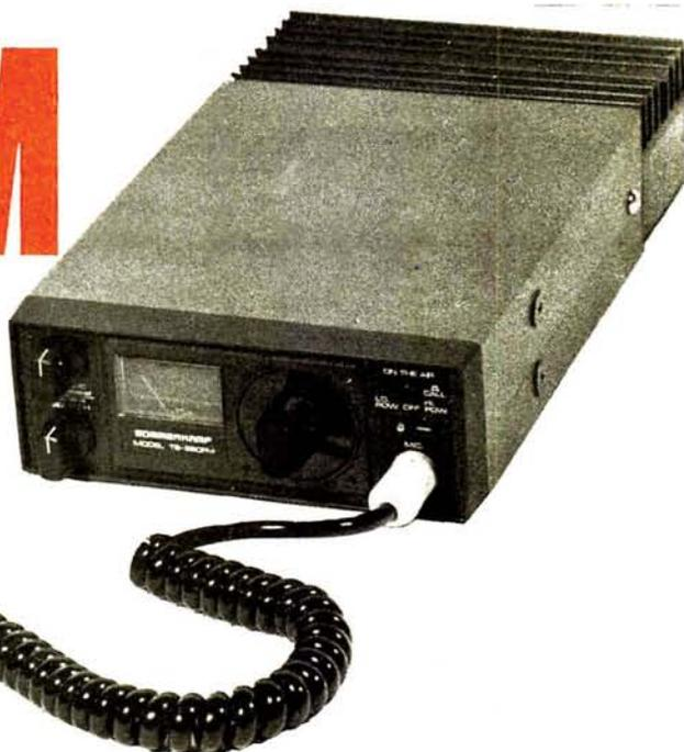
"Not just another synthesised rig, but a transceiver worthy of anybody's car dash board or glove shelf," is the opinion of the author about the TS280FM 2m f.m. transceiver. Sommerkamp, the European connection with Yaesu-Musen of Japan, have produced this rig with a 75W input capability to a fully frequency synthesised, all solid-state design for the 144-146MHz band.
