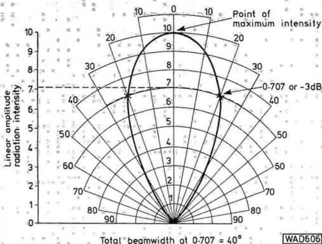
**Fig. 3: How the beam width of radiation at -3dB is established with reference to absolute intensity**
