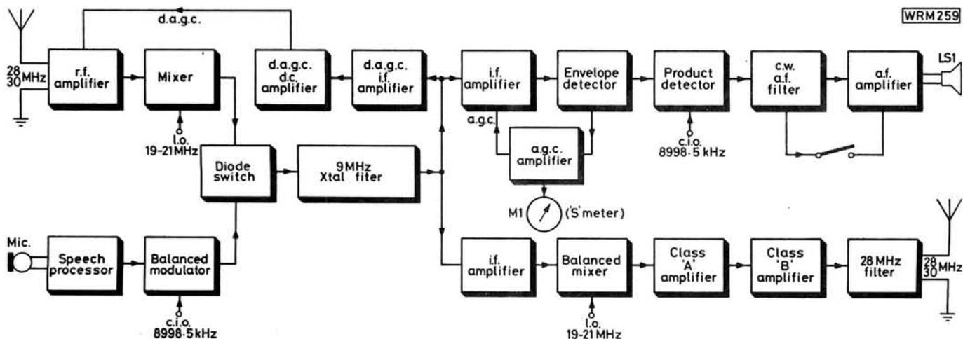
Fig. 1: The block diagram of the complete transceiver
