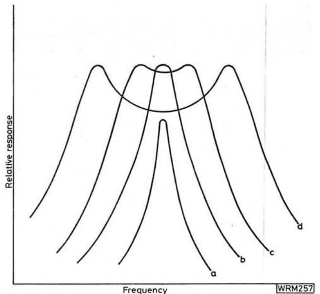
**Fig. 12: Response curves for two parallel tuned circuits under various conditions of coupling**
