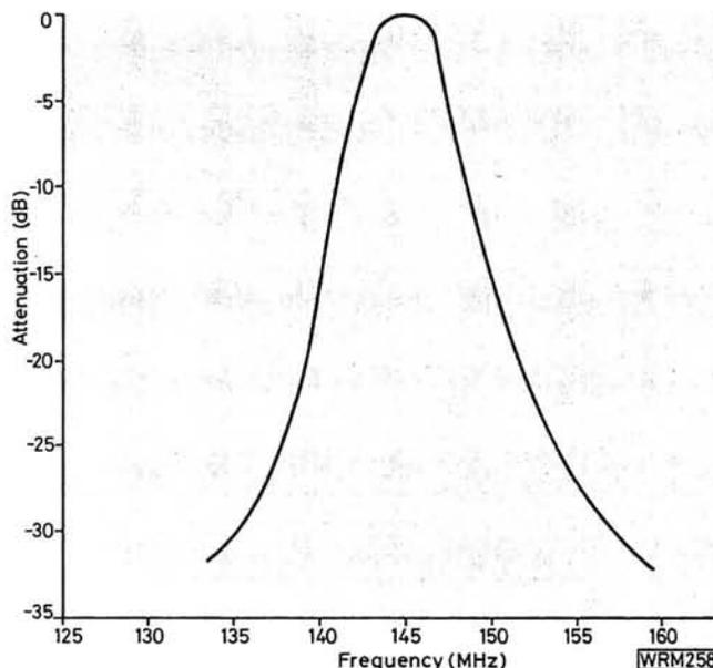
Fig. 15: The frequency response of the filter unit
