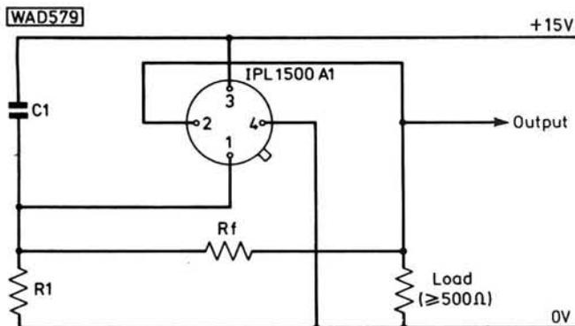
Fig. 7: Circuit for increasing the hysteresis level
