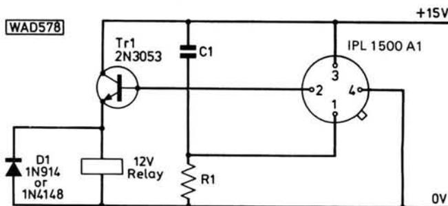
Fig. 6: The switching circuit for a heavy-duty relay
