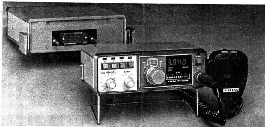
The latest idea in v.h.f. and u.h.f. mobile rigs is separates. The Yaesu FT-720R is such an animal with pluggable 70cm and 2m r.f. units. Further details
