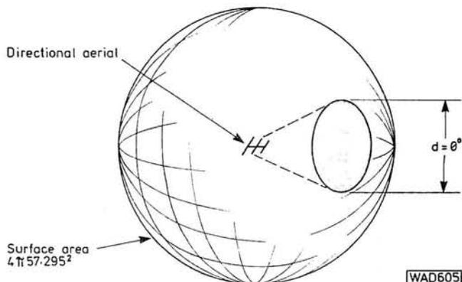
Fig. 2: Area of directed radiation in relationship to that otherwise produced by an isotropic source
