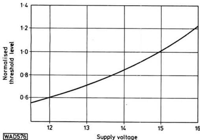
Fig. 4: Variation of switching threshold level with supply voltage
