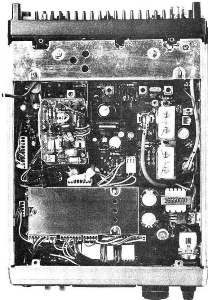
**Interior view of the Standard C7800 with the bottom cover removed. The substantial heatsink is at the top**
