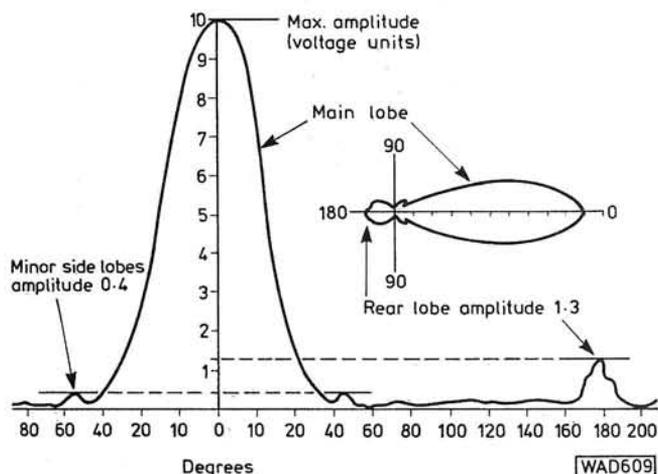
**Fig. 6: How the dB level of rear and other minor lobes is related to gain of main lobe at maximum intensity**
