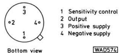
Fig. 2: Pin connections
