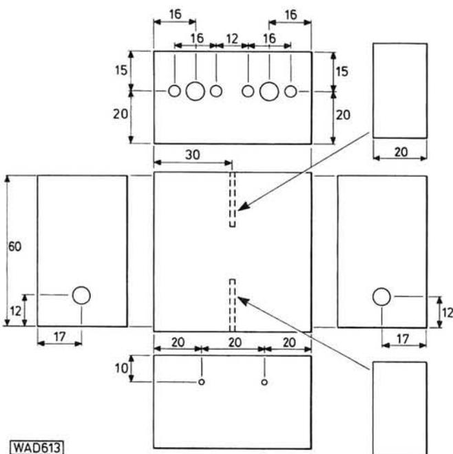
Fig. 13: Mechanical details of filter screening prior to assembly. All dimensions in mm
