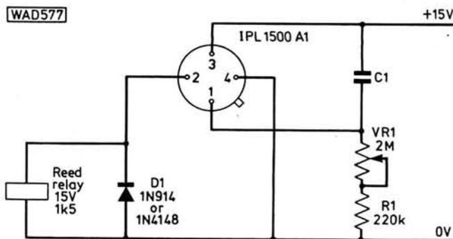
Fig. 5: A simple reed relay switching circuit
