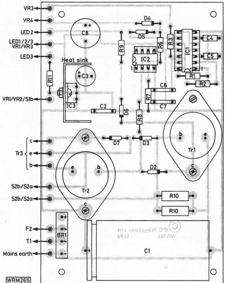
**Fig. 4: The copper track pattern for the p.c.b. shown full size. The component placement drawing Fig. 5 is shown above right. Components not mounted on this board should be fitted onto the control panel using the tags on the potentiometers as mounting points**
