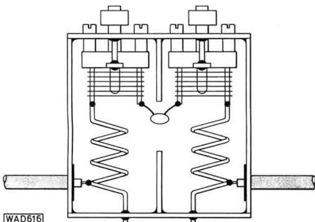
Fig. 14: Internal layout of the filter unit
