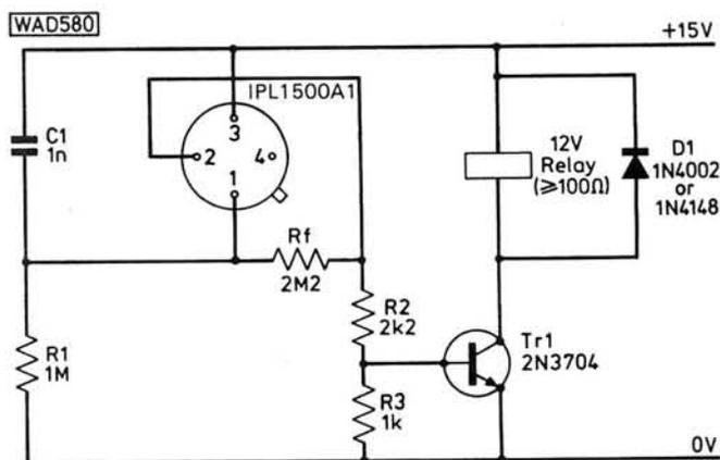
Fig. 8: A complete heavy-duty switching circuit
