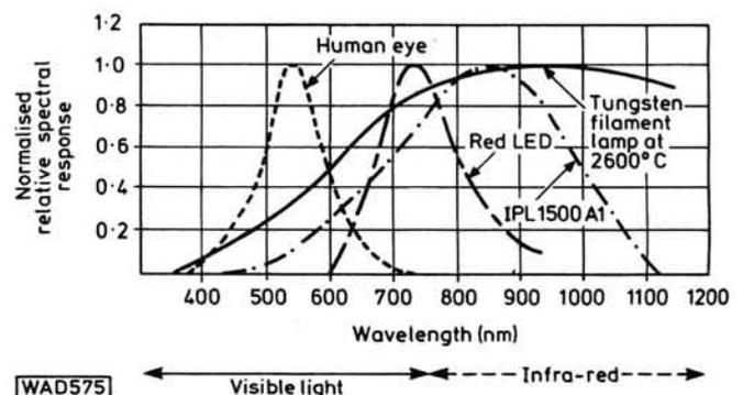
Fig. 3: The spectral sensitivity of the IPL1500A1
