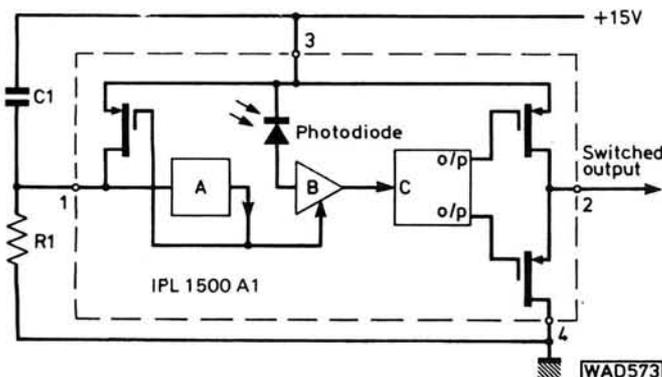
Fig. 1: The internal circuit of the IPL1500A1
