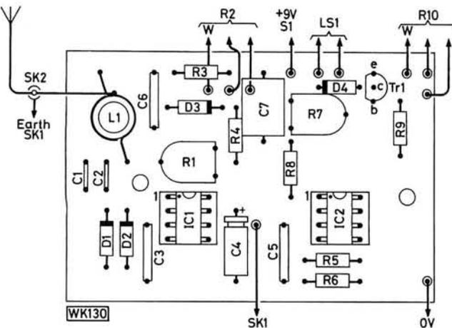
Fig. 2: Track pattern and component layout of the meter
