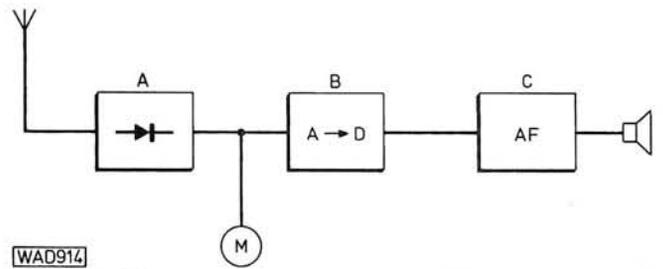
Fig. 3: Block diagram of the audible field strength meter
