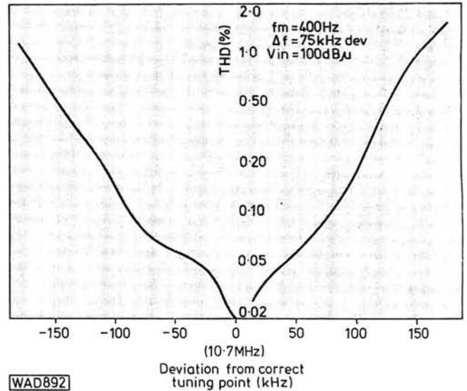
**Fig. 4: Increase in total harmonic distortion as the tuning is adjusted on either side of the correct tuning point**
