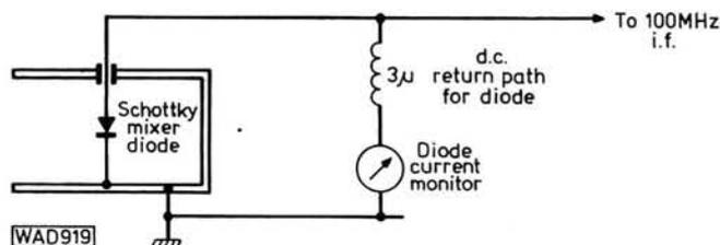
Fig. 14: Schottky mixer diode current monitor circuit
