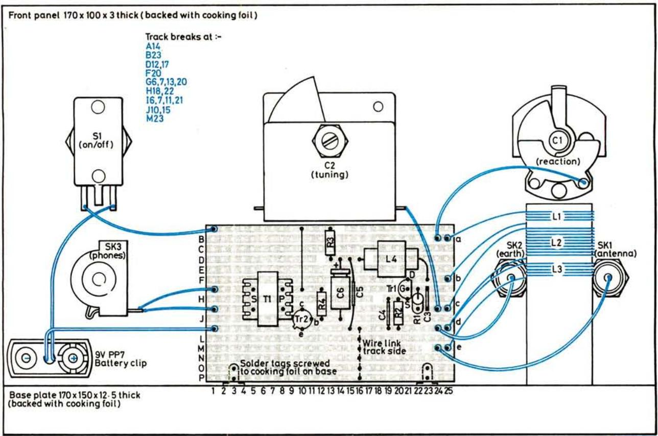
Fig. 2: Interwiring and Veroboard layout. This drawing is to scale to allow the front panel layout to be copied
