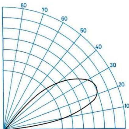
$5/8\lambda$  antenna, gain 3dB radiation angle  $30^\circ$
