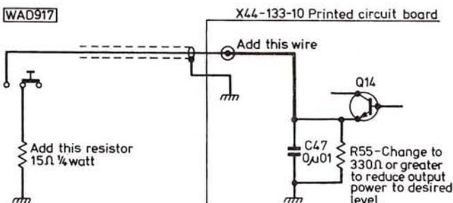
If you decide that you would like an even lower output, simply increase the value of the Q14 emitter resistor, but keep in mind that the value of the emitter resistor and the sub-tone switch resistor when connected in parallel must equal  $10\Omega$  if you want to maintain full output power when the switch is open.
