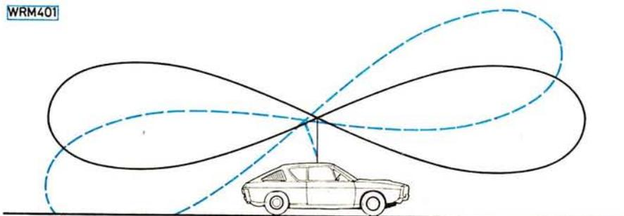
◀ Fig. 1:  $5/8\lambda$  antenna radiation pattern—solid line vehicle stationary—dotted line vehicle on the move
