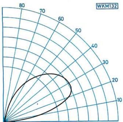
$\lambda/4$  antenna, gain 0dB radiation angle  $44^\circ$
