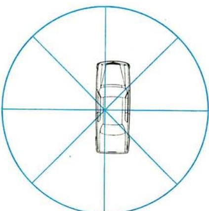
$5/8\lambda$  antenna gutter mounted
