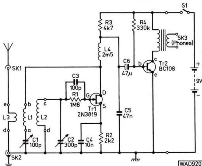
Fig. 1: The circuit diagram of the s.w. receiver
