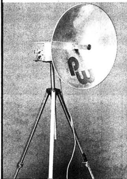
The antenna system designed for the PW Exe uses a specially designed and spun aluminium dish and arrangements have been made for the supply of this special item to our readers.
