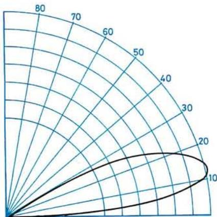
PW Slim Jim, gain 5.5dB radiation angle  $15^\circ$
