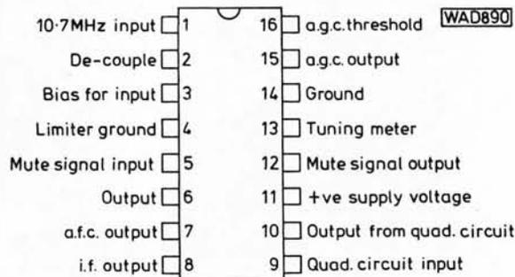
Fig. 1: Connections of the HA11225 and KB4441 devices
