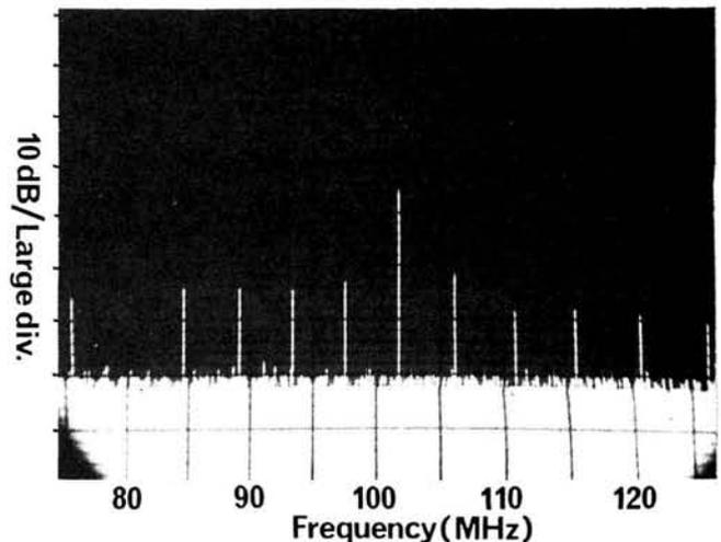
Spectrum analyser photograph showing relative harmonic output and amplitudes
