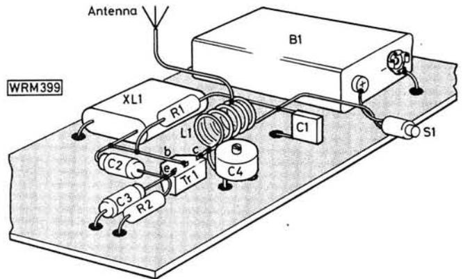
Fig. 12: Component layout details of the oscillator
