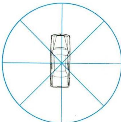
$5/8\lambda$  antenna mounted centrally on the roof
