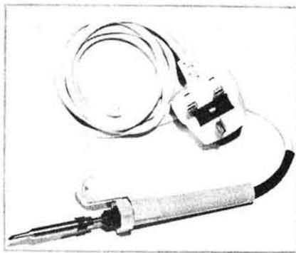
With a power consumption of 17W, the CS model produces a maximum tip temperature of 420°C. The larger 25W model produces up to 400°C with much greater thermal capacity for use as a general purpose soldering iron.
