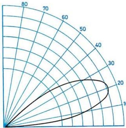
$7/8\lambda$  antenna, gain 4dB radiation angle  $25^\circ$
