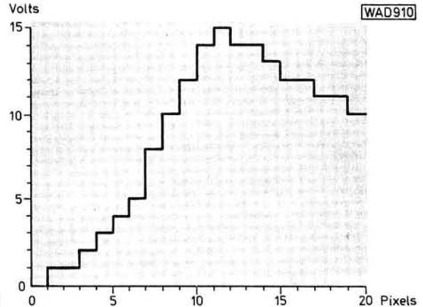
**Fig. 11: Digital representation of signal**
