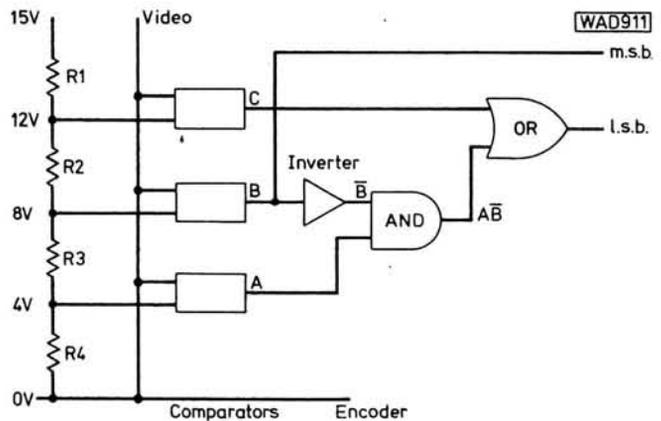
**Fig. 12: 2-Bit A-D Converter**
