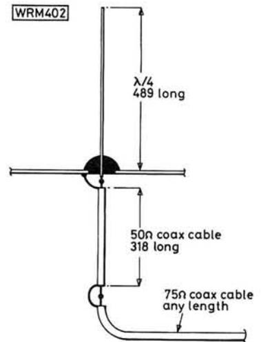
Fig. 3: Coaxial matching transformer system ▶
