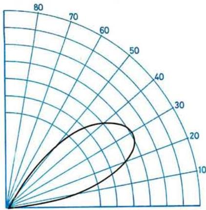
$\lambda/2$  antenna, gain 2dB radiation angle  $35^\circ$
