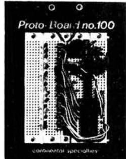
PB 100 Kit complete with 760 contacts accepts up to ten 14-pin Dips, with two binding posts and sturdy base. Large capacity with Kit economy.
