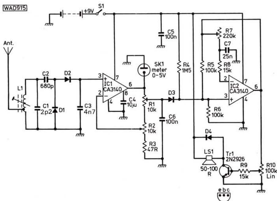
Fig. 1: Full circuit diagram for the audible field strength meter
