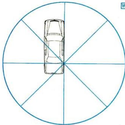
$\lambda/4$  antenna mounted on the rear wing
