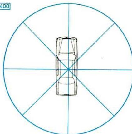
$\lambda/4$  antenna mounted centrally on the roof
