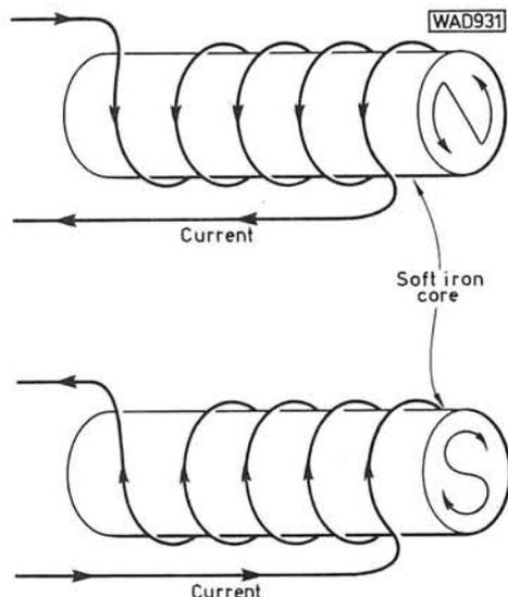
**Fig. 12: Field direction in a solenoid**
