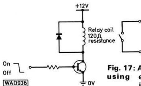
**Fig. 17: A practical circuit using energy in an inductor**
