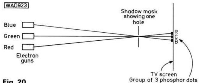
which glows blue when energised by an electron beam, whilst the other two glow green and red respectively.
