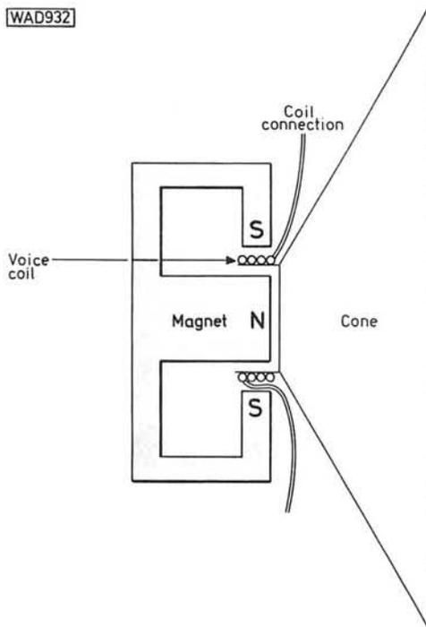
**Fig. 13: Loudspeakers use the effects of electromagnets to produce their sound**
