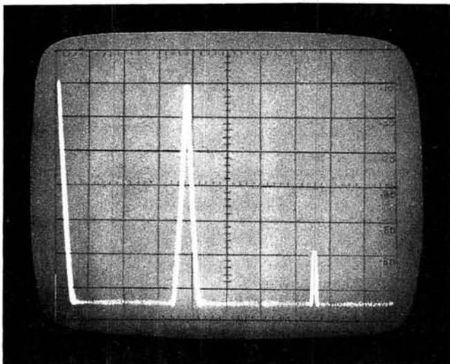
**Fig. 44: The fundamental frequency plus the second harmonic at 80m. This may be seen to be approximately 50dB down on the wanted signal. The noise floor at about 65dB down is the only other signal present; all other spuri are therefore >60dB down**
