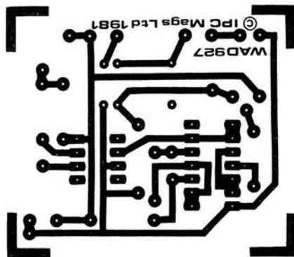
Fig. 2: The track pattern of the p.c.b., shown full size
