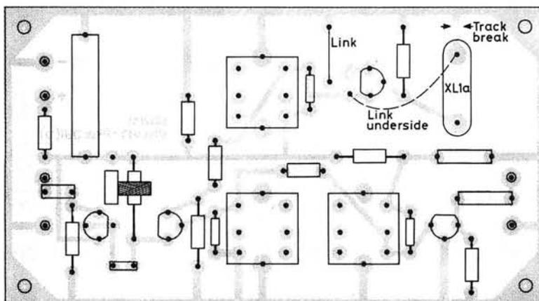
Fig. 5: Required modification for fundamental operation of the crystal oscillator
