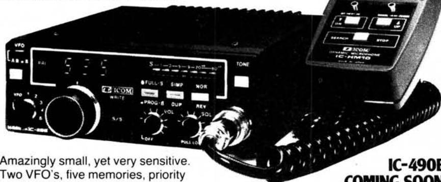
Amazingly small, yet very sensitive. Two VFO's, five memories, priority channel, full duplex and reverse, LED S-meter, 25KHz or 5KHz step tuning, same multi-scanning functions as the 290 from mic or front panel. All in all the best 2M FM mobile ICOM have ever made.
