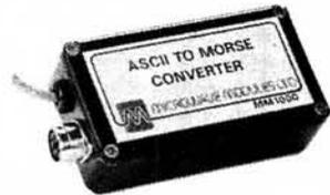
This microprocessor controlled unit enables any parallel ASCII keyboard to send variable speed morse in the range 12-30wpm.
