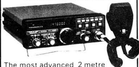
The most advanced 2 metre mobile available today - USB, LSB, FM, CW full scanning with priority channel, 4 memory channels, dual synthesized VFO system.
