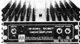
This all new 10 metre solid-state linear amplifier is intended for use with any existing 28MHz equipment having an output power of up to 10 watts. When used with such a drive source this unit will provide an output power of 100 watts on SSB and FM and 40 watts on AM.
