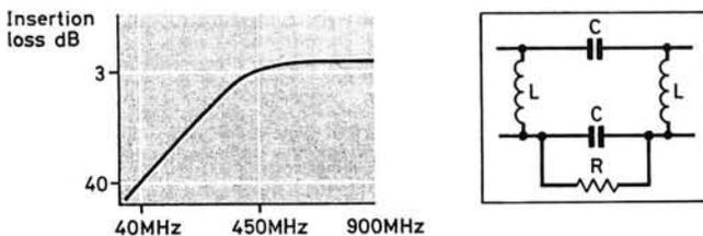
**Fig. 3(b): Typical circuit and frequency response of a high-pass filter suitable for use with the UK u.h.f. TV service**
