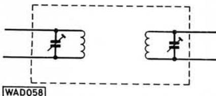
Fig. 1: Original i.f. transformer
