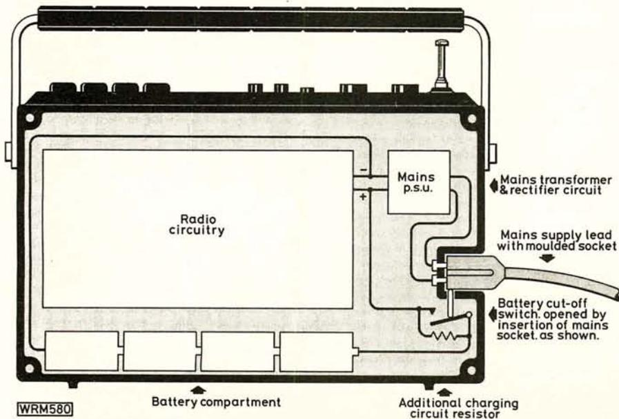
**Fig. 1: Schematic layout of an average mains/battery portable radio showing the modification required to provide charging current when using a NiCad battery pack.**
