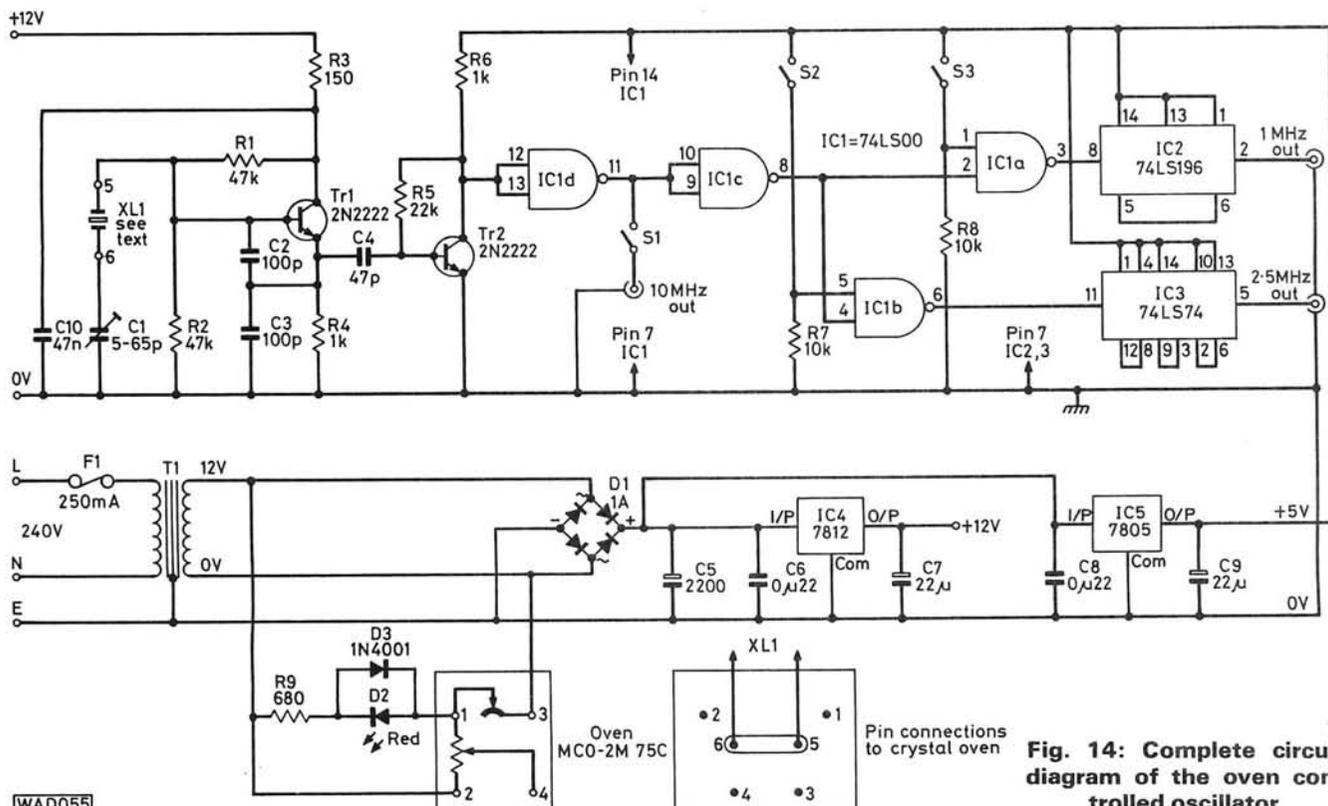
**Fig. 14: Complete circuit diagram of the oven controlled oscillator**
