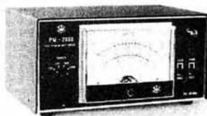
The PM-2000 is an accurate means of measuring your peak envelope output of power on SSB. The unit has been inspected by the home office and found suitable for its purpose. SWR measurements can also be made, but the PM 2000 does what all other SWR meters cannot do; i.e. tell you your peak output power as required in your licence. **PRICE £46**
