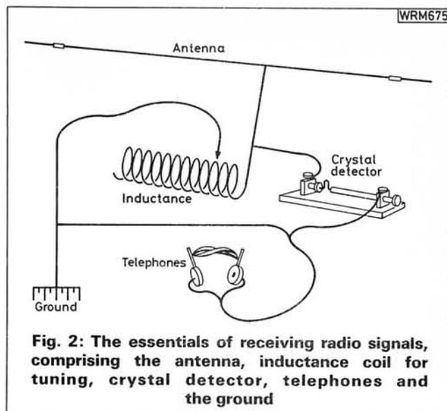
**Fig. 2: The essentials of receiving radio signals, comprising the antenna, inductance coil for tuning, crystal detector, telephones and the ground**
