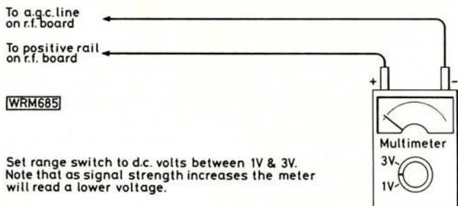
**Fig. 6: Increased directional resolution can be obtained by using a larger scale meter**
