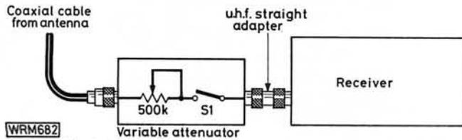
**Fig. 3: Variable attenuator; switch contacts should be fairly close together when open to ensure capacitive coupling**
