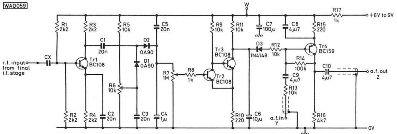
Fig. 1: Circuit diagram of the Add-on Squelch
