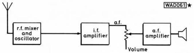
Fig. 2(a): Block diagram of a simple superhet receiver
