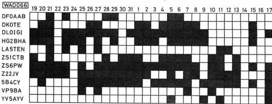
Fig. 1: Distribution of 28MHz beacon signals
