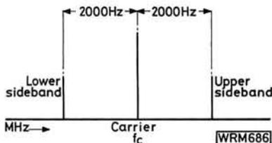
**Fig. 1:** In conventional a.m. signals the carrier and two sidebands are radiated as with a 2000Hz audio tone shown here. Several other components are produced by the modulating process but can be ignored here. SSB is only a variation of a.m.
