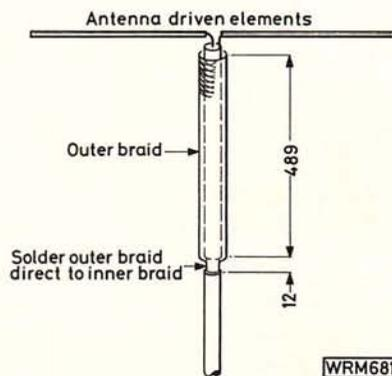
**Fig. 2: Details of the  $\lambda/4$  "Bazooka" 1:1 balun. The additional outer braid was obtained from a length of larger coaxial feeder**
