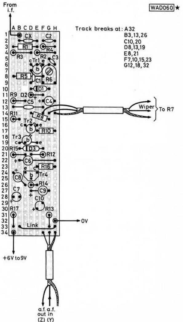
Fig. 3: The suggested Veroboard layout for the squelch circuit
