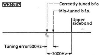
**Fig. 2:** Distortion of the modulation results if the carrier lost in generating an s.s.b. signal is not replaced in the receiver by a local oscillator of exactly the same frequency. In practice the injection is made after the signal has been converted to the i.f. and not at carrier frequency as shown here
