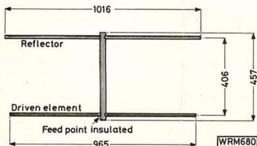
**Fig. 1: The layout and dimensions of the modified Band I TV antenna**
