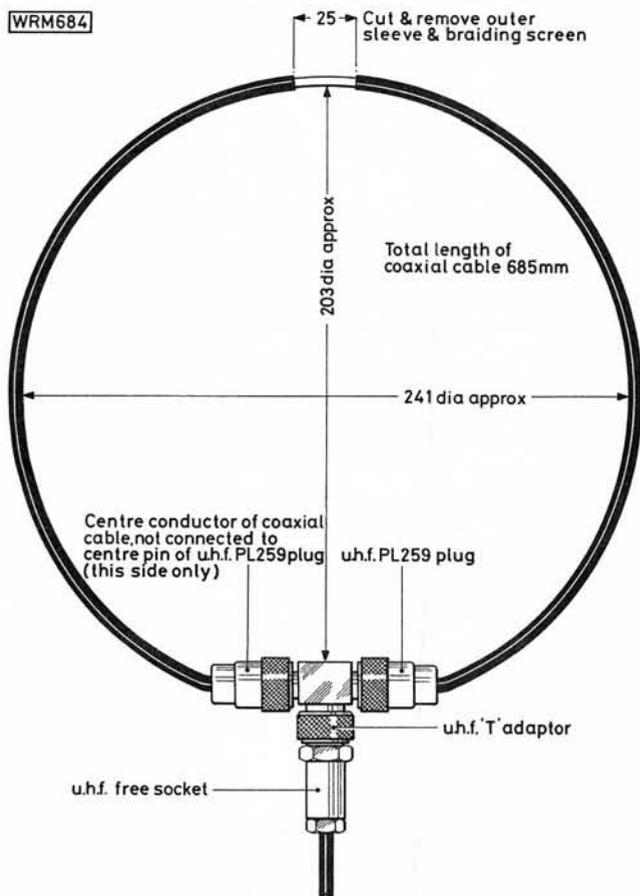
**Fig. 5: The untuned shielded loop antenna used for "close-in" work. This layout works well at 27, 28, 70 and 145MHz, peaking at 60MHz and with reduced efficiency on other frequencies**
