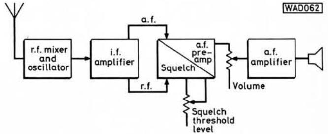
Fig. 2(b): Block diagram of the receiver with squelch added
