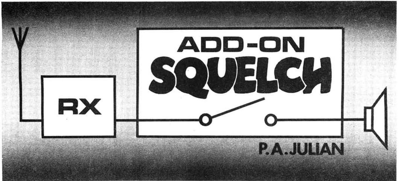
A squelch circuit is an electronic means of shutting down the audio stage of a radio receiver while no signal is being received. When a signal of a pre-determined level is received the audio stage is automatically switched on. This type of circuit is particularly useful in two-way radio applications where, under "no signal" conditions, background and ignition noise can be tiresome. Squelch can also be used in v.h.f. f.m. receivers to provide muting while tuning between stations.
