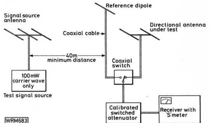
**Fig. 4: Test set-up for optimising DF antennas. The arrangement of equipment on the right also forms the basis for a good operational DF system**
