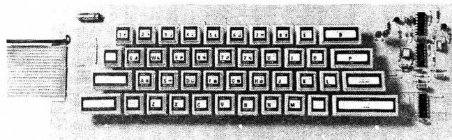
The actual keyboard connections are made via two ribbon cables which are plugged into the two sockets used for the ZX81 keyboard tails. I had great difficulty in keeping the wire ends actually in the sockets and intend to change the sockets for either soldered joints or a totally different plug and socket system.
