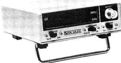
Power is either from internal batteries (six R6/HP7 cells) or an external 7.5V d.c. supply at about 130mA maximum. A word of warning when using an external supply—the rear-panel input connector is a coaxial type, recessed inside the metal case. The sleeve of the connector is the positive, and the counter case is negative.
