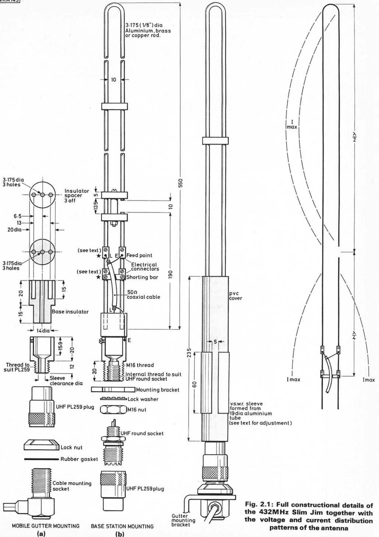
Fig. 2.1: Full constructional details of the 432MHz Slim Jim together with the voltage and current distribution patterns of the antenna
