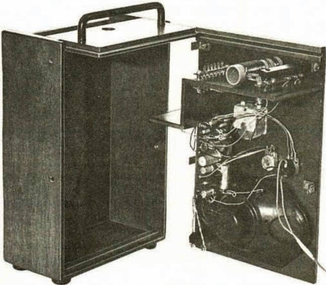
**Fig. 5: An exploded view of the author's receiver and its wooden case. The wires disappearing to the right are connected to the 9V battery**
