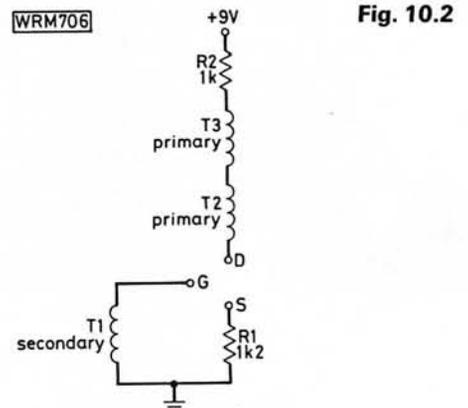
Under these fault conditions, the voltage being developed across R1 could not be applied between gate and source because of the break in the circuit. Consequently the channel was a low resistance, high current flowed, and most of the 9V was distributed between R1 and R2.
