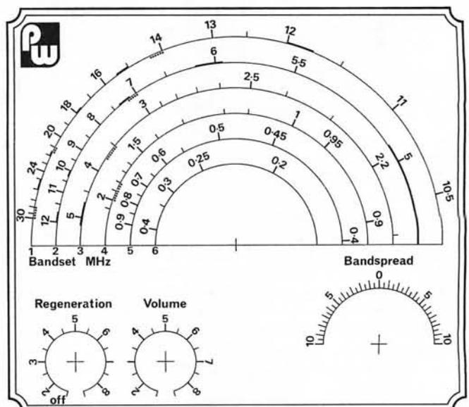
Fig. 4: The front panel dial of the LMS receiver, shown here half full size. Solid lines around the scale are broadcast bands with amateur allocations shown dotted
