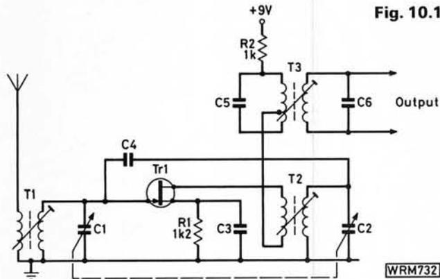
**No. 1:** Given that the source potential was +2V, and oscillations and signals were suppressed, you were asked to estimate the gate and drain potentials with respect to earth.
