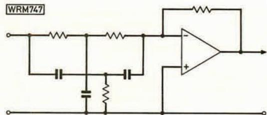
Fig. 1: The basic bridge circuit
