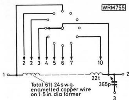
**Fig. 3: Circuit of a.t.u., matching wire antenna to receiver on any h.f. band. Cardboard centre of toilet roll makes ideal coil former. Prick small holes at one end to anchor wire, wind on two turns, scrape wire clean and twist small loop. Leave 3mm space, wind on two more turns, make another loop, space, three turns, make loop, and so on. The coil is mounted directly on capacitor and switch. Use insulating panel to isolate capacitor or mount on insulating pillars on aluminium panel**
