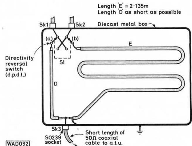
Fig. 3: Internal details of the phase reversing unit
