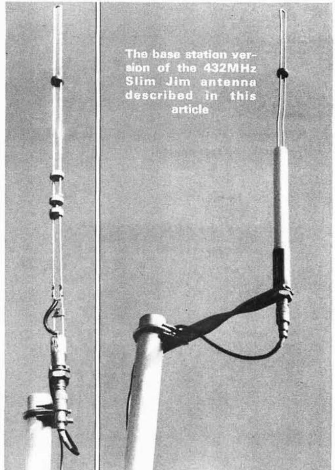
accomplished by adjusting the position of the v.s.w.r. sleeve between the base of the antenna and the top of the  $\lambda/4$  lower matching stub section.
