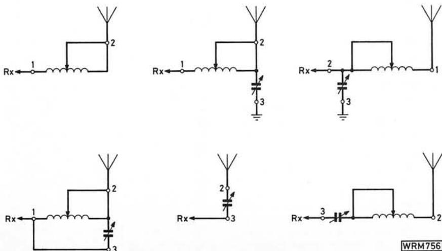
**Fig. 4: Six variations of a.t.u. circuit. Antenna, earth and receiver input leads fitted with wander plugs to fit sockets 1, 2 and 3. Optimum circuit depends on frequency and antenna's length**
