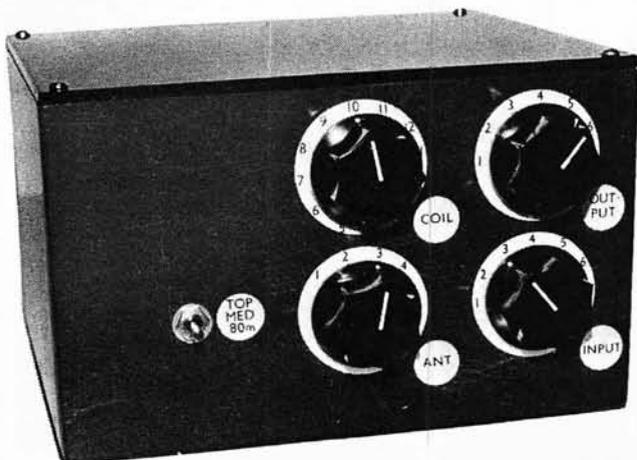
Cardboard discs are glued behind the knobs and marked by Letraset or similar system. The discs used were obtained from the local stationers in the form of "conference badges". The centres were removed by perforating them with the aid of a domestic sewing machine.
