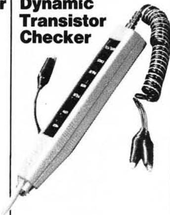
Obtains power from circuit being tested. Indicates high, low or pulsed (to 10 MHz) logic states. Minimum detectable pulse width is 50 ns. Tests almost every logic family including TTL, LS, CMOS, DTL.  $7\frac{3}{4} \times 1\frac{1}{8}$ ". 34" leads. 22-301 ..... £15.95
