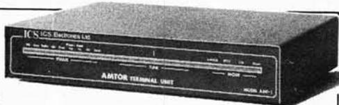
This AMTOR terminal unit (Amateur Teleprinting Over Radio) is a micro-processor controlled error-correcting data communication system, allowing virtually error-free data transmission between suitably equipped stations. Made in England by ICS Electronics, it offers full AMTOR error-correcting facilities plus RTTY, ASCII and CW (transmit only).
