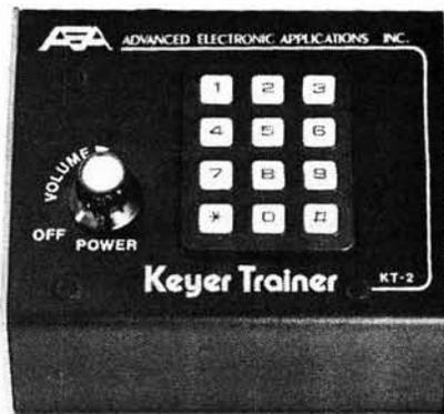
overridden by simply touching any key pad or the paddle. Semi-automatic or "bug" key operation can be selected instead of the normal iambic operation. A sidetone can also be selected.
