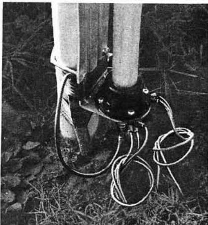
The HF5 base, with connections to five buried radials for improved soil conductivity
