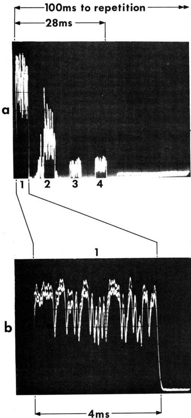
Fig. 2.6: Four pulse modulated "Woodpecker" signals
