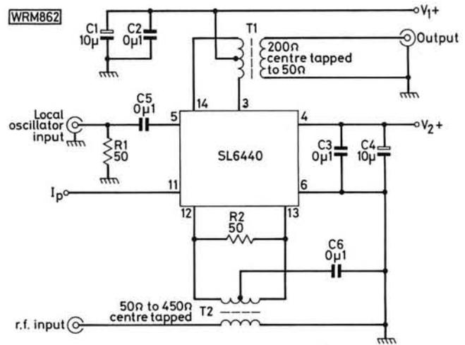
Fig. 4: A high performance balanced circuit
