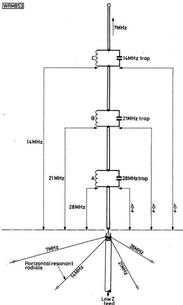
Fig. 8.1: Multi-band trap vertical antenna operating with a resonant radial system
