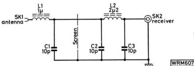
Fig. 1: Circuit diagram
