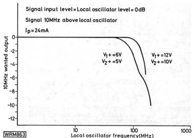
Fig. 5: Frequency performance of the SL6440
