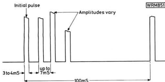
Fig. 2.2: Unmodulated four pulse "Woodpecker" signal which often precedes usual modulated pulse transmissions
