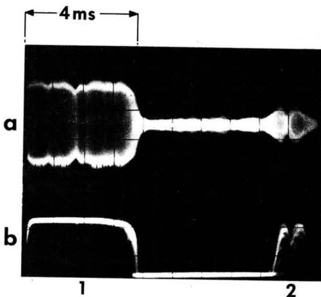
Fig. 2.1: Oscilloscope showing the expanded "Woodpecker" pulse (a) unrectified (b) rectified
