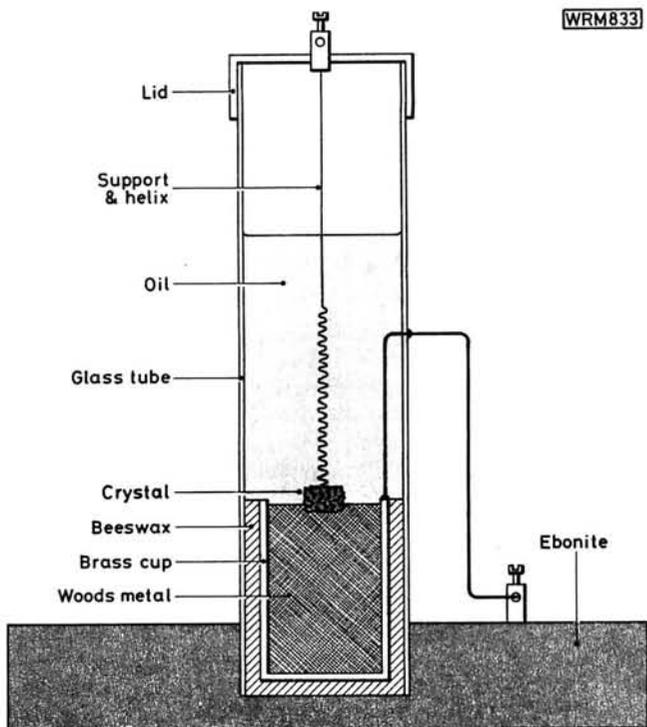
**Fig. 9: An example of an oil-immersed point contact detector**
