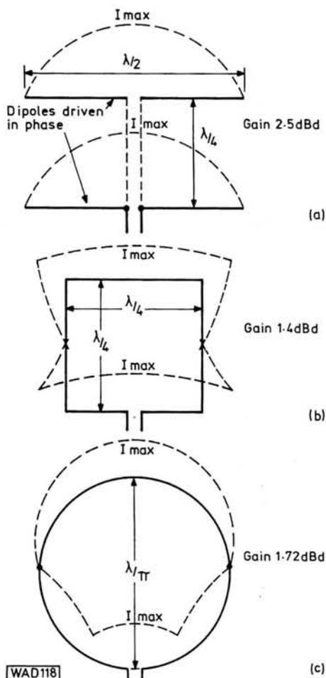
**Fig. 1(a):** Configuration of a two-element array from which the square loop is derived (b) Square loop format showing current distribution; gain factor 1.4dB per single loop over dipole (c) Circular loop with diameter  $\lambda/\pi$  has a more uniform distribution of current; gain factor 1.72dB per single loop over dipole
