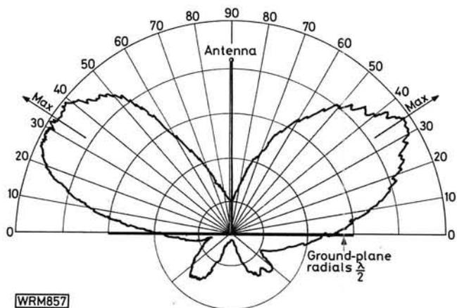
**Fig. 8.5: Typical vertical angle radiation from  $5\lambda/8$  v.h.f. vertical above a ground-plane of four  $\lambda/2$  radials**
