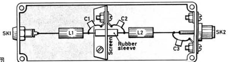
Fig. 2: General layout of the filter
