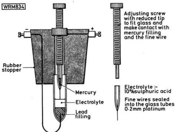
**Fig. 10: One design of an electrolytic detector**
