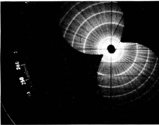
Fig. 5: Radiation pattern of a single loop of diameter  $\lambda$  taken from a 941.9MHz model
