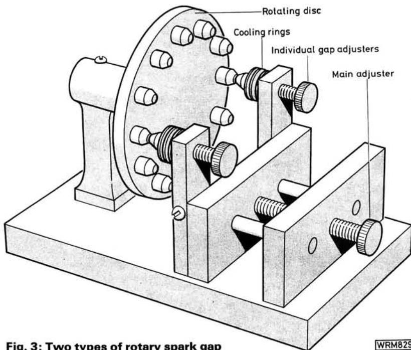
**Fig. 3: Two types of rotary spark gap**
