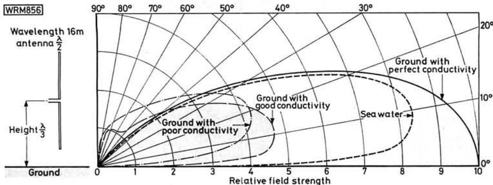
**Fig. 8.4: Vertical angle radiation from vertical  $\lambda/2$  with centre point  $\lambda/3$  above ground showing effects of ground conductivity**
