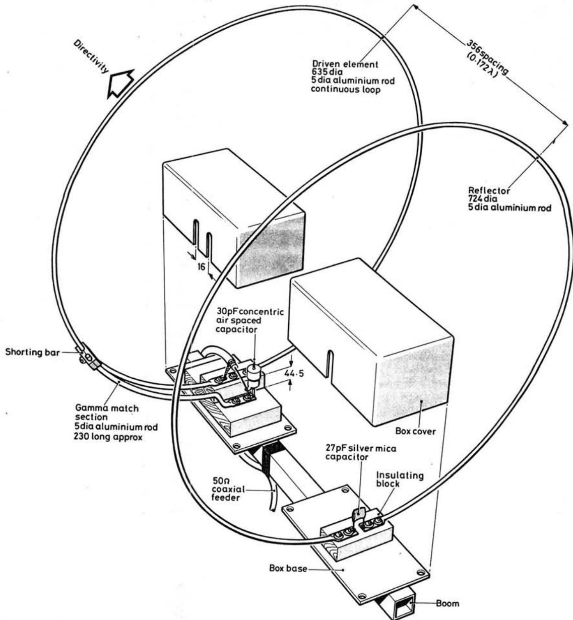
**Fig. 4: Full construction details of the two-element 144MHz ring beam antenna. The boom may be connected to the supporting mast by means of a bracket located between the elements as shown in the photograph on page 26. As drawn, the antenna is horizontally polarised; rotating the boom and element assembly through 90 degrees will provide vertical polarisation**
