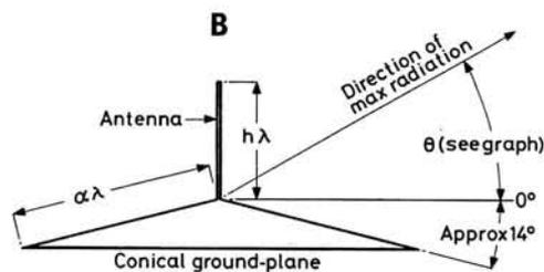
**Fig. 8.6(A): Angle of maximum radiation obtainable using flat disc ground-planes of various radii and (B) angle of maximum radiation using conical ground-planes**
