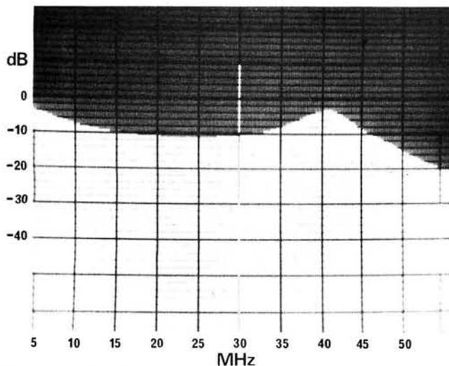
Spectrum analyser plots of the filter. Above  $C1 = C2 = C3 = 10\text{pF}$ . Below  $C1 = C2 = 40\text{pF}$ ,  $C3 = 10\text{pF}$ . By varying  $C1$  and  $C2$  it is possible to alter the characteristics
