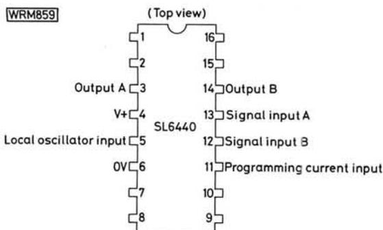
Fig. 1: Connections of the SL6440
