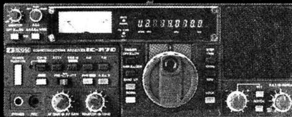
The R-70 covers all modes (when the FM option is included), and uses 2 CPU-driven VFO's for split frequency working, and has 3 IF frequencies: 70MHz, 9MHz and 455KHz, and a dynamic range of 100dB. It has a built-in mains supply.
