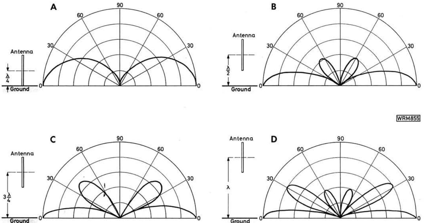
**Fig. 8.3:** Vertical angle radiation patterns for  $\lambda/2$  vertical antennas at heights to centre point of (A)  $\lambda/4$ , (B)  $\lambda/2$ , (C)  $3\lambda/4$ , (D)  $\lambda$ .
