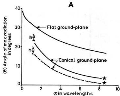
★ Slope angle of cone approx  $14^\circ$
