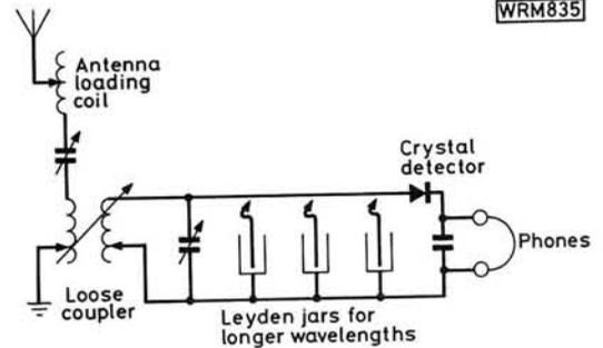
**Fig. 5: The circuit of a typical crystal receiver**
