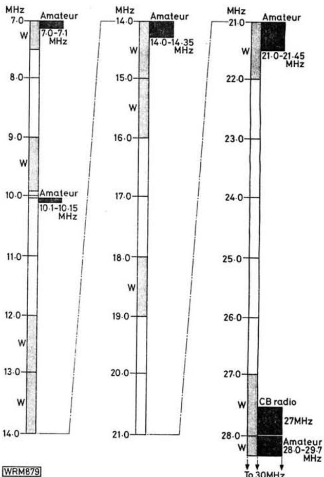
Fig. 2.5: Usage of the frequency band 7-30MHz by the Russian OTHR
