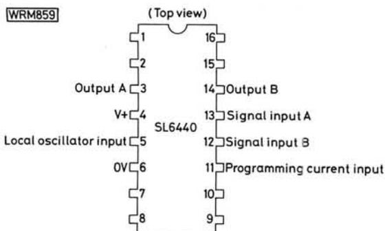
Fig. 1: Connections of the SL6440
