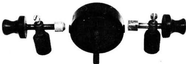
The voltage supply for the spark gap was normally provided by an induction coil with a make and break set of contacts fed from a suitable battery (the same principle as now used for coil ignition in petrol engines). Almost any form of regular switching of the d.c. supply was applied to the induction coil primary.
