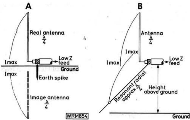
**Fig. 8.2(A):** Current distribution of a  $\lambda/4$  vertical with base at ground level and (B) in conjunction with resonant horizontal radial
