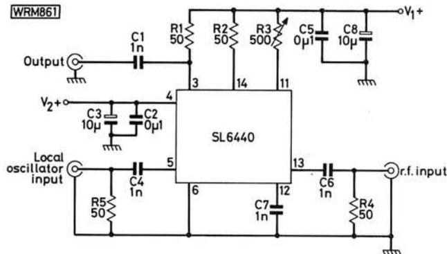
Fig. 3: A simple single-ended mixer circuit
