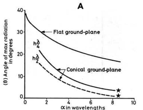
★ Slope angle of cone approx  $14^\circ$
