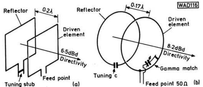
**Fig. 3(a):** Configuration of a two-element quad antenna for optimum gain/smallest amplitude rear and side lobes (b) Configuration of two-element circular loop antenna for optimum gain and no significant rear/side lobe amplitudes
