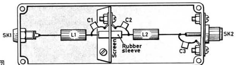
Fig. 2: General layout of the filter
