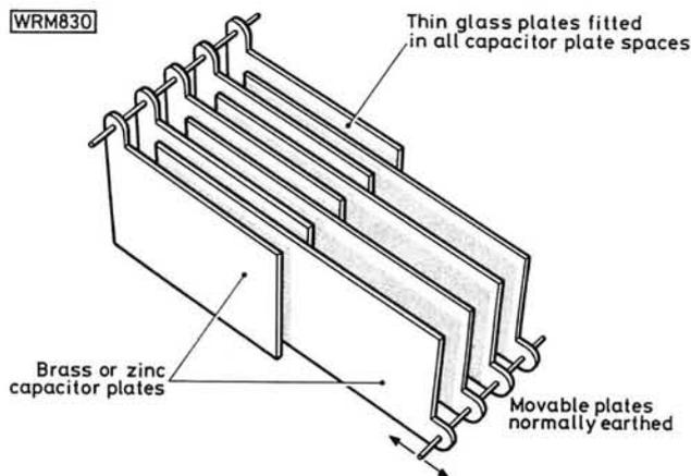
Fig. 2: An early form of adjustable capacitor
