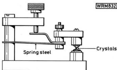
**Fig. 8: A Perikon two-crystal detector**
