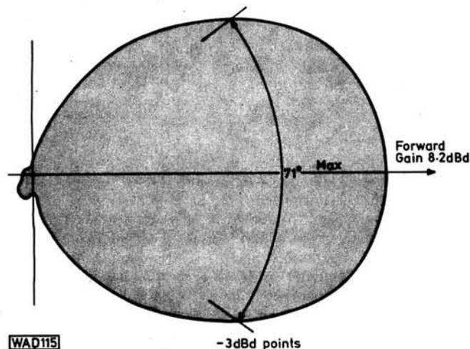
Fig. 6: Horizontal mode radiation pattern of the prototype 144MHz antenna. Measured gain is 8.2dBd
