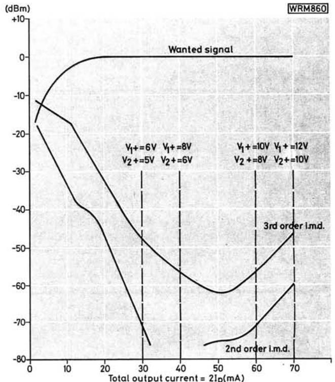
Fig. 2: Variation of 2nd and 3rd order intermodulation levels with the total output current (Signal frequency 30MHz)
