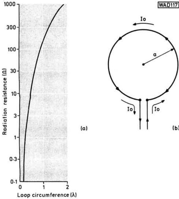
**Fig. 2(a):** The radiation resistance of circular loops up to  $2\lambda$  diameter. The  $R_r$  of a  $\lambda/\pi$  diameter loop is approximately  $150\Omega$  (b) Direction of current (in-phase) around a circular loop  $\lambda/\pi$  diameter. Points of maximum current are designated as  $I_o$
