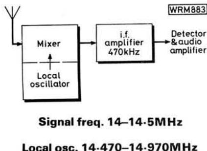
**Fig. 1: Simplest superhet circuit with combined mixer/local oscillator feeding into a fixed frequency amplifier where most of the gain of the receiver takes place**
