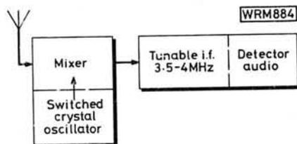
**Fig. 2: Here the mixer is associated with an oscillator having several fixed frequency crystals, one for each band, feeding into an i.f. amplifier which can be tuned over a range of 500kHz, usually one range of a conventional superhet. Hence there is double frequency conversion**
