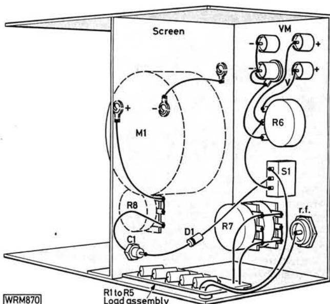
Fig. 4: A cutaway internal view of the prototype. Note the voltage input earthing tag is taken from the phono socket and carefully enlarged to fit the thread of the wander plug socket. The feed-through capacitor is soldered to a washer or piece of tinplate which is then bolted to the dividing screen
