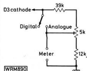
Fig. 4: Details of the digital/analogue metering direct readout facility
