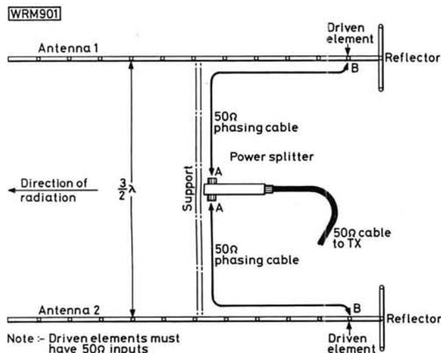
**Fig. 9.3: A pair of beam antennas stacked  $3\lambda/2$  apart phased and fed via a two-way power splitter and phasing lines an equal number of  $\lambda/2$  multiples long**
