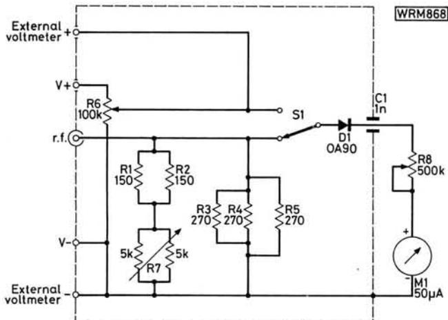
Fig. 3: The circuit diagram of the prototype. Note that C1 is now a feed-through capacitor providing r.f. isolation for M1 as an additional function
