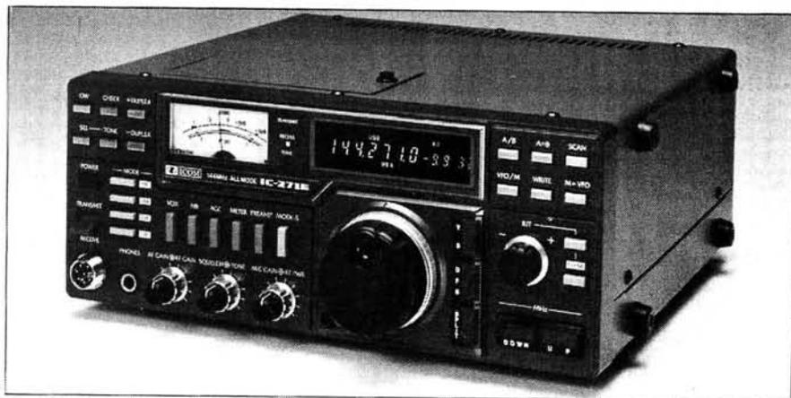
Optional extras include; speech synthesiser announcing displayed frequency; 22 channel memory extension—with scan facilities; 10Hz tuning facility and internal "chopper"
