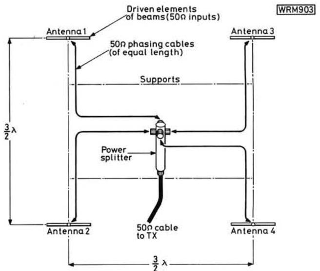
**Fig. 9.4: Four beam antennas stacked and bayed  $3\lambda/2$  apart and fed via a four-way power splitter through phasing lines each an equal number of  $\lambda/2$  multiples long**
