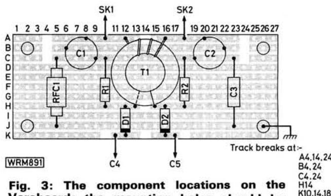
Fig. 3: The component locations on the Veroboard; the mounting holes should be drilled very carefully to avoid damaging the board
