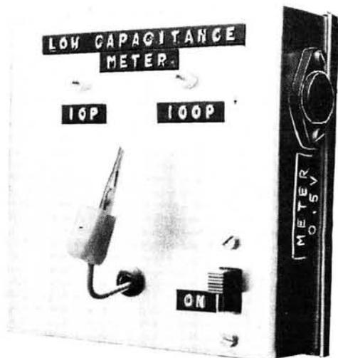
The ratio of capacitance between the maximum test capacitance (10pF or 100pF) to that of C1 or C2 has been made high in order to ensure that the signal voltage across the lower capacitor varies in a substantially linear fashion. This ratio will be seen to be about 10:1.
