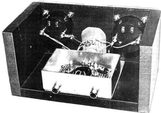
line it will show the s.w.r. presented by the antenna system to the bridge without any immediate adjustment being possible. By checking the s.w.r. at different frequencies across a band it will, however, show the effective bandwidth of the system and indicate whether alterations to the dimensions of the antenna are necessary to bring it to resonance at a higher or lower frequency.
