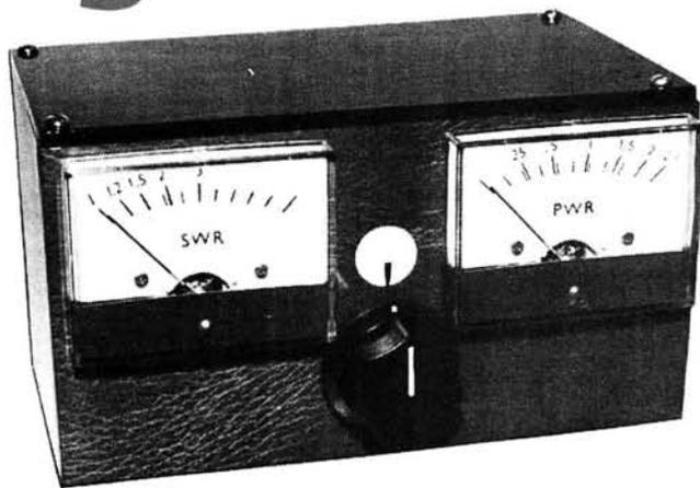
reflected readings are obtained simultaneously on the two meters M1 and M2, and the bridge is matched and balanced at the required load impedance by C1 and C2. Brief details are given in Fig. 5 of an alternative, less expensive, single meter version.
