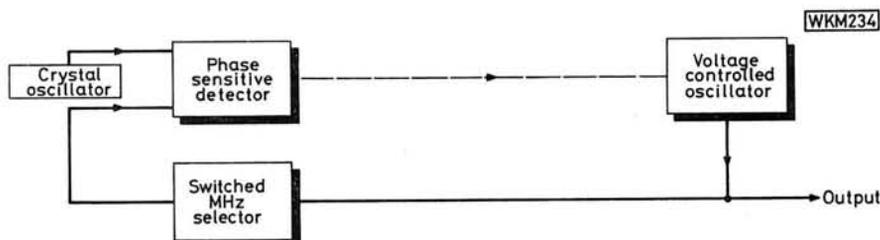
Fig. 3: Here the p.l.l. circuit includes a circuit that provides integral harmonics of the basic 1MHz crystal frequency right through the required receiver tuning range, selected by a simple switch
