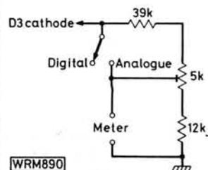
Fig. 4: Details of the digital/analog metering direct readout facility
