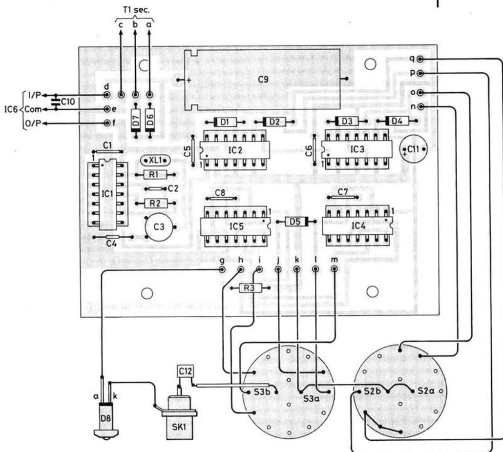
Although no fuse was fitted into the prototype chassis it is suggested that one be fitted where indicated. A 1 amp rating should prove suitable. The actual transformer connections will depend on the make used, the connections shown are for the RS 207-633. This transformer has the secondary connections along the bottom nearest to the chassis—mains connections are on the top and easy to touch, so be careful when working on the unit with the cover removed. The transformer is held in place by two
