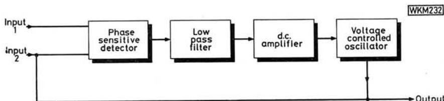
Fig. 1: The four basic stages required to form a voltage controlled oscillator or phase-locked loop circuit (p.l.l.)
