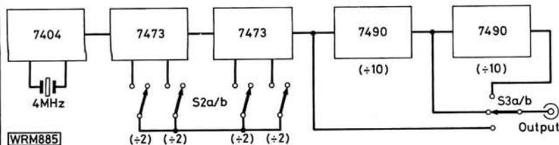
Fig. 1: Schematic block diagram of the Digital Calibrator outlining the division process used to obtain the final marker spacings, harmonics of which are usable well into the u.h.f. regions
