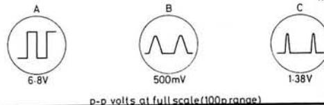
acts like a Class C amplifier in that only parts of the negative half-cycles at pin 2 are amplified, these giving a positive-going output at pin 6. A combination of a.c. and d.c. feedback ensures a linear input/output voltage relationship. The MOSFET op. amp. was chosen in preference to the usual 741 as it will continue to operate on these negative half-cycles, when its input voltage falls below earth potential. This avoids the complication of double or split supplies.
