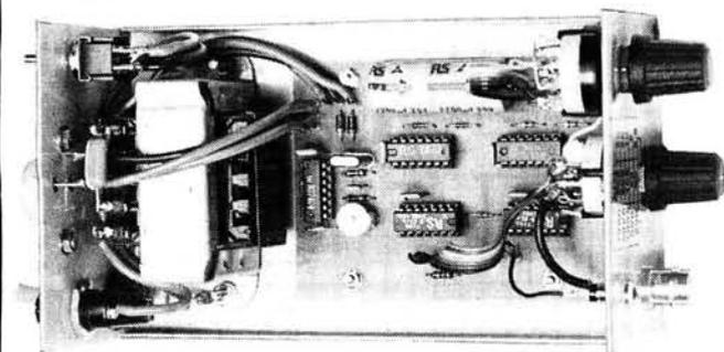
As we know the actual frequency coming from the calibrator on its fundamental frequency, at each setting of the switches, we must know how long each square wave pulse takes and this can be used to give precise timing pulses for calibrating (oscilloscope time bases etc.) test equipment.
