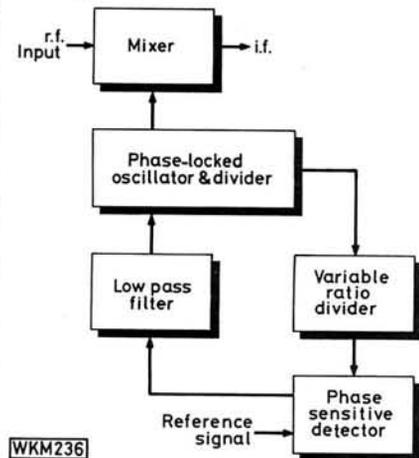
**Fig. 5: The type of circuit used in many modern receivers using full frequency synthesis with the tuning at 10 or 100Hz intervals, suitable for frequencies into the u.h.f. range**
