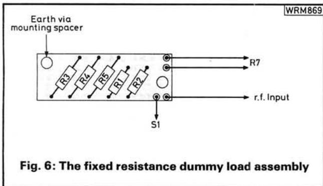
Fig. 6: The fixed resistance dummy load assembly
