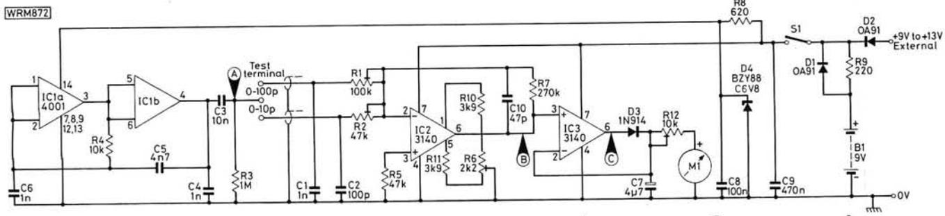
**Fig. 2: The complete circuit diagram of the sensitive capacitance meter. The waveforms shown adjacent are peak-peak volts at full scale (100pF range)**
