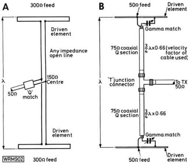
**Fig. 9.2: (A) Two stacked folded dipoles fed in-phase via an open line (see text). (B) Two gamma matched dipoles with 50Ω feed impedance, phased by a pair of 75Ω "Q" sections of coaxial cable**
