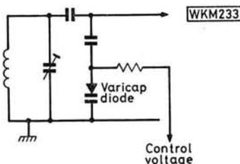
Fig. 2: The d.c. control voltage is applied to a varicap diode which acts as a variable capacitor across the tuned circuit, its value depending upon the applied voltage
