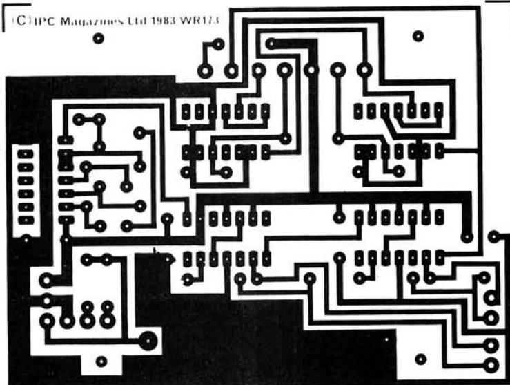
Fig. 3: Component placement/interconnection details and full size p.c.b. track pattern
