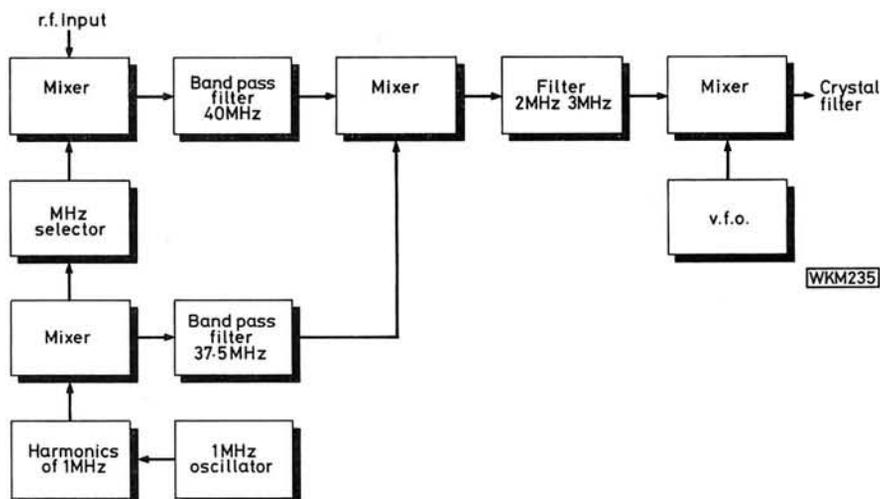
Fig. 4: Simplified diagram of the Wadley Loop system which was used by Racal in some of its famous communications receivers
