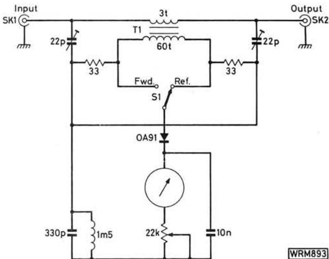
**Fig. 5: A single meter version of the s.w.r. bridge**
