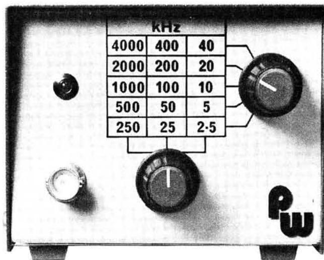
The Digital Calibrator front panel showing marker spacings
