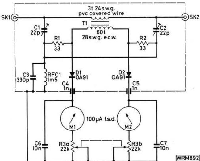
Fig. 2: The circuit diagram of the QRP s.w.r. bridge
