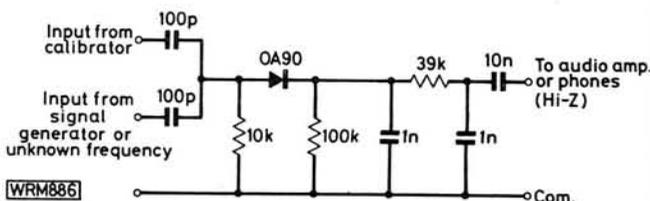
**Fig. 4: Diode detector circuit suitable for beating the output from a signal generator with the Calibrator output. The generator should be tuned for zero beat at each calibration point required**
