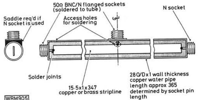
Fig. 9.6: A "practical" 50 $\Omega$  low loss 432MHz antenna combiner as built by G8MCP/G8MCQ and successfully used for e.m.e. work
