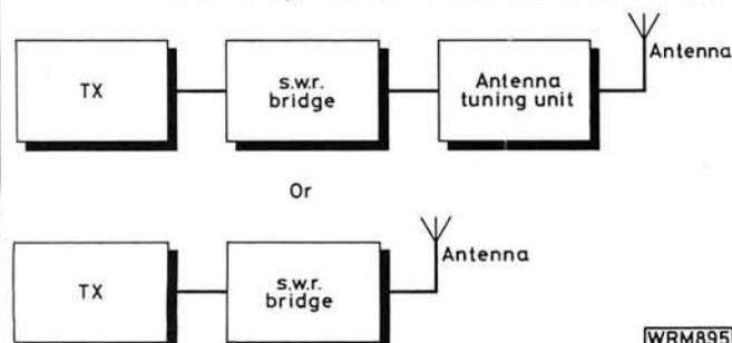
Fig. 1: Where to place the s.w.r. bridge—the length of feeder between the TX and the bridge should be as short as possible
