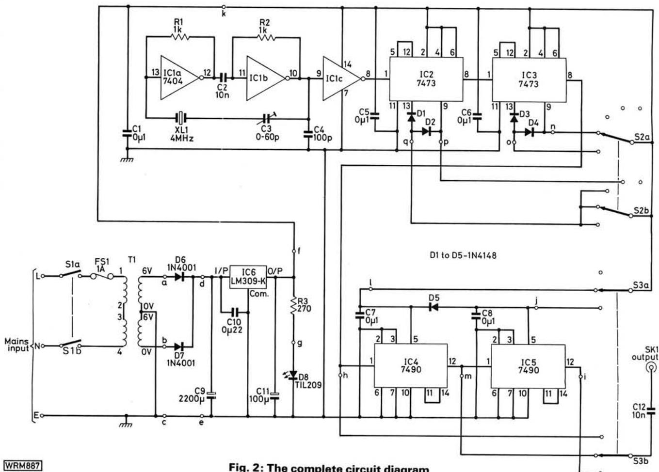
Fig. 2: The complete circuit diagram
