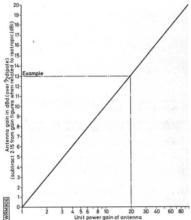
The graph covers up to 20dBd and to determine e.r.p. it is only necessary to multiply the power fed to the antenna by the unit power gain. The dotted line example shows the power gain related to 13dBd as almost 20 (actual figure 19.95) so with 25 watts applied to the antenna terminals, the e.r.p. would be  $19.95 \times 25 = 498.75$  watts.
