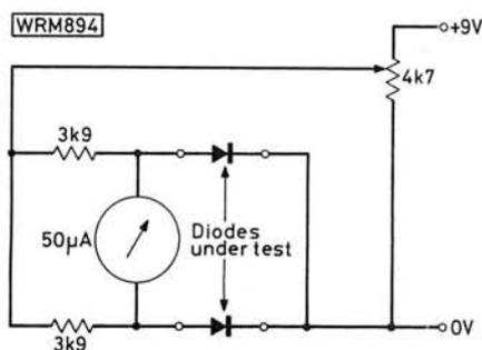
**Fig. 4: A simple diode matching circuit. The two resistors should be matched with an ohmmeter. As the voltage is increased by rotating the potentiometer the meter should not deflect more than 1µA from its no-current setting. It may be necessary to test several diodes before a matched pair is obtained**
