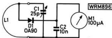
Fig. 1 (above): Shows the circuit diagram of the Simple 144MHz Wavemeter. The layout below shows the general arrangement of components built into the plastics enclosure. For reliable operation it is essential that the relative positions of L1, D1 and C1 are maintained
