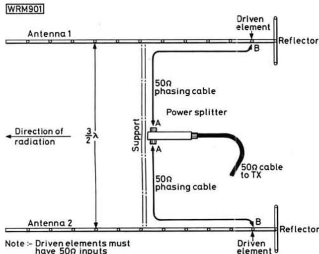
**Fig. 9.3: A pair of beam antennas stacked  $3\lambda/2$  apart phased and fed via a two-way power splitter and phasing lines an equal number of  $\lambda/2$  multiples long**
