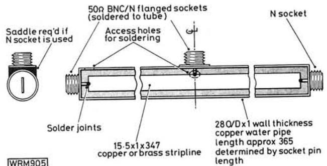
Fig. 9.6: A "practical" 50Ω low loss 432MHz antenna combiner as built by G8MCP/G8MCQ and successfully used for e.m.e. work
