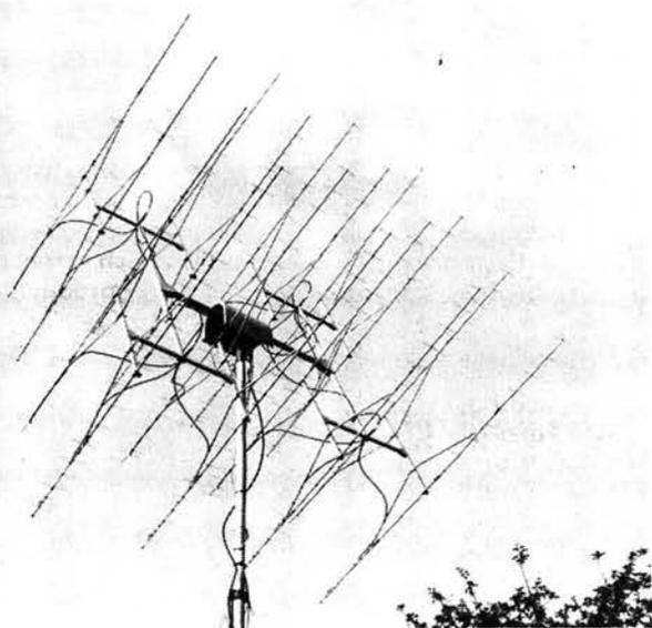
**A very impressive array of stacked and bayed antennas! This system, which is fully steerable for 432MHz e.m.e. operations, consists of sixteen 21-element Tonna Yagis**
