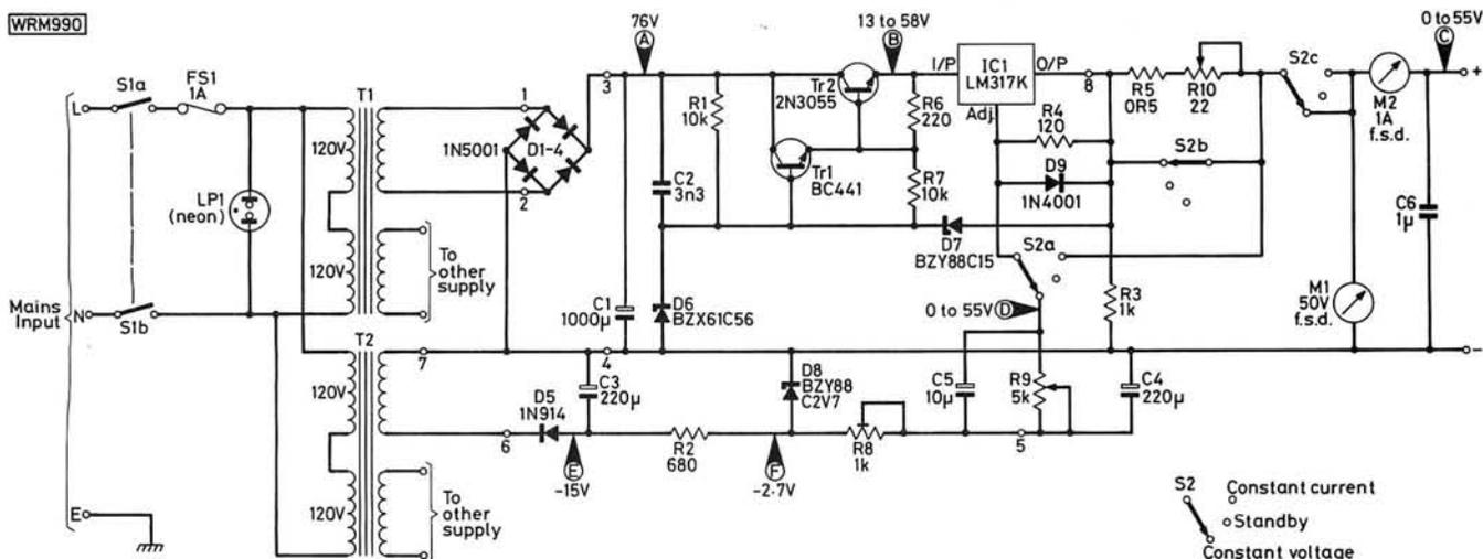
Fig. 1.3: Complete circuit diagram of the PW Bridport dual regulated power supply. Note that only one supply is shown, the other being identical with the component references indicated by the addition of 100 (e.g. R104 etc)
