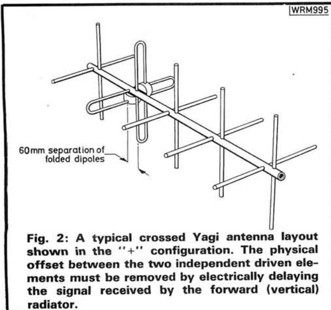
**Fig. 2: A typical crossed Yagi antenna layout shown in the "+" configuration. The physical offset between the two independent driven elements must be removed by electrically delaying the signal received by the forward (vertical) radiator.**
