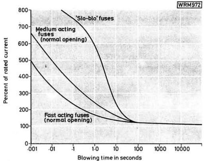
Fig. 1.1: Chart showing the relation of percent of rated current to blowing time
