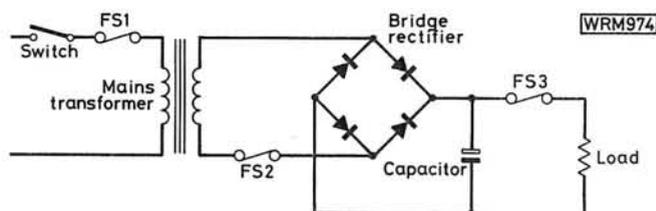
Fig. 1.3: A typical power supply circuit
