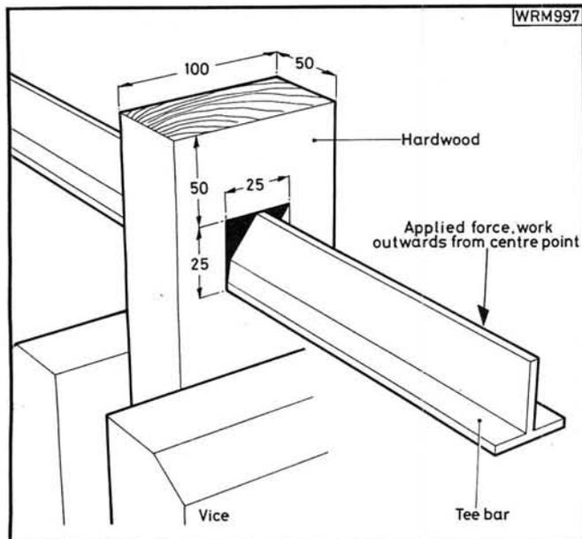
**Fig. 5: The method used by the author to form the parabolic ribs. With care and patience this technique will yield a smooth curve free of kinks**
