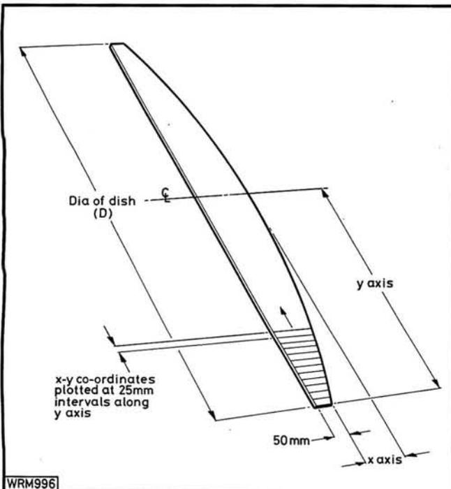
Fig. 2: The profile template arrangement. Melamine faced 12mm Chipboard is ideal for this job, being easy to mark and cut to shape
