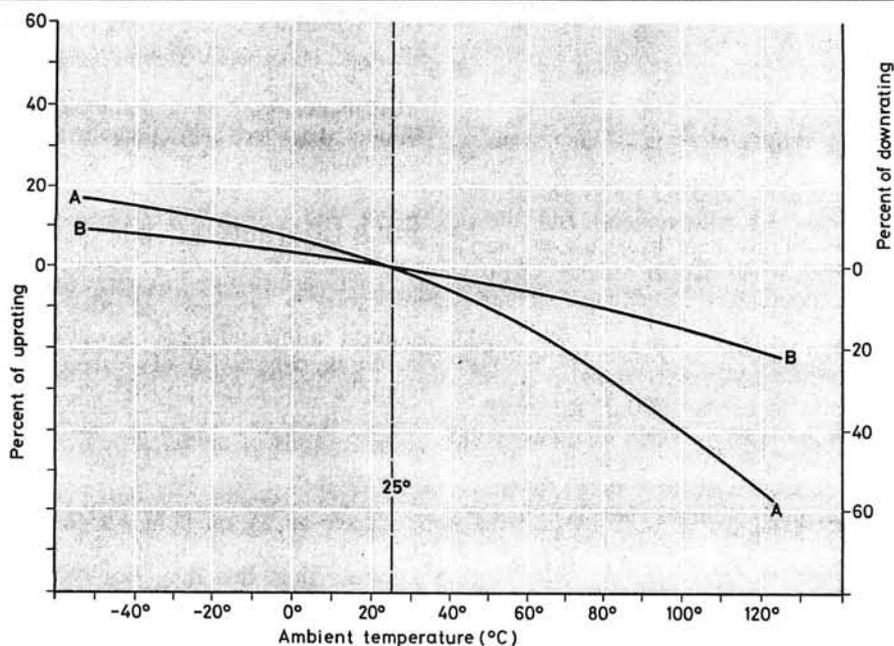
Fig. 1.2: Chart showing effect of ambient temperature on current carrying capacity
