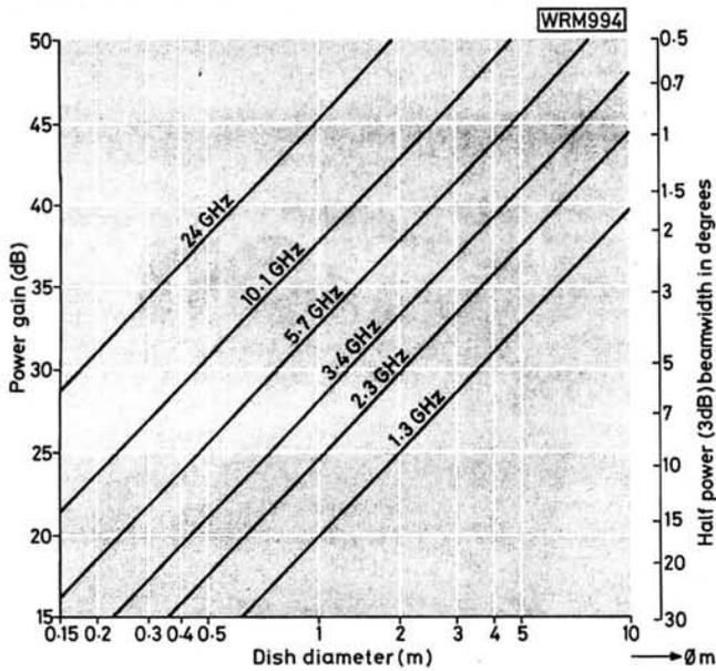
Fig. 1: Graph relating the available gain from a parabolic dish to amateur bands, based on an efficiency of approximately 50 per cent
