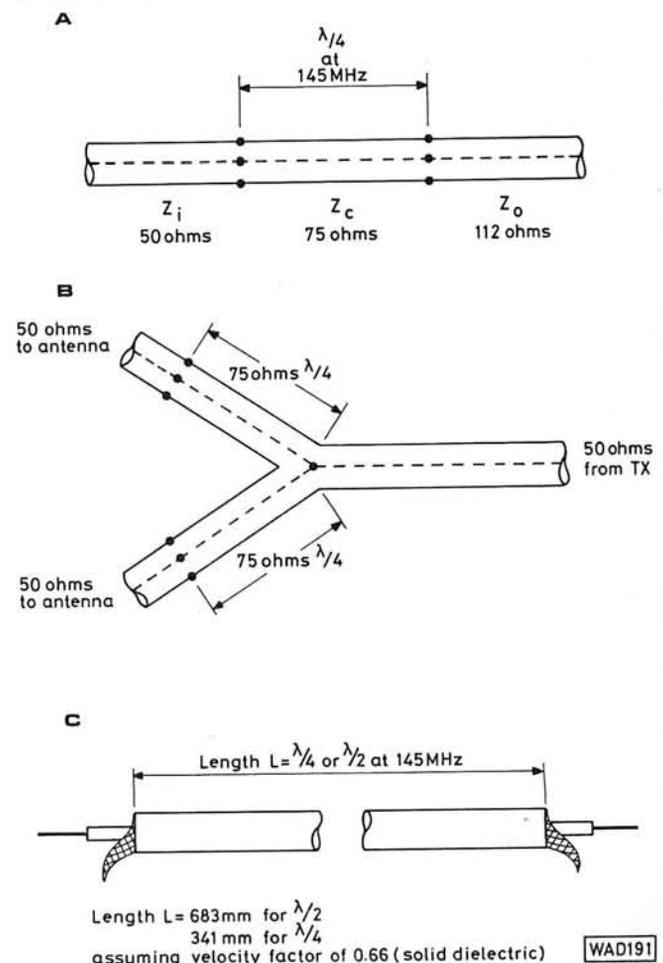
**Fig. 3: Details of the impedance transformer and matching arrangement used in the control box, together with cutting details**
