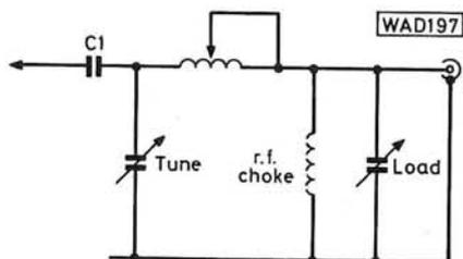
**Fig. 2: Simplified output stage of a transceiver with r.f. choke added to offset blocking effect of capacitor C1 and give d.c. path to earth**
