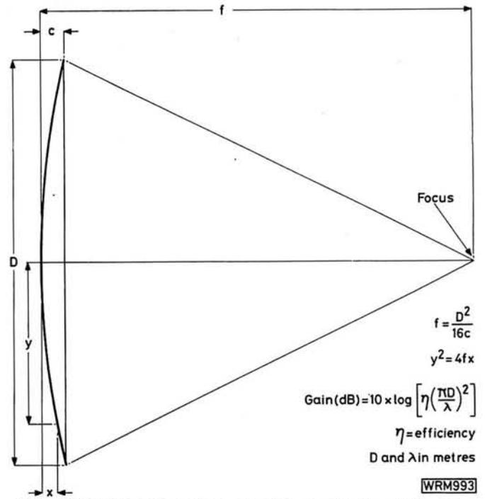
Fig. 3: Basic geometry of the parabolic dish. The formulae shown are used to determine the required parameters
