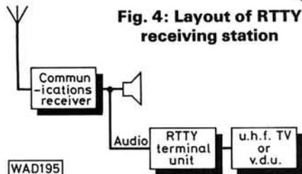
Fig. 4: Layout of RTTY receiving station
