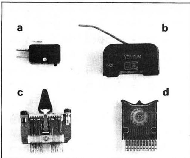
**Fig. 11: (a) Button-actuator miniature microswitch. (b) Lever-actuator, heavy-duty microswitch. (c) Lever switch. (d) Thumbwheel edge switch**
