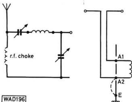
**Fig. 1: Circuit of a typical a.t.u. with an r.f. choke added to give a d.c. path to earth for static charges. Right, a dipole connected to receiver input terminals may not have a d.c. path to earth so it is important that one side of the feeder is connected to earth as shown. If coaxial feeder is used this would be the outer shield or braid**
