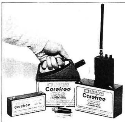
feature of these batteries is the use of calcium as the hardening agent in the lead-acid grid, rather than antimony which has the effect of eventually "poisoning" the battery by depositing itself onto the active material of the negative plate.
