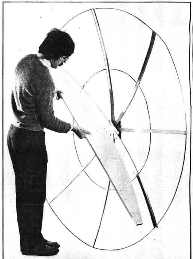
The 2m parabolic dish being checked for profile accuracy before final mesh cladding
