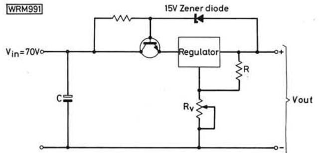
Fig. 1.2: The basic regulator circuit used in the PW Bridport
