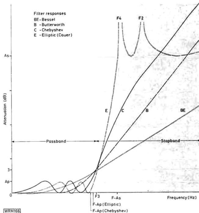
Fig. 1.1: Modern filter responses for typical 5-branch lowpass designs
