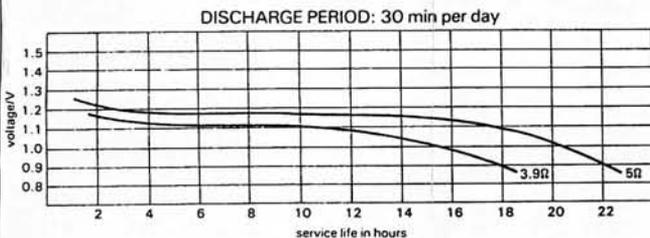
The voltage shown is plotted from the on-load voltage obtained at the end of each day's discharge (HP2 battery)
