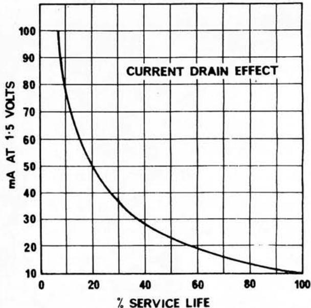
The current drain effect for an SP2 battery
