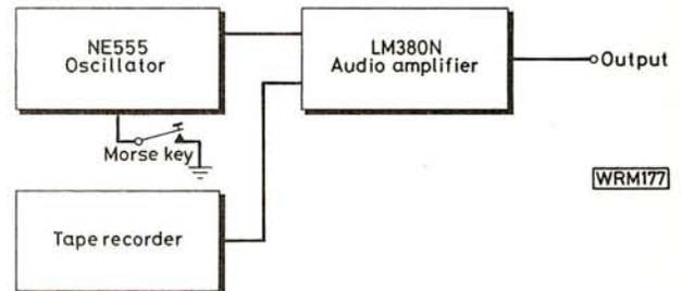
Fig. 1: Schematic block diagram of the training aid. The aim is to key the oscillator in time with the pre-recorded input to develop correct style by direct comparison
