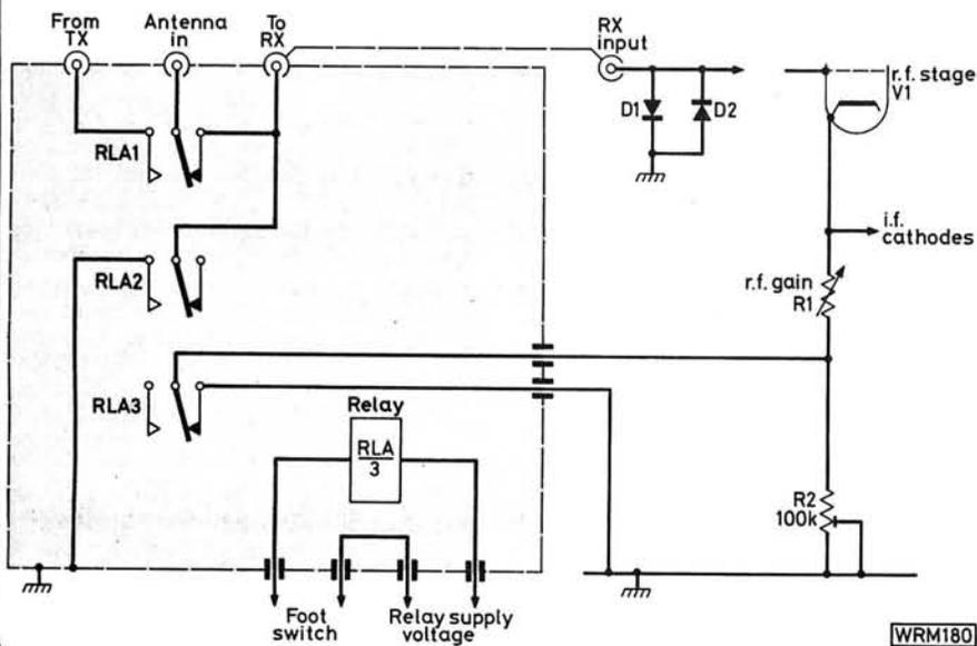
Fig. 1: Composite drawing showing the receive/transmit switching for separate transmitter and receiver. The cross-connected diodes D1, D2 should be connected by the shortest possible leads right across the receiver's antenna terminals or socket, preferably inside the set. The mod to the RF gain control is easily adapted for solid-state receivers. Note the relay contacts RLA2 which put a short circuit across the receiver's input circuit as additional protection
