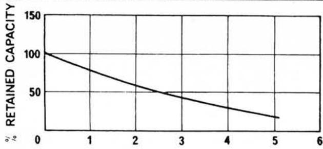
Charge retention with time for nickel-cadmium cells
