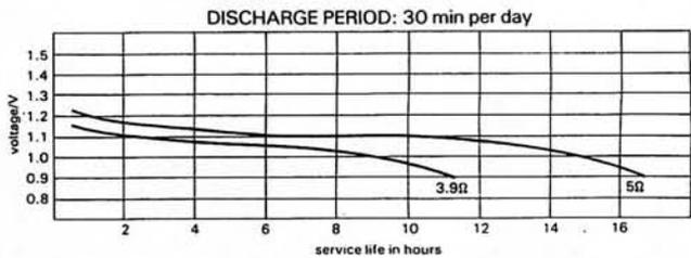
The voltage shown is plotted from the on-load voltage obtained at the end of each day's discharge (SP2 battery)
