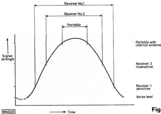
Fig. 1: Fading cycle
