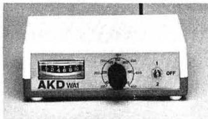
120-450MHz, providing a meter readout of relative signal strength. The unit is fully portable, using a 6-F22 (PP3) 9 volt battery supply and is supplied complete with external antenna. Being a sensitive device it can also be used as a field strength meter for comparative measurements over its frequency range.
