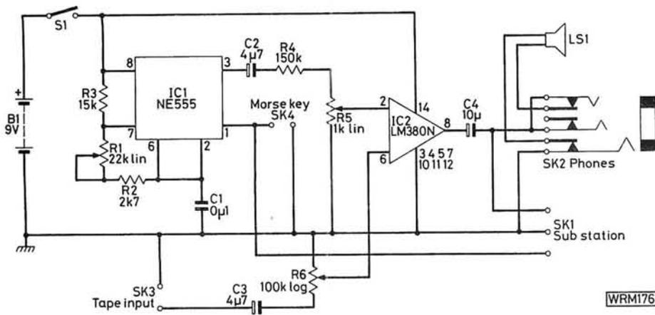
Fig. 2: Circuit diagram of the trainer together with details of the optional external sub-station. Pins 4 and 5 of IC1 are not terminated
