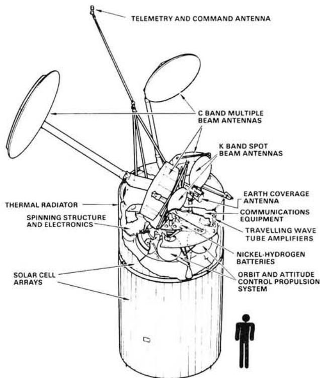
Fig. 2.1: INTELSAT VI spacecraft configuration
