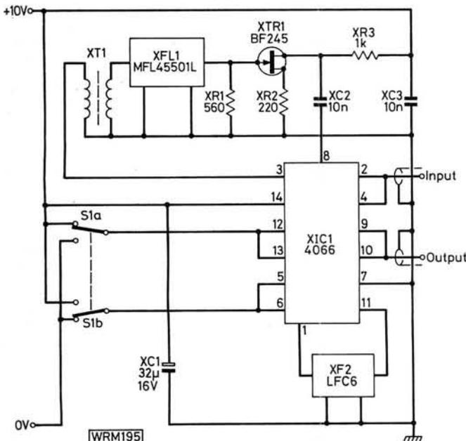
**Fig. 2.1: The circuit diagram of the new switching board**
