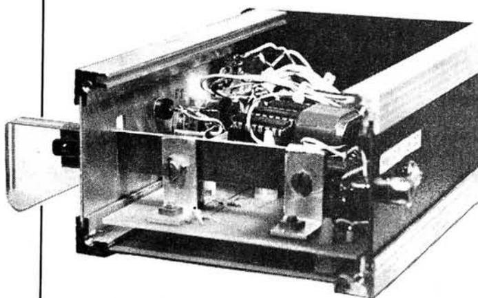
An end view of the prototype keyer showing the bug key. The movable wiper is formed from a 100 × 12mm piece of 1.5mm double-sided p.c.b.
