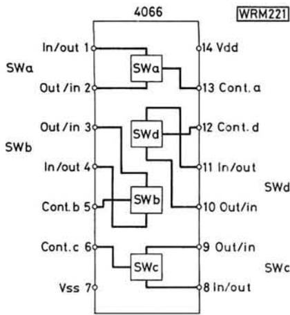
**The internal circuit of the 4066 c.m.o.s. quad switch**
