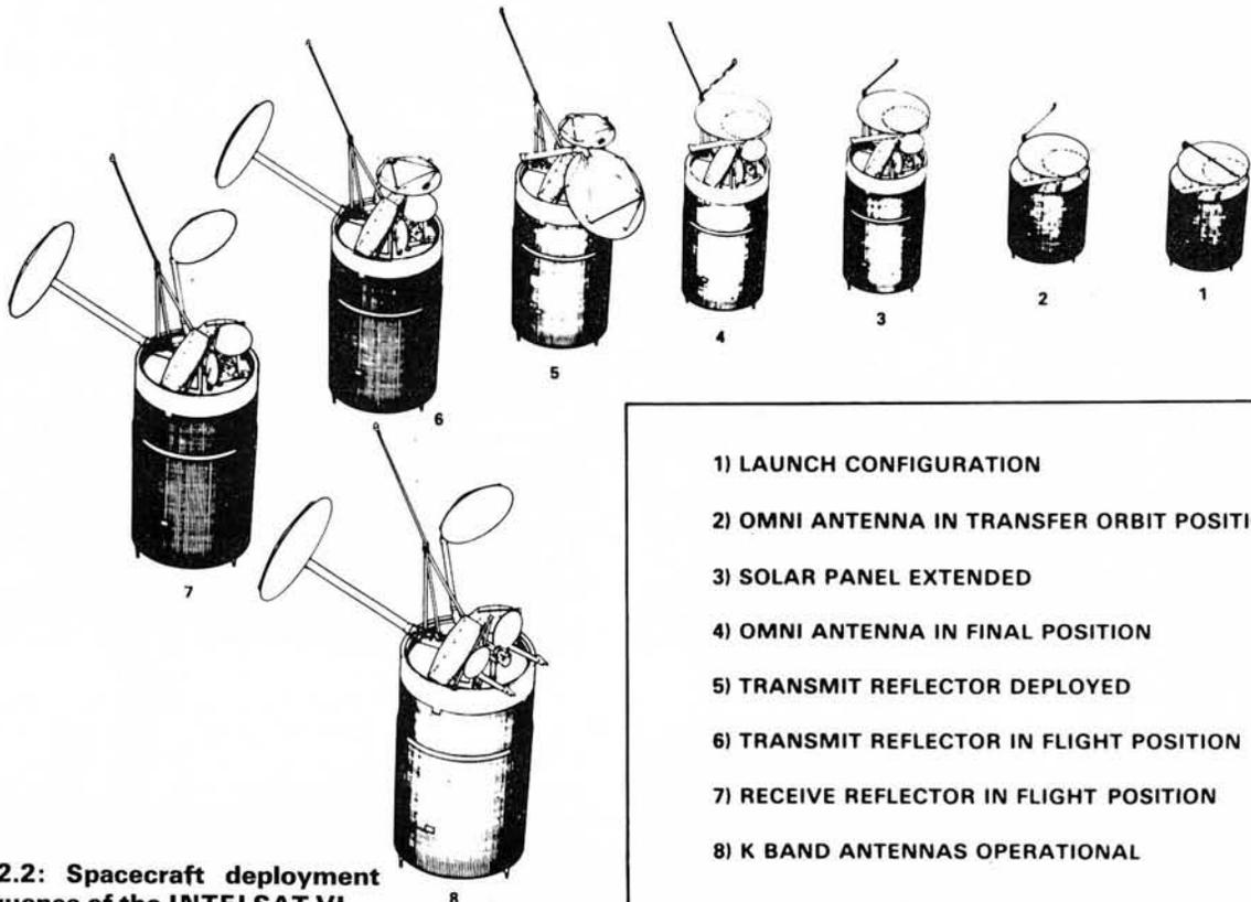
**Fig. 2.2: Spacecraft deployment sequence of the INTELSAT VI**
