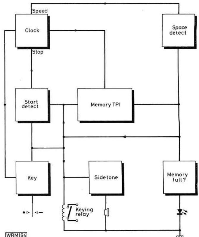
Fig. 1: Block diagram of the Memory Keyer
